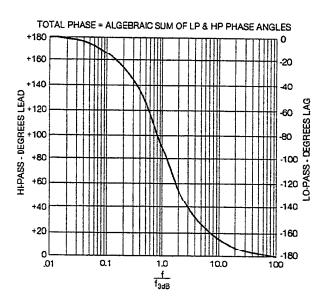
Figure 1-5. 12 dB FILTER PHASE vs NORMALIZED FREQ. RESPONSE
