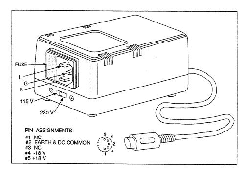
Figure B-1. EXTERNAL POWER SUPPLY
