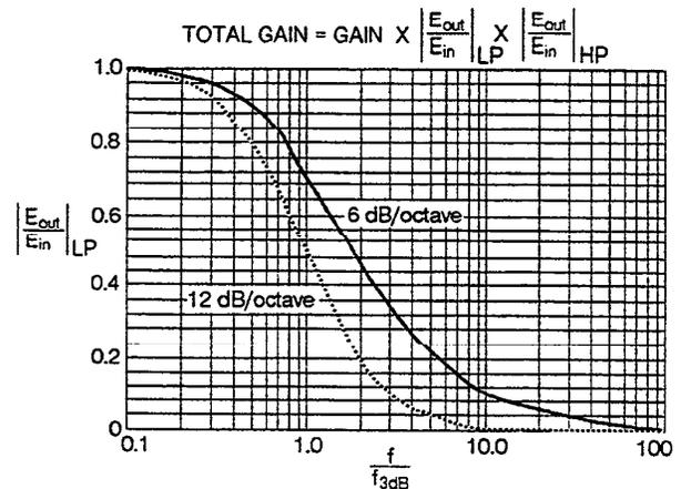
Figure 1-2. LOW-PASS FILTER AMPLITUDE vs NORMALIZED FREQ. RESPONSE
