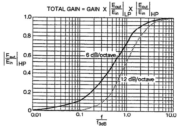
Figure 1-3. HI-PASS FILTER AMPLITUDE vs NORMALIZED FREQ. RESPONSE
