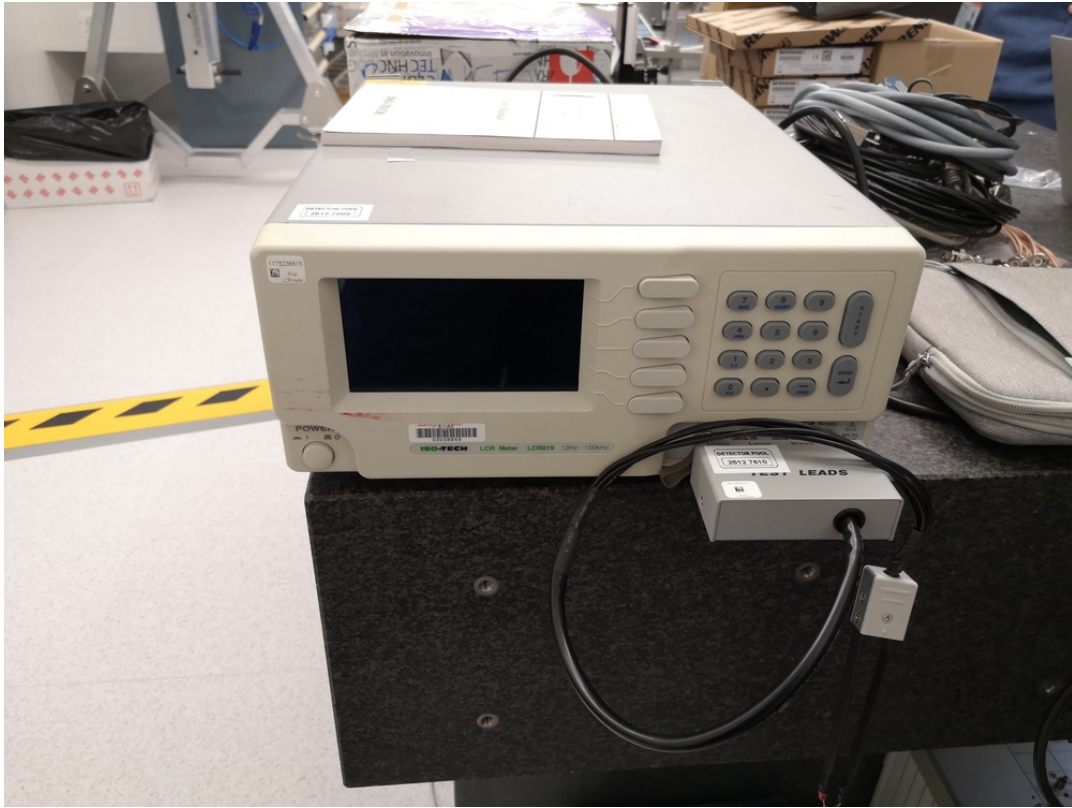
Figure 2.3: LCR Meter used for the measurements
