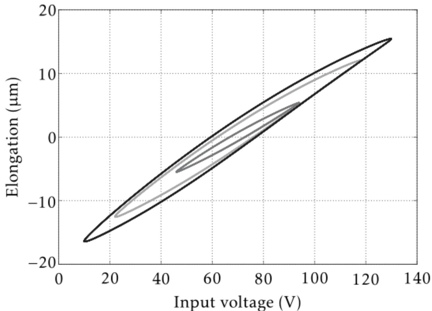
**Figure 6.16:** Measured hysteresis loops for a single PE actuator, 70 V bias + 1 Hz sine wave: 60 V amplitude (black), 48 V amplitude (light grey), 24 V amplitude (dark grey)
