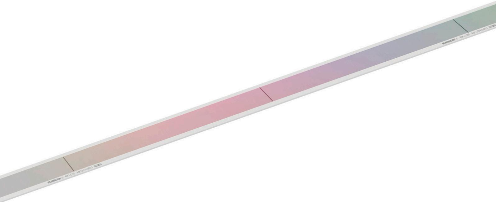
**RKLC is a robust, 6 mm wide stainless steel encoder tape scale with a thickness of 0.15 mm. This allows the scale, when rigidly fixed to a machine axis, to become ‘mastered’ to the machine substrate, matching its thermal expansion coefficient and behaviour. Differential movement between the scale and the machine is thus minimised, improving the metrological performance that can be achieved with simple thermal system compensation.**
