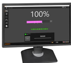
The VIONiC encoder system is compatible with the Advanced Diagnostic Tool ADTi-100 and ADT View software. They provide comprehensive real-time encoder data feedback to aid more challenging installations and diagnostics. The intuitive software interface can be used for:
