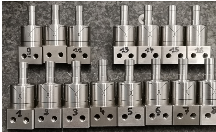
(a) 15 of the 16 received flexible joints
