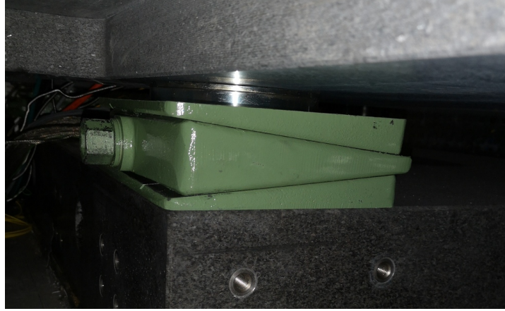
Figure 2.74: AirLoc used for the granite (2120-KSKC).
