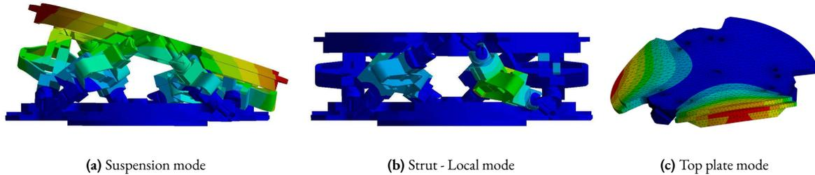
**Figure 3.97:** Measurement of strut flexible modes. First six modes are “suspension” modes in which the top plate behaves as a rigid body (a). Then modes of the struts have natural frequencies from 205 Hz to 420 Hz (b). Finally, the first flexible mode of the top plate is at 650 Hz (c)
