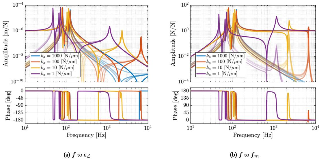
**Figure 3.38:** Effect of axial stiffness of the flexible joints on the plant dynamics. Both from actuator force  $f$  to strut motion measured by external metrology  $\epsilon_{\mathcal{L}}$  (a) and to the force sensors  $f_m$  (b)
