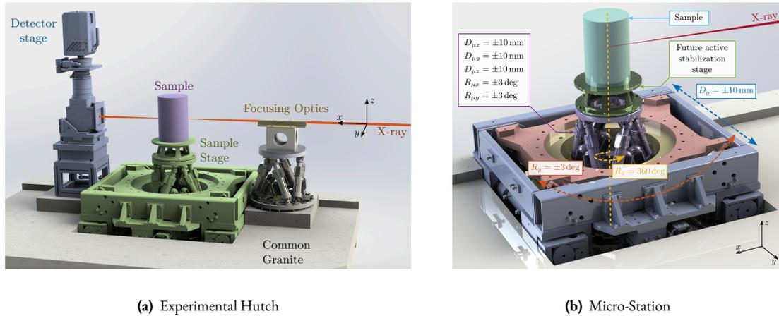
**Figure 1.5:** CAD view of the ID31 Experimental Hutch (a). There are typically four main elements: the focusing optics in yellow, the sample stage in green, the sample itself in purple and the detector in blue. All these elements are fixed to the same granite. CAD view of the micro-station with associated degrees of freedom (b).
