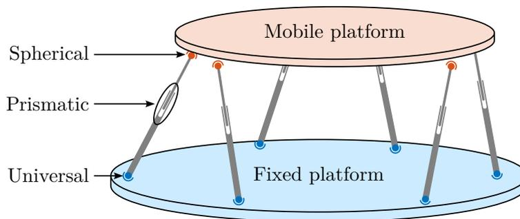
**Figure 2.104:** Schematical representation of the Stewart platform architecture.
