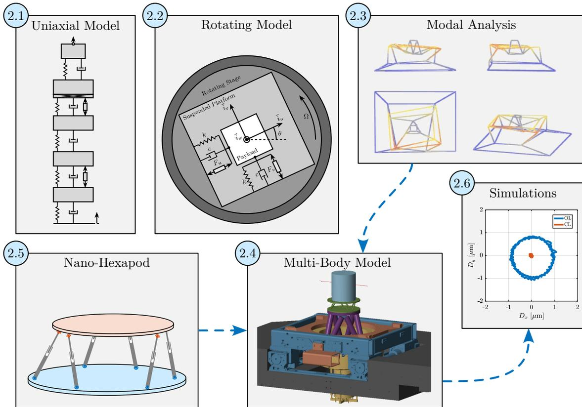
**Figure 2.1:** Overview of the conceptual design development. The approach evolves from simplified analytical models to a multi-body model tuned from experimental modal analysis. It is concluded by closed-loop simulations of tomography experiments, validating the conceptual design.
