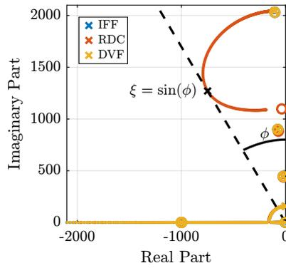
**Figure 2.18:** Root Locus for the three damping techniques applied with the soft nano-hexapod. It is shown that the RDC active damping technique has some authority on one mode of the micro-station. This mode corresponds to the suspension mode of the micro-hexapod.
