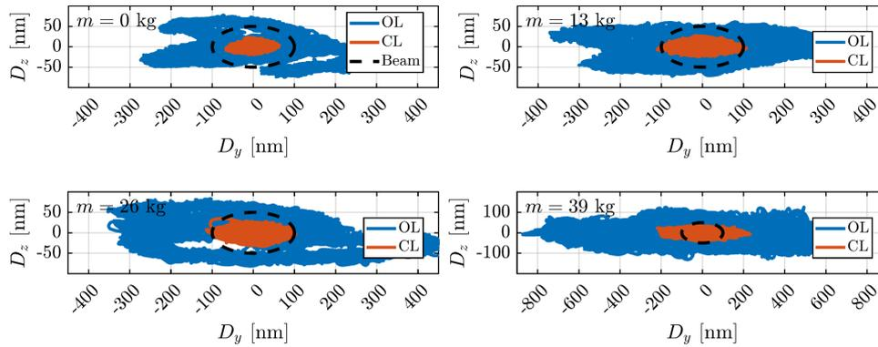
**Figure 4.104:** Measured errors in the  $Y - Z$  plane during tomography experiments at 6 deg/s for all considered payloads. In the open-loop case, the effect of eccentricity is removed from the data.
