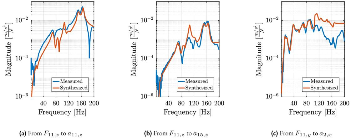
**Figure 2.75:** Comparison of the measured FRF with the FRF synthesized from the modal model.
