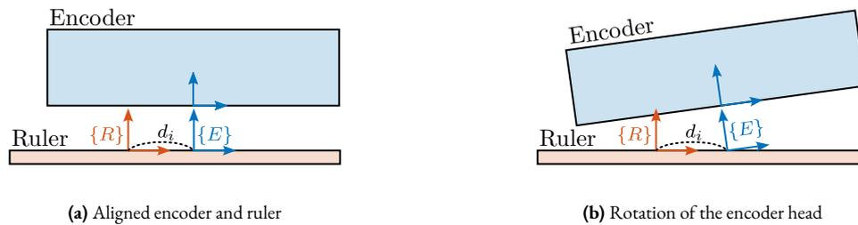
**Figure 3.101:** Representation of the encoder model in the multi-body model. Measurement  $d_i$  corresponds to the  $x$  position of the encoder frame  $\{E\}$  expressed in the ruler frame  $\{R\}$  (a). A rotation of the encoder therefore induces a measured displacement (b).
