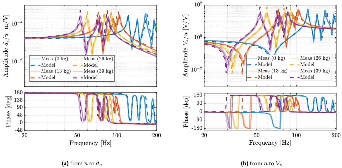
**Figure 4.75:** Comparison of the diagonal elements (i.e. “direct” terms) of the measured FRF matrix and the dynamics identified from the multi-body model. Both for the dynamics from  $u$  to  $d_e$  (a) and from  $u$  to  $V_s$  (b)
