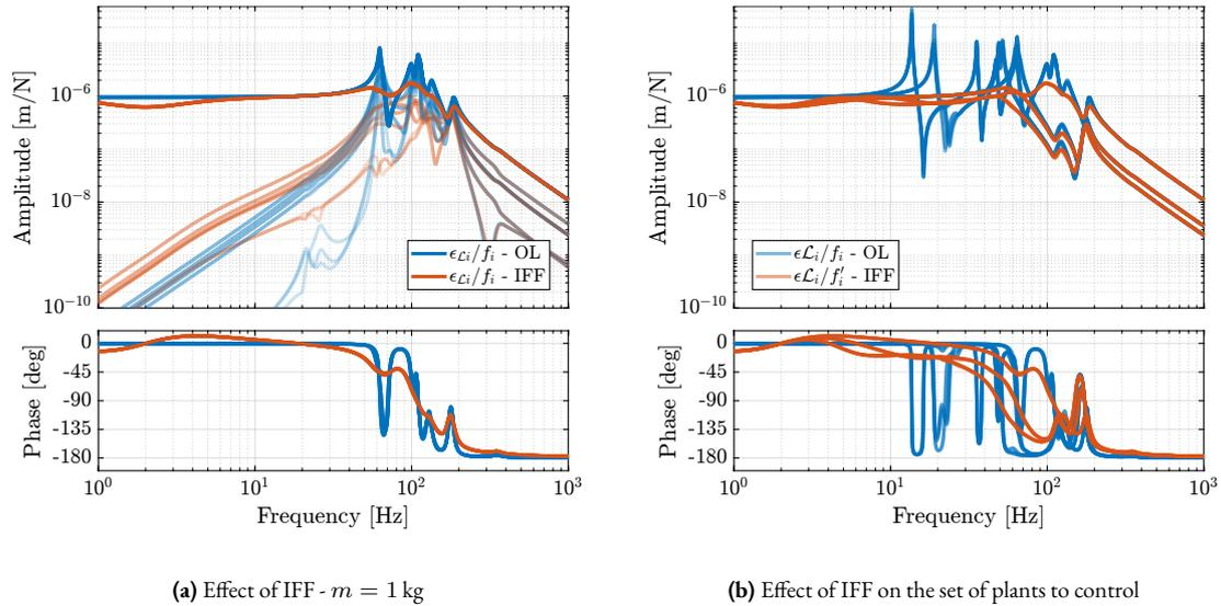
**Figure 2.130:** Effect of Decentralized Integral Force Feedback on the positioning plant for a 1 kg sample mass (a). The direct terms of the positioning plants for all considered payloads are shown in (b).
