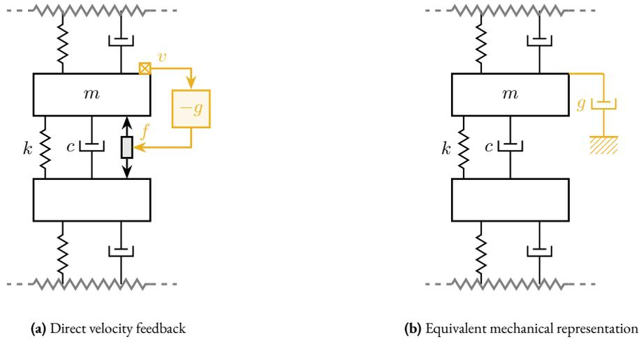
**Figure 2.15:** Direct velocity Feedback (a) is equivalent to a “sky hook damper” (b)
