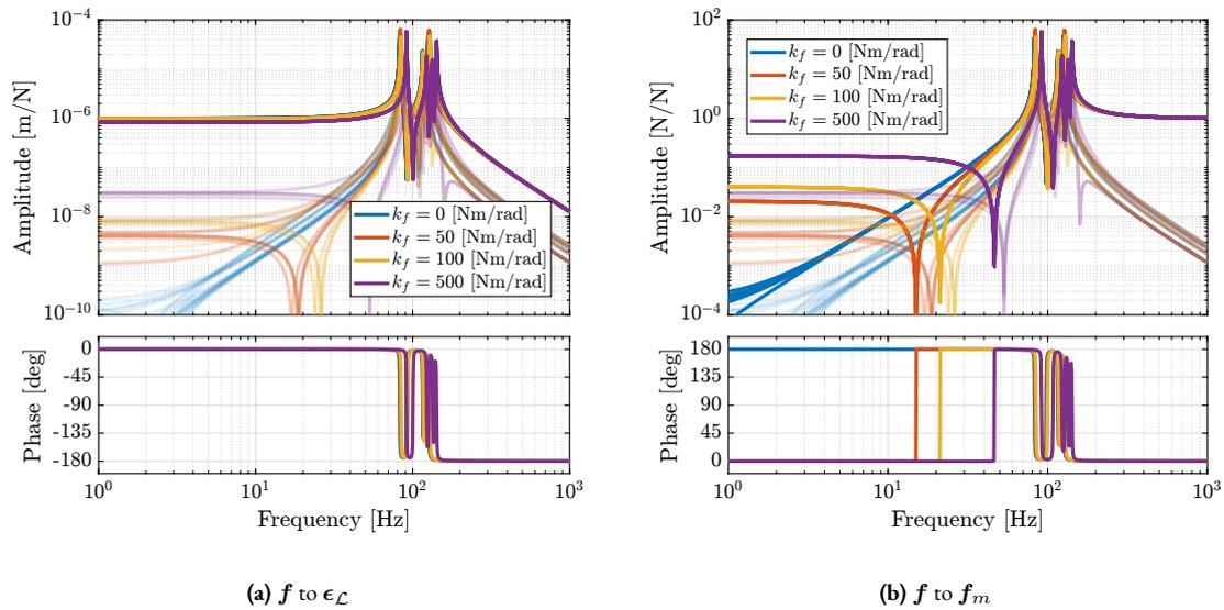
**Figure 3.36:** Effect of bending stiffness of the flexible joints on the plant dynamics. Both from actuator force  $f$  to strut motion measured by external metrology  $\epsilon_{\mathcal{L}}$  (a) and to the force sensors  $f_m$  (b)
