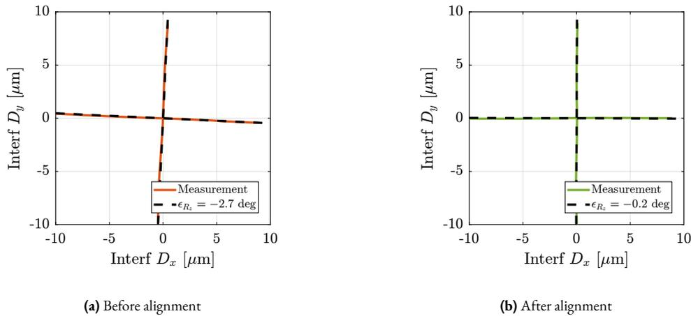
**Figure 4.86:** Measurement of the Nano-Hexapod axes in the frame of the external metrology. Before alignment (a) and after alignment (b).
