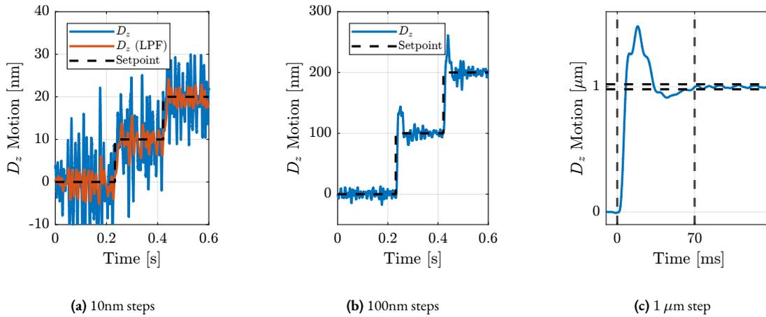
**Figure 4.108:** Vertical steps performed with the nano-hexapod. 10nm steps are shown in (a) with the low-pass filtered data corresponding to an integration time of 50 ms. 100nm steps are shown in (b). The response time to reach a peak-to-peak error of  $\pm 20$  nm is  $\approx 70$  ms as shown in (c) for a  $1 \mu\text{m}$  step.
