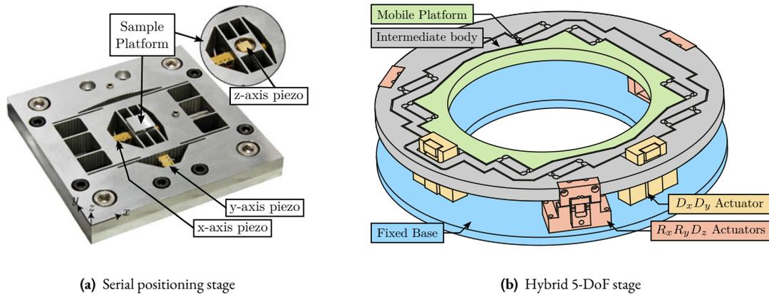
**Figure 2.102:** Examples of an XYZ serial positioning stage [76] (a) and of a 5-DoF hybrid (parallel/serial) positioning platform [128] (b).
