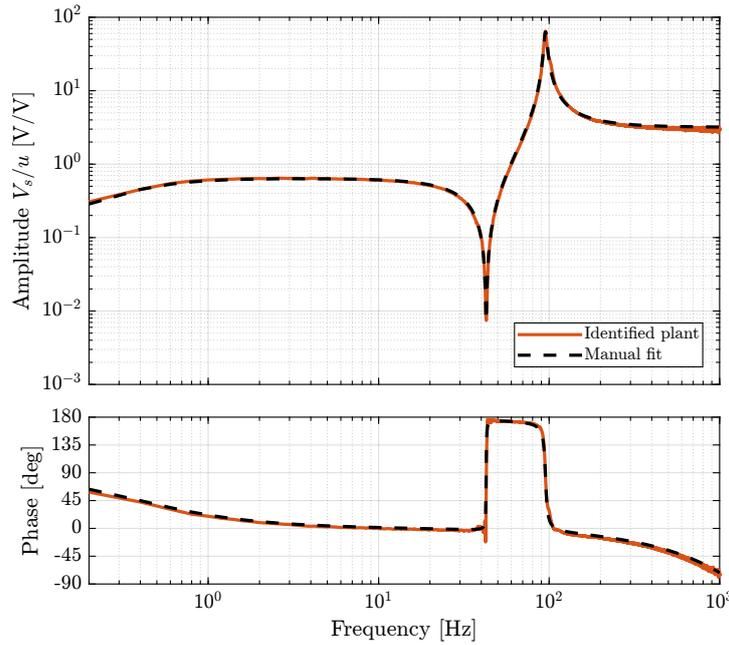
**Figure 4.17:** Identified IFF plant and manually tuned model of the plant (a time delay of  $200 \mu\text{s}$  is added to the model of the plant to better match the identified phase). Note that a minimum-phase zero is identified here even though the coherence is not good around the frequency of the zero.
