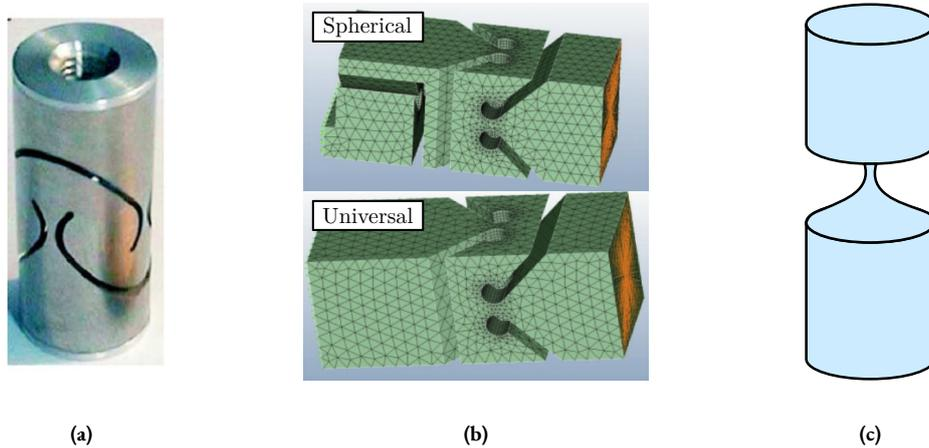
**Figure 3.35:** Example of different flexible joints geometry used for Stewart platforms. (a) Typical “universal” flexible joint used in [112]. (b) Torsional stiffness can be explicitly specified as done in [155]. (c) “Thin” flexible joints having “notch curves” are also used [38].
