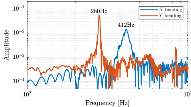
**Figure 4.9:** Frequency response functions for the two tests using the instrumented hammer and the laser vibrometer. The Y-bending mode is measured at 280 Hz and the X-bending mode at 412 Hz
