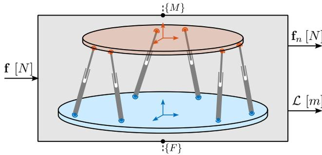
Figure 2.110: Nano-Hexapod plant with inputs and outputs. Frames  $\{F\}$  and  $\{M\}$  can be connected to other elements in the model.
