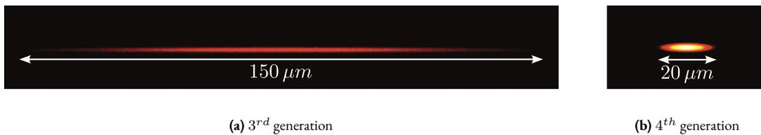
**Figure 1.8:** View of the ESRF X-ray beam before the EBS upgrade (a) and after the EBS upgrade (b). The brilliance is increased, whereas the horizontal size and emittance are reduced.
