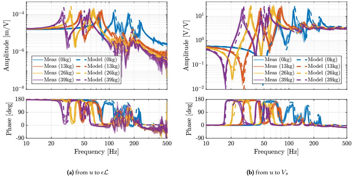
**Figure 4.89:** Comparison of the diagonal elements (i.e. “direct” terms) of the measured FRF matrix and the dynamics identified from the multi-body model. Both for the dynamics from  $u$  to  $\epsilon\mathcal{L}$  (a) and from  $u$  to  $V_s$  (b)
