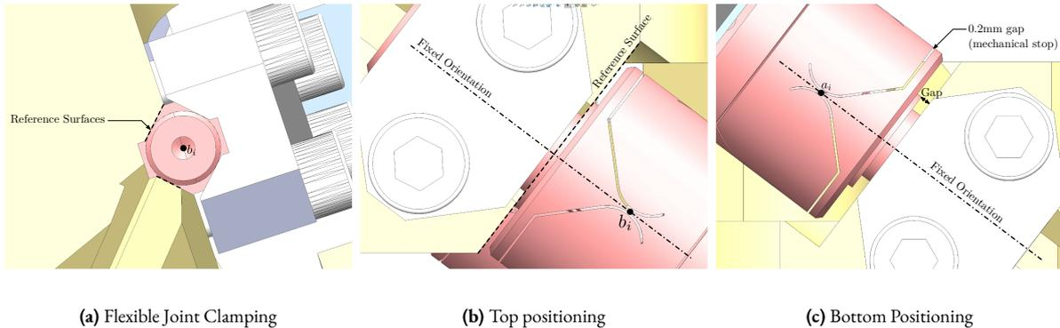
**Figure 3.96:** Fixation of the flexible points to the nano-hexapod plates. Both top and bottom flexible joints are clamped to the plates as shown in (a). While the top flexible joint is in contact with the top plate for precise positioning of its center of rotation (b), the bottom joint is just oriented (c).
