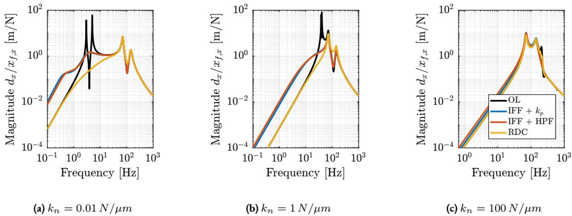
**Figure 2.60:** Effect of floor motion  $x_{f,x}$  on the position error  $d_x$  - Comparison of active damping techniques for the three nano-hexapod stiffnesses. IFF is shown to increase the sensitivity to floor motion at low-frequency.
