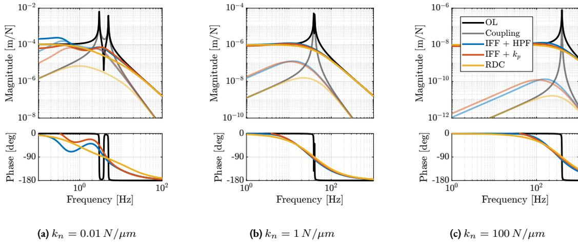
**Figure 2.57:** Comparison of the damped plants for the three proposed active damping techniques (IFF with HPF in blue, IFF with  $k_p$  in red and RDC in yellow). The direct terms are shown by solid lines, and the coupling terms are shown by the shaded lines. Three nano-hexapod stiffnesses are considered. For this analysis the rotating velocity is  $\Omega = 60$  rpm and the suspended mass is  $m_n + m_s = 16$  kg.
