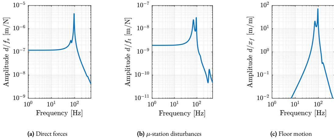
**Figure 2.5:** Sensitivity of the relative motion  $d$  to disturbances:  $f_s$  the direct forces applied on the sample (a),  $f_t$  disturbances from the micro-station stages (b) and  $x_f$  the floor motion (a)
