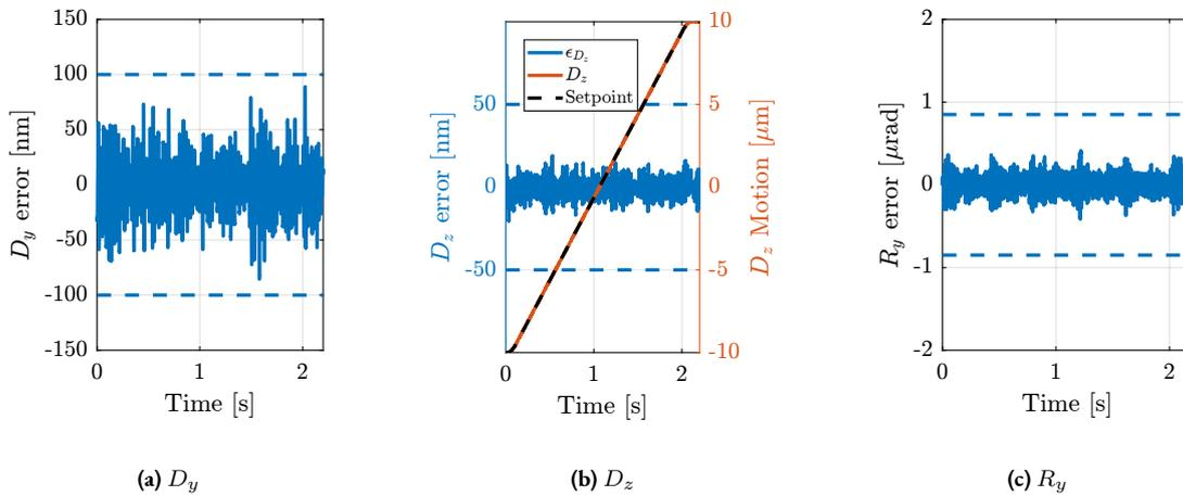
**Figure 4.109:**  $D_z$  scan at a velocity of  $10 \mu\text{m/s}$ .  $D_z$  setpoint, measured position and error are shown in (b). Errors in  $D_y$  and  $R_y$  are respectively shown in (a) and (c)
