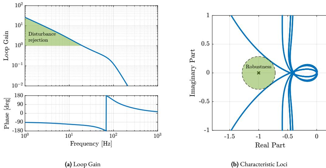
**Figure 2.121:** Decentralized HAC-IFF. Loop gain (a) is used for the design of the controller and to estimate the disturbance rejection performances. Characteristic Loci (b) is used to verify the stability and robustness of the feedback loop.
