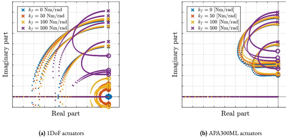
**Figure 3.37:** Effect of bending stiffness of the flexible joints on the attainable damping with decentralized IFF. When having an actuator modelled as 1DoF without parallel stiffness to the force sensor (a), and with the 2DoF model of the APA300ML (b)
