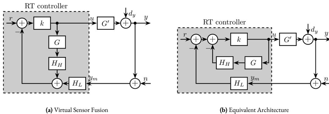
**Figure 3.64:** Control architecture for virtual sensor fusion (a). An equivalent architecture is shown in (b). The signals are the reference signal  $r$ , the output perturbation  $d_y$ , the measurement noise  $n$  and the control input  $u$ .
