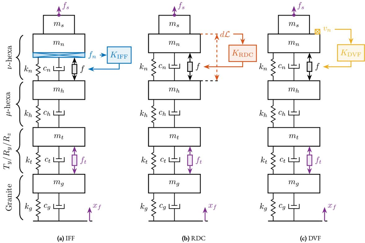
**Figure 2.12:** Three active damping strategies. Integral Force Feedback (a) using a force sensor, Relative Damping Control (b) using a relative displacement sensor, and Direct Velocity Feedback (c) using a geophone
