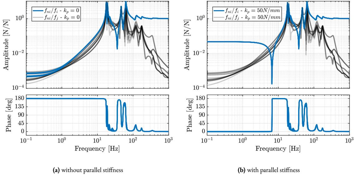
**Figure 2.125:** Effect of stiffness parallel to the force sensor on the IFF plant with  $\Omega_z = 360$  deg/s and a payload mass of 25kg. The dynamics without parallel stiffness has non-minimum phase zeros at low frequency (a). The added parallel stiffness transforms the non-minimum phase zeros into complex conjugate zeros (b)
