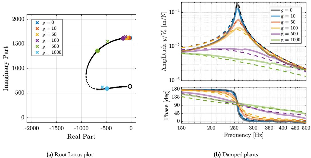
**Figure 3.28:** Results using Integral Force Feedback with the APA95ML. Closed-loop poles as a function of the controller gain  $g$  are predicted by root Locus plot (a). Circles are predictions from the model while crosses are poles estimated from the experimental data. Damped plants estimated from the model (dashed curves) and measured ones (solid curves) are compared in (b) for all tested controller gains.
