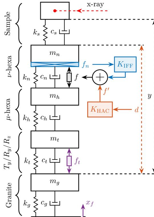
**Figure 2.35:** Uniaxial model considering some flexibility between the nano-hexapod top platform and the sample. In this case, the measured and controlled distance  $d$  is different from the distance  $y$  which is the real performance index
