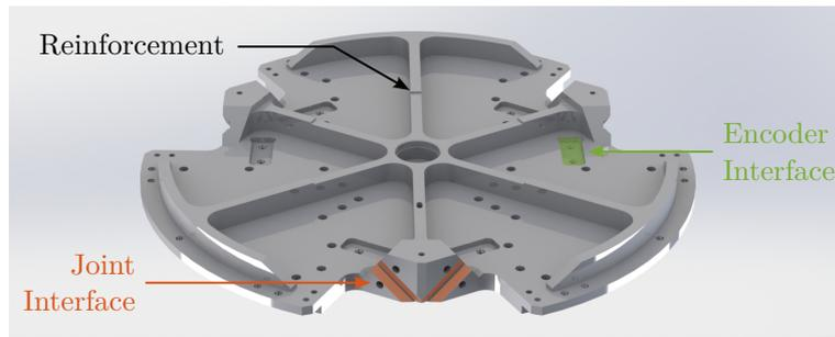
**Figure 3.95:** The mechanical design for the top platform incorporates precisely positioned V-grooves for the joint interfaces (displayed in red). The purpose of the encoder interface (shown in green) is detailed later.
