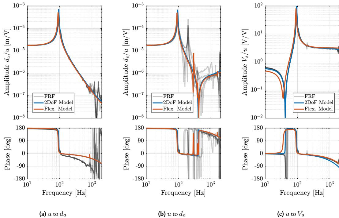
**Figure 4.51:** Comparison of the measured frequency response functions, the multi-body model using the 2 DoF APA model, and using the “flexible” APA300ML model (Super-Element extracted from a Finite Element Model).
