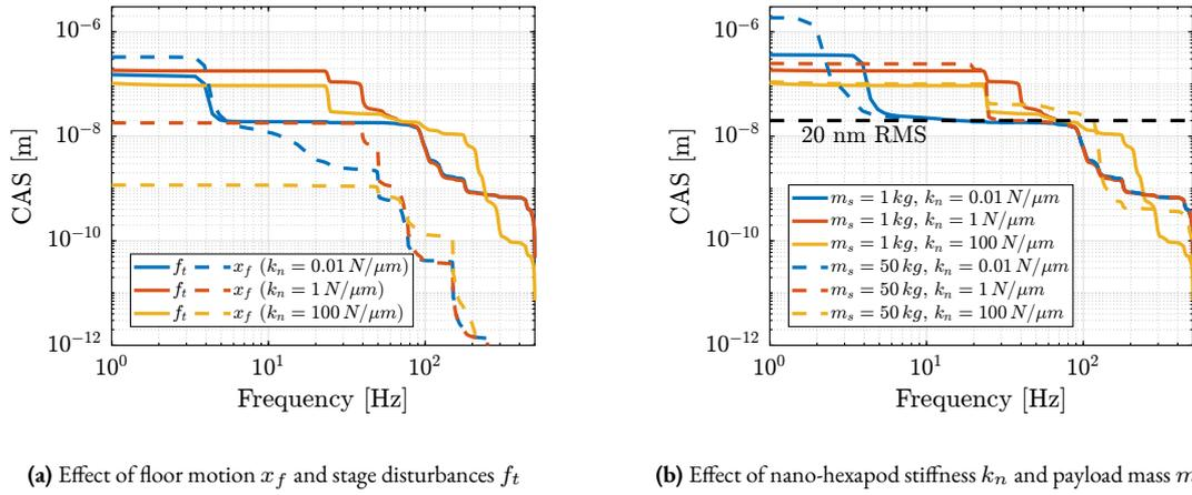
**Figure 2.11:** Cumulative Amplitude Spectrum of the relative motion  $d$ . The effect of  $x_f$  and  $f_t$  are shown in (a). The effect of sample mass for the three hexapod stiffnesses is shown in (b). The control objective of having a residual error of 20 nm RMS is shown by the horizontal black dashed line.
