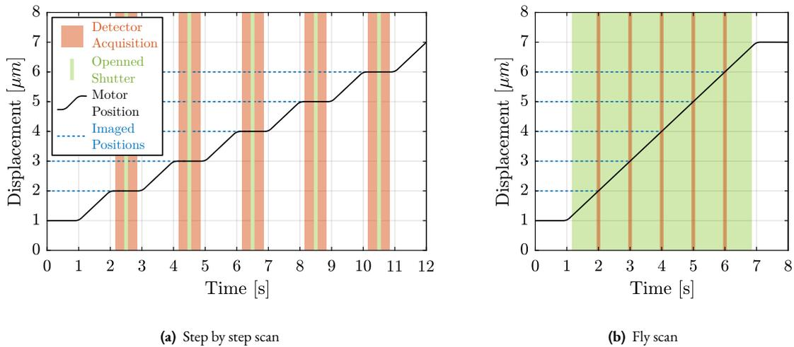
**Figure 1.10:** Two acquisition modes. In step-by-step mode (a), the motor moves at the wanted imaged position, the detector acquisition is started, the shutter is opened briefly to have the wanted exposition, the detector acquisition is stopped, and the motor can move to a new position. In *fly-scan* mode (b), the shutter is opened while the sample is in motion, and the detector is acquired only at the wanted positions, on the *fly*.
