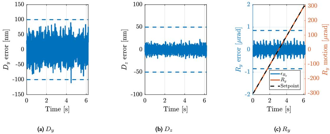
**Figure 4.107:** Reflectivity scan ( $R_y$ ) with a rotational velocity of  $100 \mu\text{rad}/\text{s}$ .
