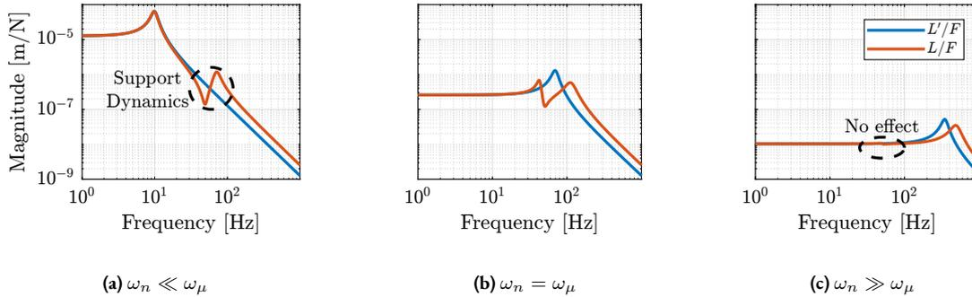
**Figure 2.30:** Effect of the support compliance on the transfer functions from  $F$  to  $L$
