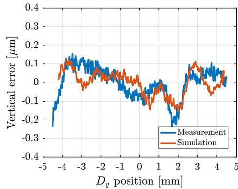
**Figure 2.99:** Vertical errors during a constant-velocity scan of the translation stage. Comparison of the measurements and simulated errors.
