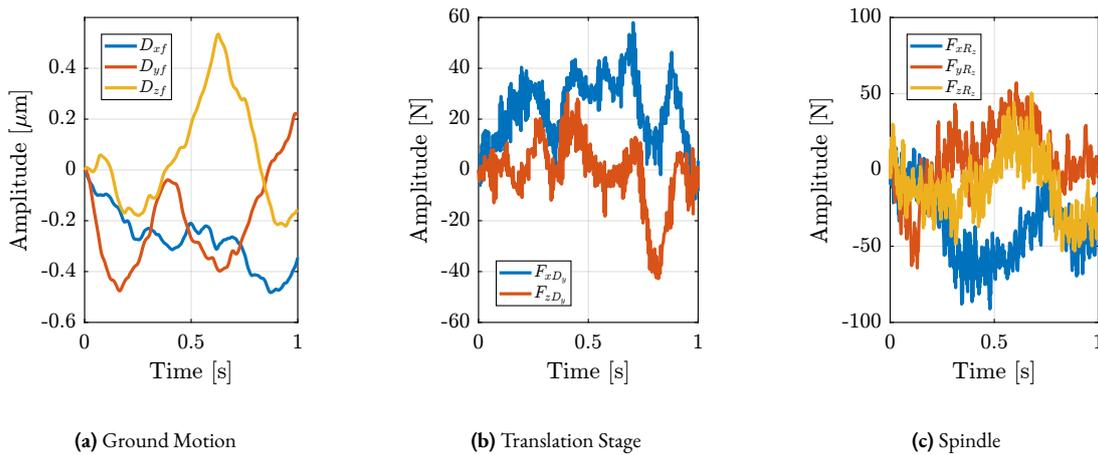
**Figure 2.97:** Generated time domain disturbance signals. Ground motion (a), translation stage (b) and spindle (c).
