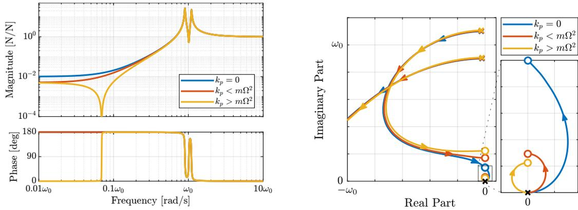
(a) Bode plot of  $G_k(1, 1) = f_u/F_u$  without parallel spring, with parallel spring stiffness  $k_p < m\Omega^2$  and  $k_p > m\Omega^2$ ,  $\Omega = 0.1\omega_0$  (b) Root Locus for IFF without parallel spring, with small parallel spring and with large parallel spring
