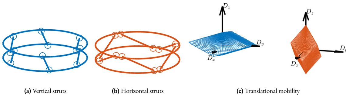
**Figure 3.5:** Effect of strut orientation on the obtained mobility in translation. Two Stewart platform geometry are considered: struts oriented vertically (a) and struts oriented horizontally (b). Obtained mobility for both geometry are shown in (c).
