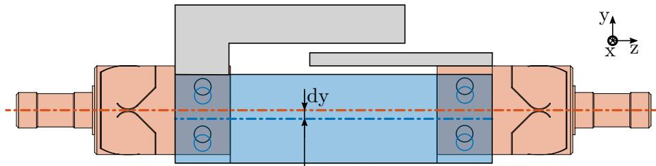
**Figure 4.52:** Mis-alignment between the joints and the APA
