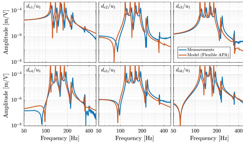
**Figure 4.74:** Comparison of the measured (in blue) and modeled (in red) frequency transfer functions from the first control signal  $u_1$  to the six encoders  $d_{e1}$  to  $d_{e6}$ . The APA are here modeled with a “super-element”.
