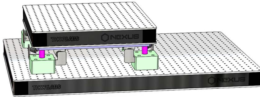
**Figure 4.60:** CAD View of the vibration table. The purple cylinders are representing the soft springs.
