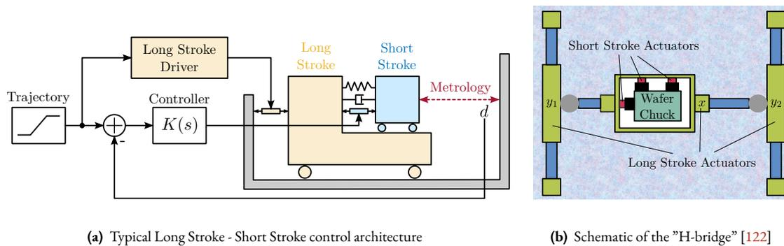
(a) Typical Long Stroke - Short Stroke control architecture
