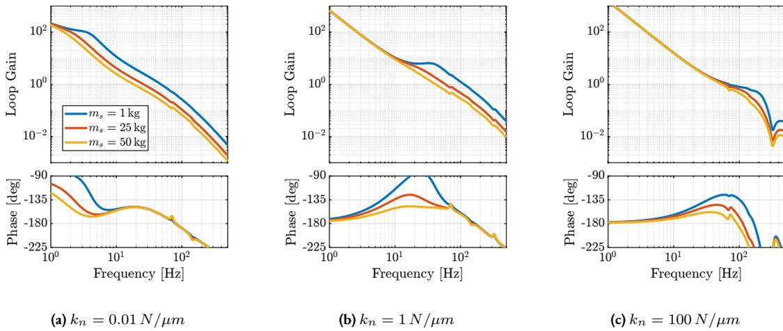
**Figure 2.25:** Loop gain for the High Authority Controller
