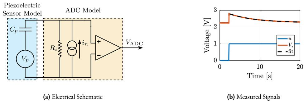
**Figure 3.80:** Electrical schematic of the ADC measuring the piezoelectric force sensor (a), adapted from [96]. Measured voltage  $V_s$  while step voltages are generated for the actuator stacks (b).
