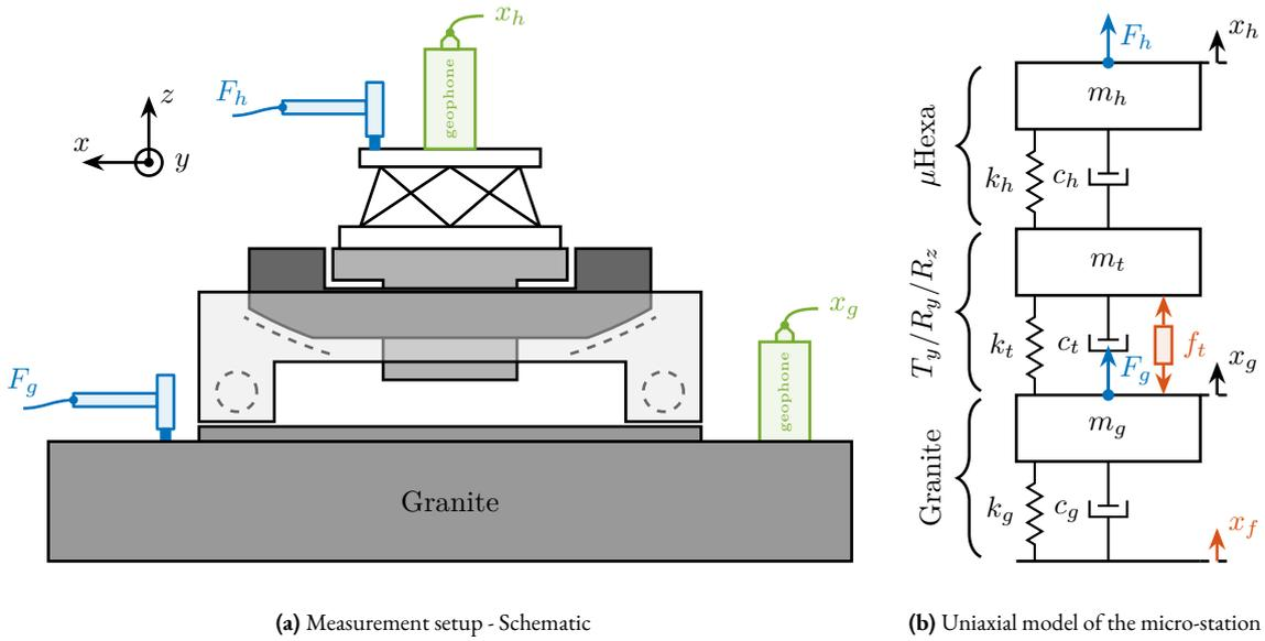
**Figure 2.2:** Schematic of the Micro-Station measurement setup and uniaxial model.
