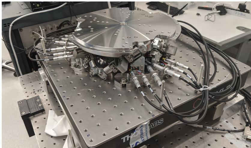
**Figure 4.63:** Mounted Nano-Hexapod on top of the suspended table
