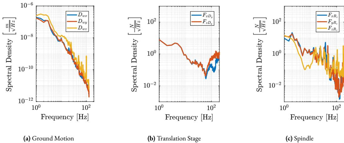
**Figure 2.96:** Measured spectral density of the micro-station disturbance sources. Ground motion (a), translation stage (b) and spindle (c).
