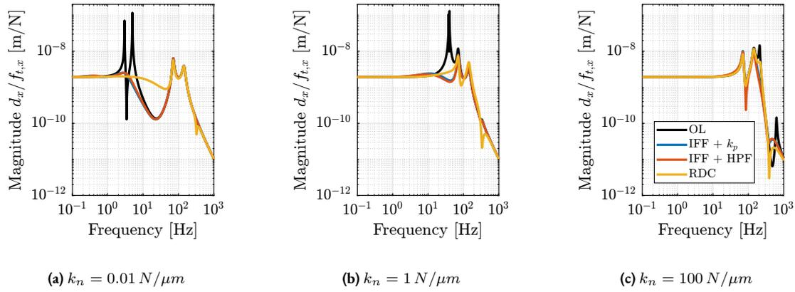
**Figure 2.61:** Effect of micro-station vibrations  $f_{t,x}$  on the position error  $d_x$  - Comparison of active damping techniques for the three nano-hexapod stiffnesses. Relative Damping Control increases the sensitivity to micro-station vibrations between the soft nano-hexapod suspension modes and the micro-station modes (a)
