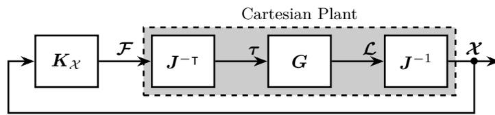
**Figure 3.10:** Typical control architecture in the cartesian frame
