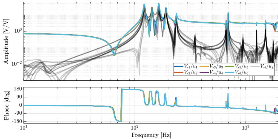
**Figure 4.68:** Measured FRF for the transfer function from  $\mathbf{u}$  to  $\mathbf{V}_s$ . The 6 diagonal terms are the colored lines (all superimposed), and the 30 off-diagonal terms are the shaded black lines.
