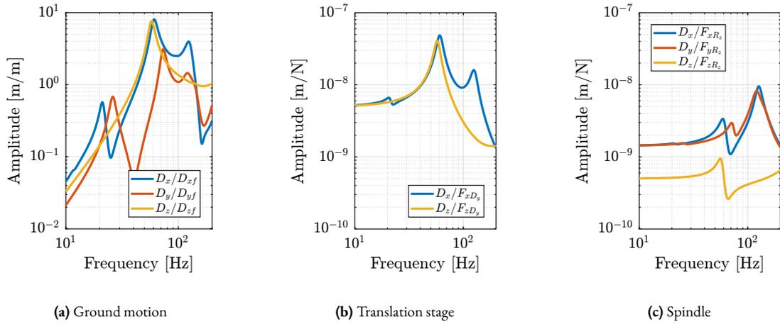
**Figure 2.95:** Extracted transfer functions from disturbances to relative motion between the micro-station’s top platform and the granite. The considered disturbances are the ground motion (a), the translation stage vibrations (b), and the spindle vibrations (c).
