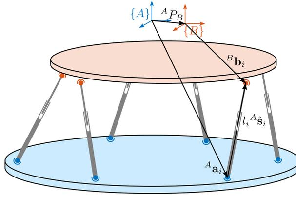
**Figure 2.106:** Notations to compute the kinematic loop closure
