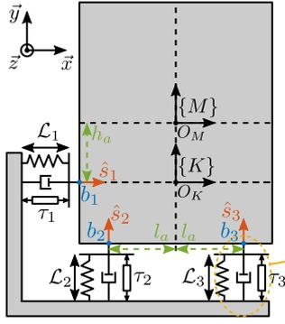
Figure 3.54: Model used to compare decoupling strategies
