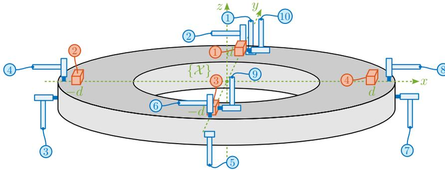
**Figure 2.87:** Schematic of the measurement setup used to estimate the compliance of the micro-station. The top platform of the positioning hexapod is shown with four 3-axis accelerometers (shown in red) are on top. 10 hammer impacts are performed at different locations (shown in blue).
