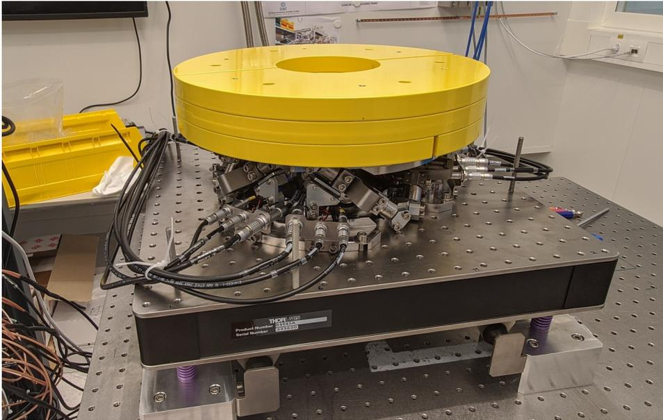
**Figure 4.69:** Picture of the nano-hexapod with the added three cylindrical masses for a total of  $\approx 40$  kg
