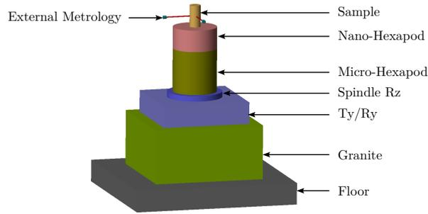
**Figure 2.58:** 3D view of the Nano-Active-Stabilization-System model.
