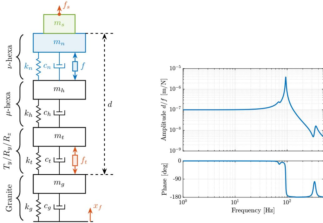
(a) Uniaxial mass-spring-damper model of the NASS (b) Bode Plot of the transfer function from actuator forces  $f$  to measured displacement  $d$  by the metrology
