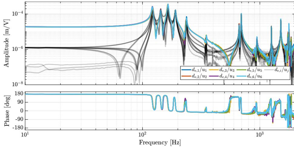
**Figure 4.67:** Measured FRF for the transfer function from  $\mathbf{u}$  to  $\mathbf{d}_e$ . The 6 diagonal terms are the colored lines (all superimposed), and the 30 off-diagonal terms are the gray lines.
