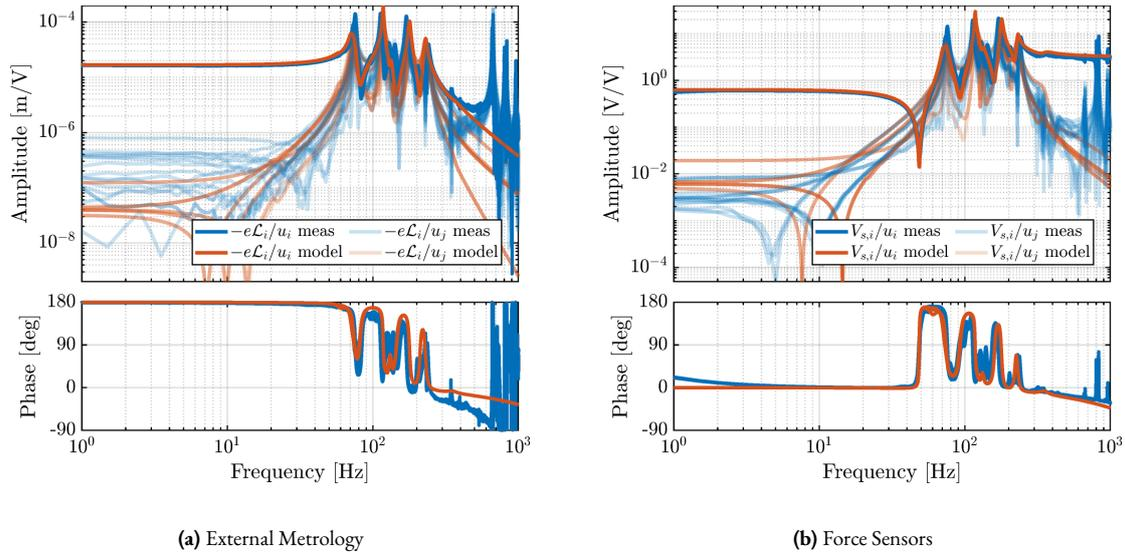
**Figure 4.85:** Comparison between the measured dynamics and the multi-body model dynamics. Both for the external metrology (a) and force sensors (b). Direct terms are displayed with solid lines while off-diagonal (i.e. coupling) terms are displayed with shaded lines.
