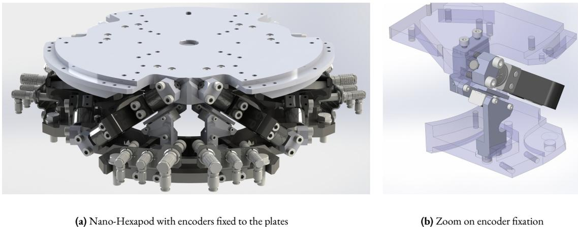
**Figure 3.98:** Alternative way of using the encoders: they are fixed directly to the plates.
