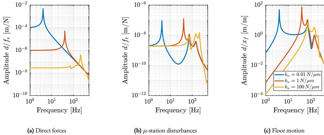
**Figure 2.10:** Sensitivity of  $d$  to disturbances for three different nano-hexapod stiffnesses.  $f_s$  the direct forces applied on the sample (a),  $f_t$  disturbances from the micro-station stages (b) and  $x_f$  the floor motion (a)
