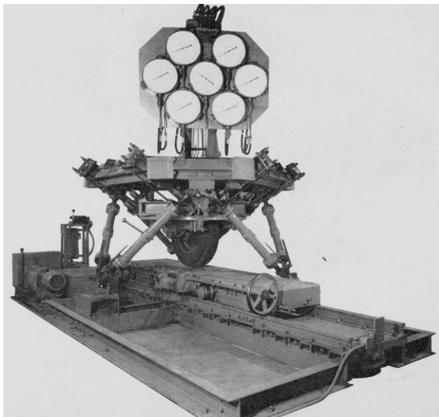
(a) Tyre test machine proposed by Gough [52]
