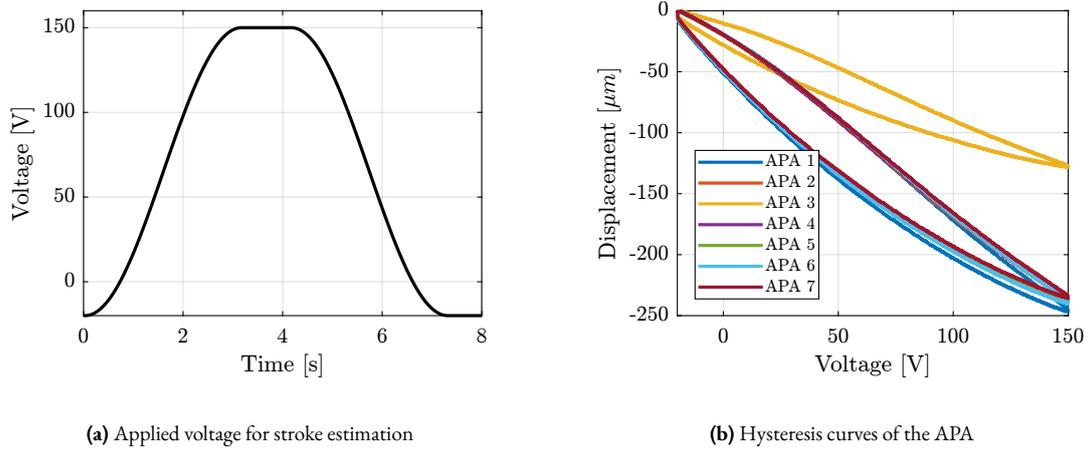
**Figure 4.6:** Generated voltage across the two piezoelectric stack actuators to estimate the stroke of the APA300ML (a). Measured displacement as a function of applied voltage (b)
