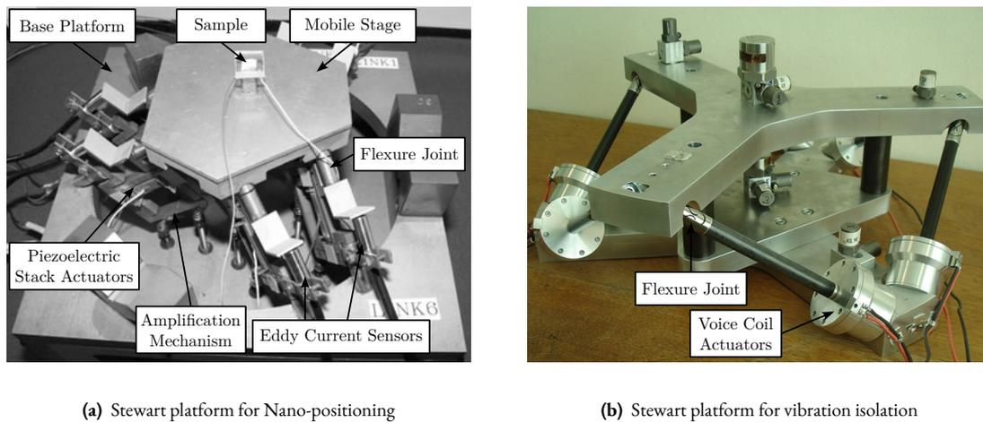
**Figure 2.103:** Two examples of Stewart platform. A Stewart platform based on piezoelectric stack actuators and used for nano-positioning is shown in (a) [48]. A Stewart platform based on voice coil actuators and used for vibration isolation is shown in (b) [108, 112]
