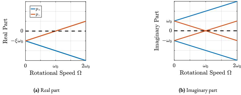
Figure 2.38: Campbell diagram - Real (a) and Imaginary (b) parts of the poles as a function of the rotating velocity  $\Omega$ .
