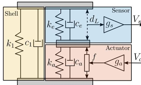
**Figure 4.21:** Schematic of the two degrees-of-freedom model of the APA300ML, adapted from [130]
