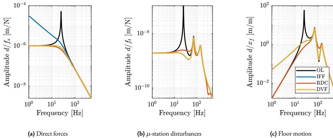
**Figure 2.20:** Change of sensitivity to disturbance with all three active damping strategies.  $f_s$  the direct forces applied on the sample (a),  $f_t$  disturbances from the micro-station stages (b) and  $x_f$  the floor motion (a)
