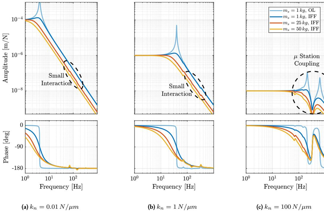
Figure 2.23: Obtained damped plant using Integral Force Feedback for three sample masses
