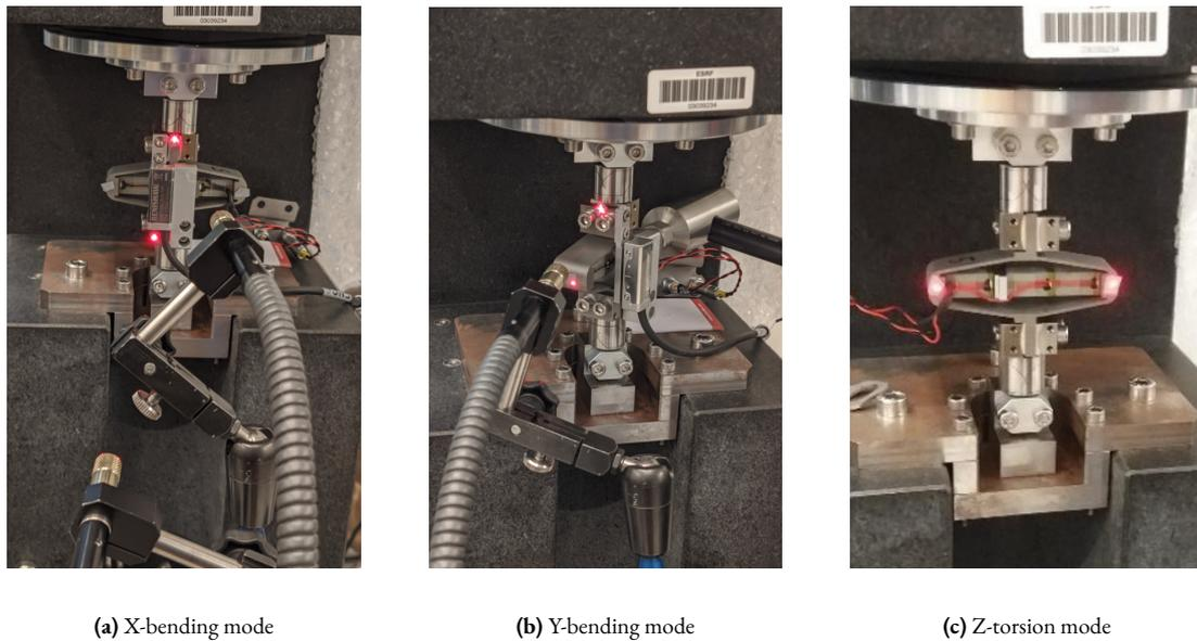
**Figure 4.44:** Measurement of strut flexible modes
