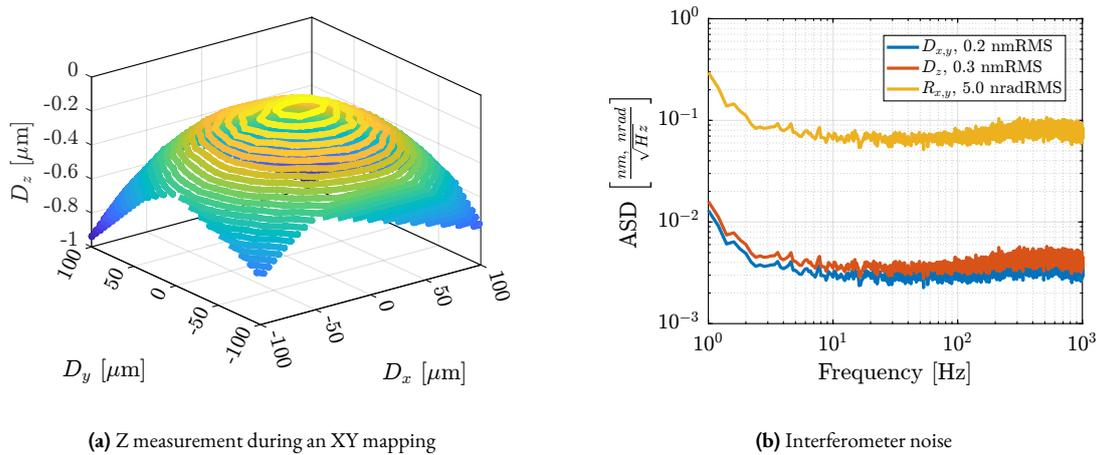
**Figure 4.83:** Estimated measurement errors of the metrology. Cross-coupling between lateral motion and vertical measurement is shown in (a). The effect of interferometer noise on the measured translations and rotations is shown in (b).
