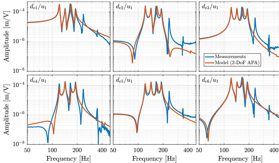
**Figure 4.73:** Comparison of the measured (in blue) and modeled (in red) frequency transfer functions from the first control signal  $u_1$  to the six encoders  $d_{e1}$  to  $d_{e6}$ . The APA are here modeled with a 2-DoF mass-spring-damper system.
