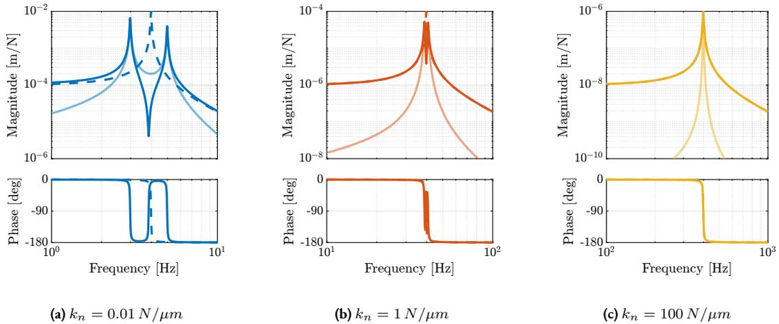
**Figure 2.53:** Effect of rotation on the nano-hexapod dynamics. Dashed lines represent plants without rotation, solid lines represent plants at maximum rotating velocity ( $\Omega = 60 \text{ rpm}$ ), and shaded lines are coupling terms at maximum rotating velocity
