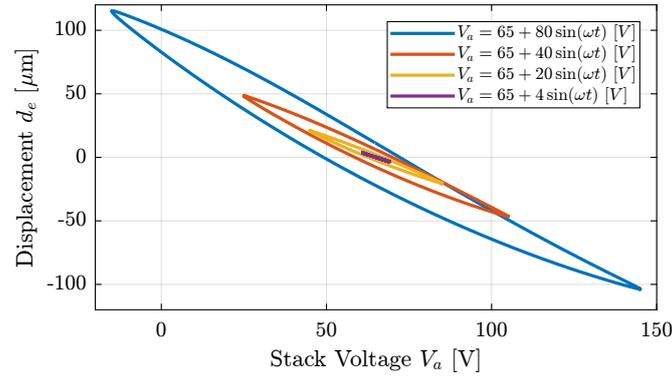
**Figure 4.12:** Displacement as a function of applied voltage for multiple excitation amplitudes
