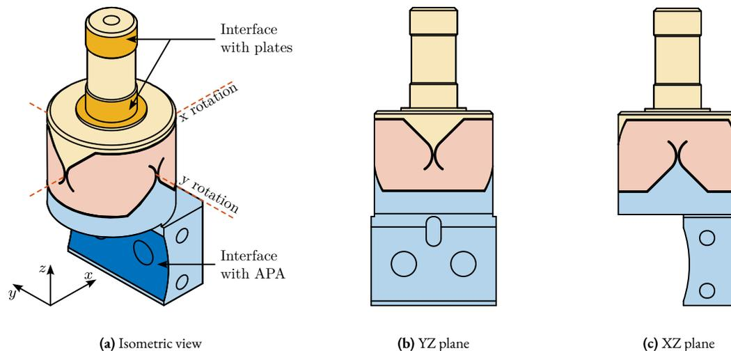
**Figure 4.26:** Geometry of the optimized flexible joints
