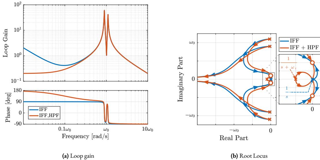
**Figure 2.42:** Comparison of the IFF with pure integrator and modified IFF with added high-pass filter ( $\Omega = 0.1\omega_0$ ). The loop gain is shown in (a) with  $\omega_i = 0.1\omega_0$  and  $g = 2$ . The root locus is shown in (b)
