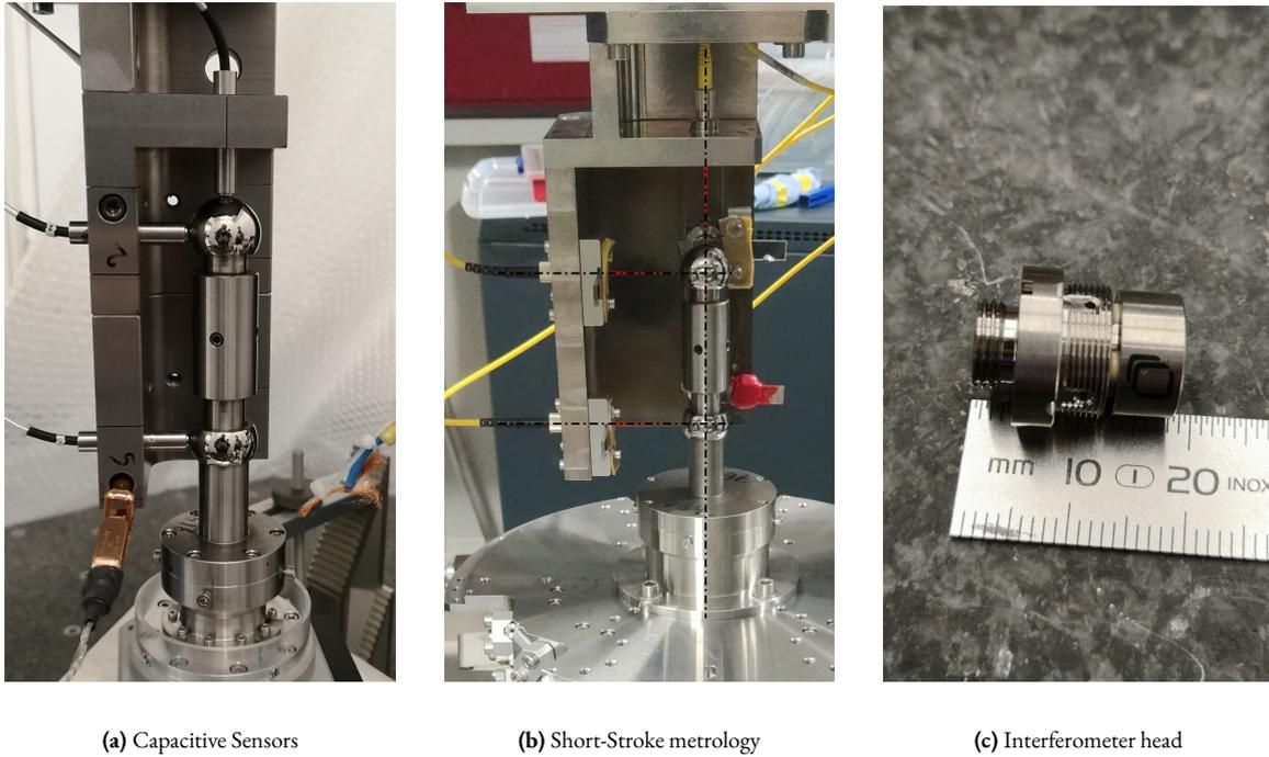
**Figure 4.78:** Short stroke metrology system used to measure the sample position with respect to the granite in 5DoF. The system is based on a “Spindle error analyzer” (a), but the capacitive sensors are replaced with fibered interferometers (b). The interferometer heads are shown in (c)
