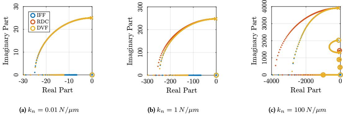
**Figure 2.17:** Root Loci for the three active damping techniques (IFF in blue, RDC in red and DVF in yellow). This is shown for the three nano-hexapod stiffnesses. The Root Loci are zoomed in the suspension mode of the nano-hexapod.
