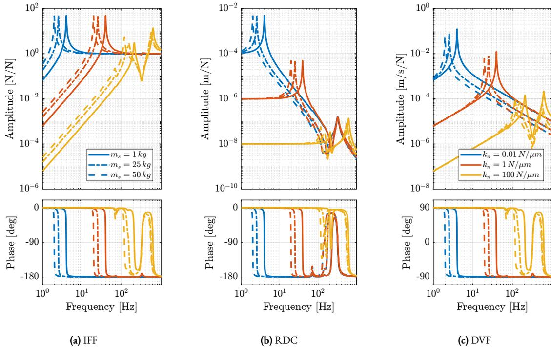
**Figure 2.16:** Plant dynamics for the three active damping techniques (IFF: **a**, RDC: **b**, DVF: **c**), for three nano-hexapod stiffnesses ( $k_n = 0.01 \text{ N}/\mu\text{m}$  in blue,  $k_n = 1 \text{ N}/\mu\text{m}$  in red and  $k_n = 100 \text{ N}/\mu\text{m}$  in yellow) and three sample's masses ( $m_s = 1 \text{ kg}$ : solid curves,  $m_s = 25 \text{ kg}$ : dot-dashed curves, and  $m_s = 50 \text{ kg}$ : dashed curves).
