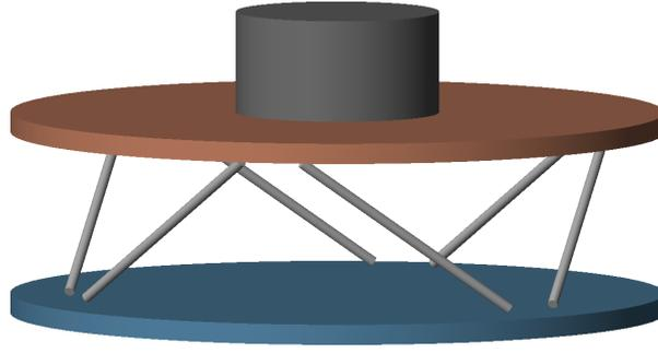
**Figure 3.11:** Cubic Stewart platform with top cylindrical payload
