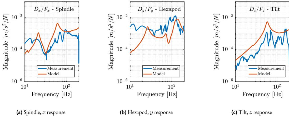
**Figure 2.86:** FRFs between the hammer impacts on the translation stage and the measured stage acceleration expressed at its CoM. Comparison of the measured and extracted FRFs from the multi-body model. Different directions are computed for different stages.
