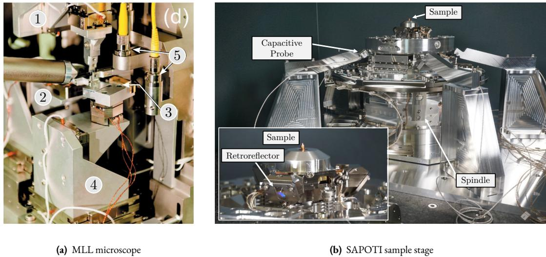
**Figure 2.100:** Example of sample stage with active XYZ corrections based on external metrology. The MLL microscope [101] at NSLS-II (a). Sample stage on SAPOTI beamline [51] at Sirius facility (b)
