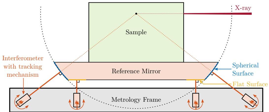
**Figure 1.17:** 2D representation of the NASS metrology system.
