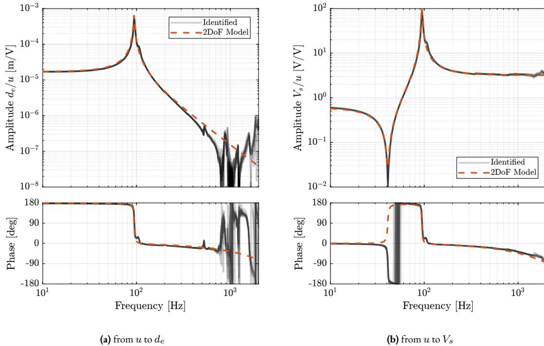
**Figure 4.23:** Comparison of the measured frequency response functions and the identified dynamics from the 2DoF model of the APA300ML. Both for the dynamics from  $u$  to  $d_e$  (a) and from  $u$  to  $V_s$  (b)
