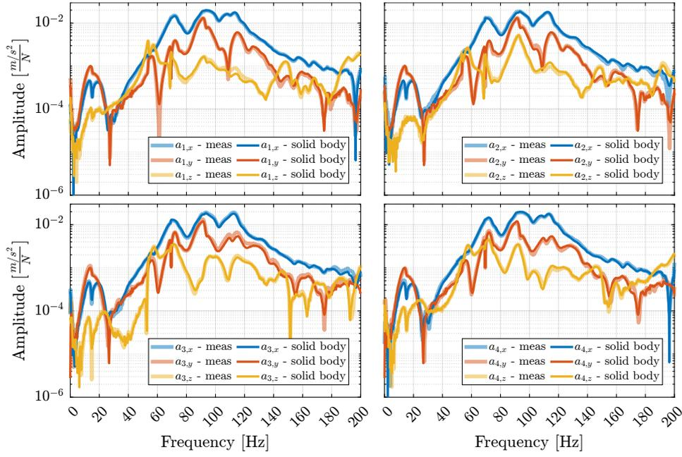
**Figure 2.71:** Comparison of the original accelerometer responses and the reconstructed responses from the solid body response. Accelerometers 1 to 4 corresponding to the micro-hexapod are shown. Input is a hammer force applied on the micro-hexapod in the  $x$  direction
