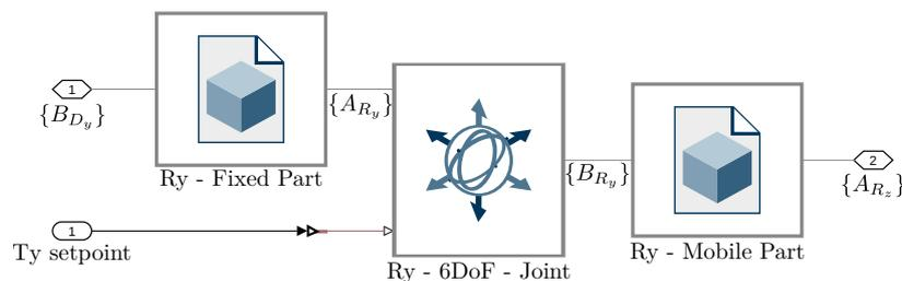
**Figure 2.84:** Example of a stage (here the tilt-stage) represented in the multi-body model software (Simulink - Simscape). It is composed of two solid bodies connected by a 6-DoF joint. One joint DoF (here the tilt angle) can be imposed, the other DoFs are represented by springs and dampers. Additional disturbing forces for all DoF can be included
