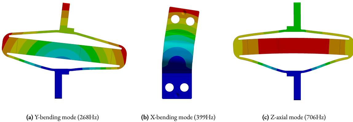
**Figure 4.7:** First three modes of the APA300ML in a fix-free condition estimated from a Finite Element Model
