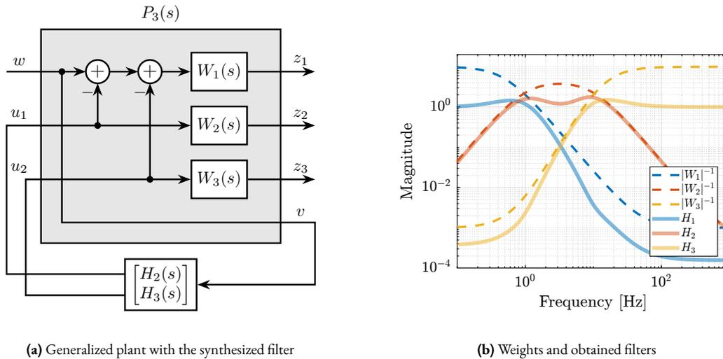
(a) Generalized plant with the synthesized filter
