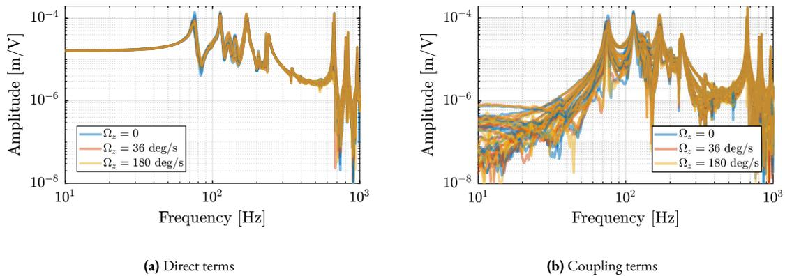
**Figure 4.90:** Effect of the spindle rotation on the plant dynamics from  $u$  to  $\epsilon\mathcal{L}$ . Three rotational velocities are tested (0 deg/s, 36 deg/s and 180 deg/s). Both direct terms (a) and coupling terms (b) are displayed.
