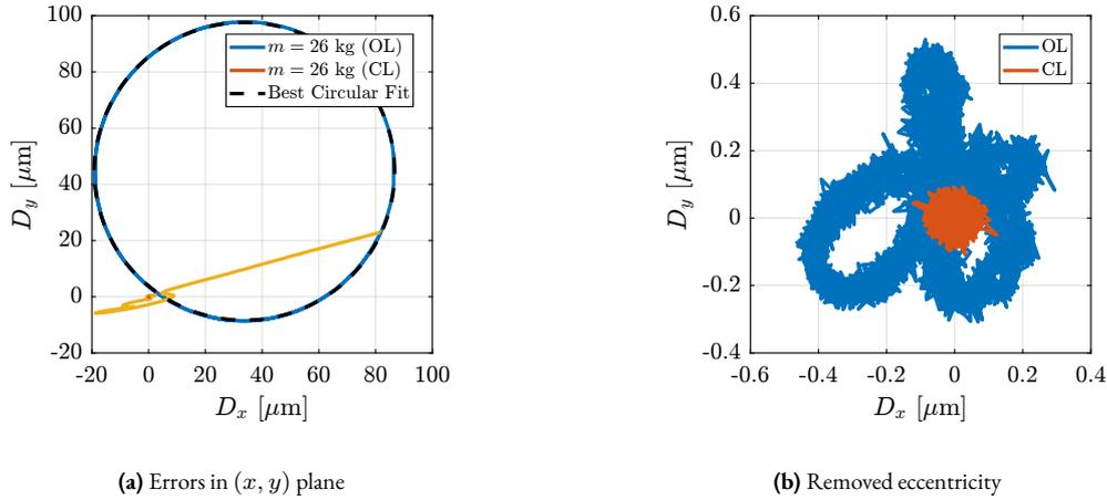
**Figure 4.103:** Tomography experiment with a rotation velocity of 6 deg/s, and payload mass of 26kg. Errors in the  $(x, y)$  plane are shown in (a). The estimated eccentricity is represented by the black dashed circle. The errors with subtracted eccentricity are shown in (b).
