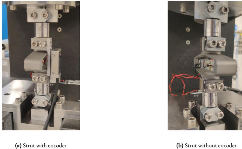
**Figure 4.47:** Struts fixed to the test bench with clamped flexible joints. The coder can be fixed to the struts (a) or removed (b)
