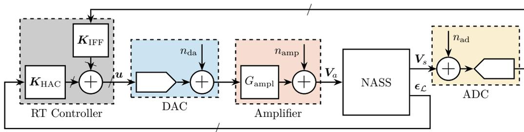
**Figure 3.72:** Block diagram of the NASS with considered instrumentation. The real time controller is a Speedgoat machine.
