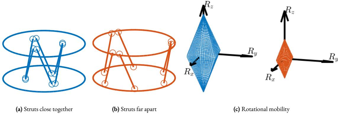
**Figure 3.6:** Effect of strut position on the obtained mobility in rotation. Two Stewart platform geometry are considered: struts close to each other (a) and struts further apart (b). Obtained mobility for both geometry are shown in (c).
