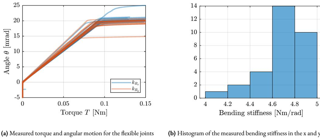
**Figure 4.37:** Result of measured  $k_{R_x}$  and  $k_{R_y}$  stiffnesses for the 16 flexible joints. Raw data are shown in (a). A histogram of the measured stiffnesses is shown in (b).
