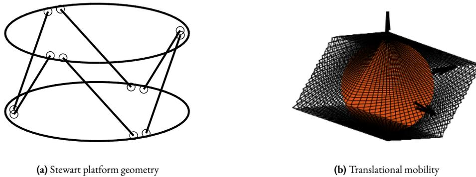
**Figure 3.4:** One Stewart platform geometry (a) and its associated translational mobility (b). A sphere with radius equal to the strut stroke is contained in the translational mobility shape.
