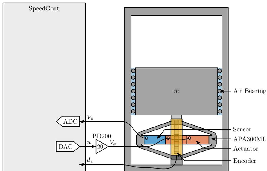
**Figure 4.11:** Schematic of the Test Bench used to measure the dynamics of the APA300ML.  $u$  is the output DAC voltage,  $V_a$  the output amplifier voltage (i.e. voltage applied across the actuator stacks),  $d_e$  the measured displacement by the encoder and  $V_s$  the measured voltage across the sensor stack.
