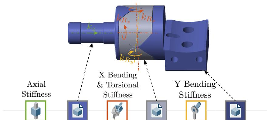
**Figure 3.100:** 4DoF multi-body model of the flexible joints
