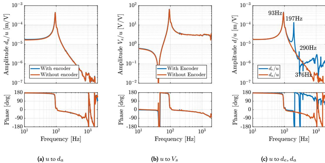
**Figure 4.48:** Effect of having the encoder fixed to the struts on the measured dynamics from  $u$  to  $d_a$  (a) and from  $u$  to  $V_s$  (b). Comparison of the observed dynamics by the encoder and interferometers (c)
