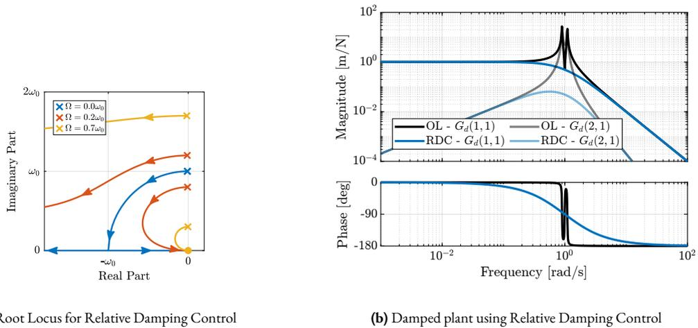
**Figure 2.50:** Relative Damping Control. Root Locus (a) and obtained damped plant (b)
