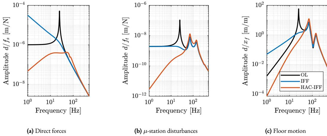
**Figure 2.26:** Change of sensitivity to disturbances with LAC and with HAC-LAC. A nano-Hexapod with  $k_n = 1 \text{ N}/\mu\text{m}$  and a sample mass of  $25 \text{ kg}$  is used.  $f_s$  the direct forces applied on the sample (a),  $f_t$  disturbances from the micro-station stages (b) and  $x_f$  the floor motion (a)
