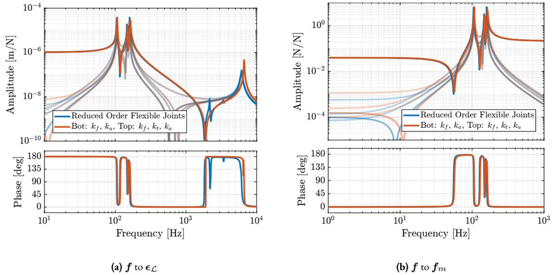
**Figure 3.42:** Comparison of the dynamics obtained between a nano-hexpod including joints modelled with FEM and a nano-hexpod having bottom joint modelled by bending stiffness  $k_f$  and axial stiffness  $k_a$  and top joints modelled by bending stiffness  $k_f$ , torsion stiffness  $k_t$  and axial stiffness  $k_a$ . Both from actuator force  $f$  to strut motion measured by external metrology  $\epsilon_{\mathcal{L}}$  (b) and to the force sensors  $f_m$  (a).
