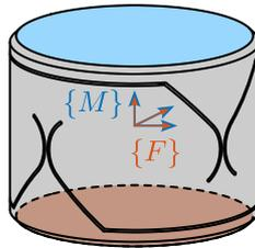
**Figure 3.41:** Defined frames for the reduced order flexible body. The two flat interfaces are considered rigid, and are linked to the two frames  $\{F\}$  and  $\{M\}$  both located at the center of the rotation.
