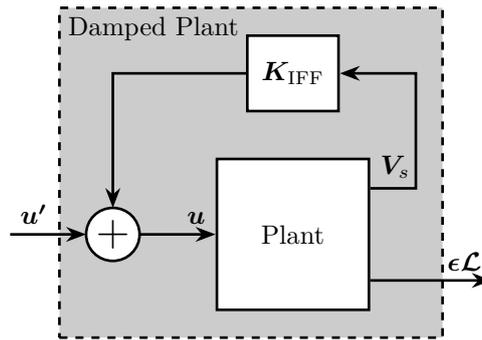
**Figure 4.91:** Block diagram of the implemented decentralized IFF controller. The controller  $\mathbf{K}_{\text{IFF}}$  is a diagonal controller with the same elements for every diagonal term  $K_{\text{IFF}}$ .
