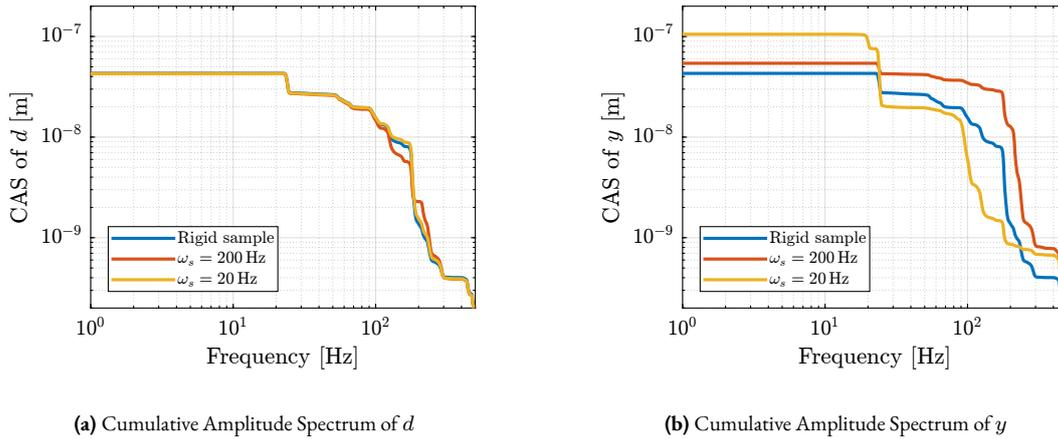
**Figure 2.36:** Cumulative Amplitude Spectrum of the distances  $d$  and  $y$ . The effect of the sample’s flexibility does not affect much  $d$  but is detrimental to the stability of  $y$ . A sample mass  $m_s = 1$  kg and a nano-hexapod stiffness of  $100$  N/ $\mu$ m are used for the simulations.
