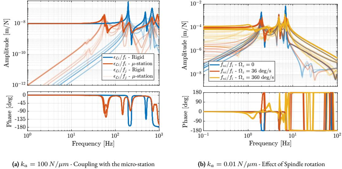
**Figure 2.132:** Coupling between a stiff nano-hexapod ( $k_a = 100 \text{ N}/\mu\text{m}$ ) and the micro-station (a). Large effect of the spindle rotational velocity for a compliance ( $k_a = 0.01 \text{ N}/\mu\text{m}$ ) nano-hexapod (b)
