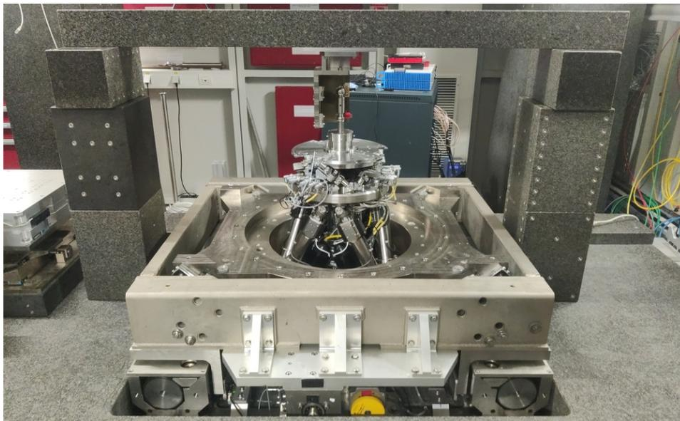
**Figure 4.81:** Granite gantry used to fix the short-stroke metrology system
