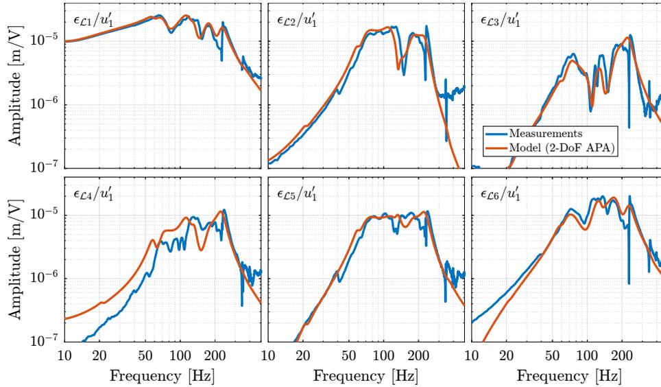
**Figure 4.97:** Comparison of the measured (in blue) and modeled (in red) frequency transfer functions from the first control signal ( $u'_1$ ) of the damped plant to the estimated errors ( $\epsilon_{\mathcal{L}_i}$ ) in the frame of the six struts by the external metrology
