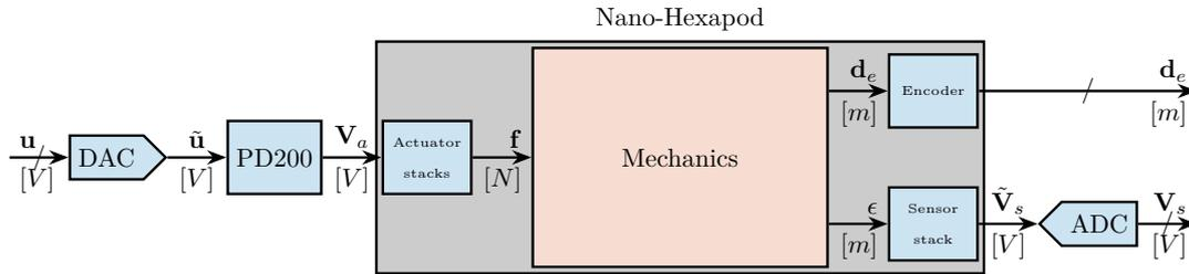
**Figure 4.64:** Block diagram of the studied system. The command signal generated by the speedgoat is  $\mathbf{u}$ , and the measured signals are  $\mathbf{d}_e$  and  $\mathbf{V}_s$ . Units are indicated in square brackets.
