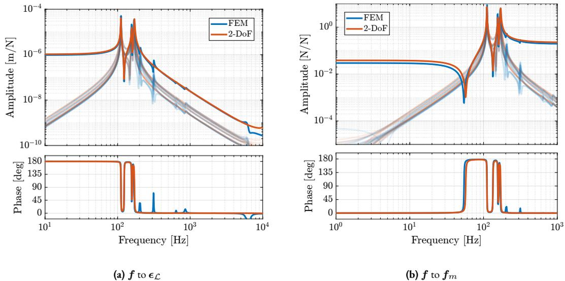
**Figure 3.34:** Comparison of the dynamics obtained between a nano-hexapod having the actuators modeled with FEM and a nano-hexapod having actuators modelled a 2DoF system. Both from actuator force  $\mathbf{f}$  to strut motion measured by external metrology  $\epsilon_{\mathcal{L}}$  (b) and to the force sensors  $\mathbf{f}_m$  (a).
