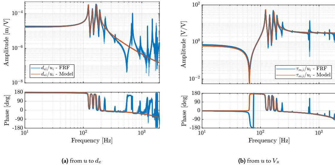
**Figure 4.72:** Comparison of the diagonal elements (i.e. “direct” terms) of the measured FRF matrix and the dynamics identified from the multi-body model. Both for the dynamics from  $u$  to  $d_e$  (a) and from  $u$  to  $V_s$  (b)
