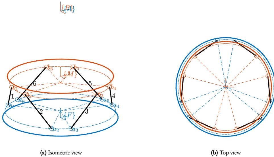
**Figure 3.21:** Obtained architecture for the Nano Hexapod
