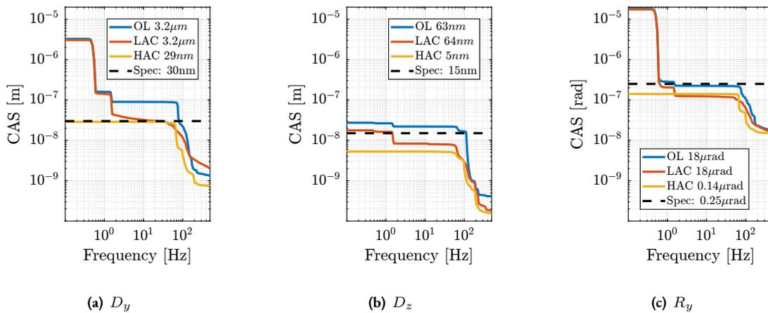
**Figure 4.106:** Cumulative Amplitude Spectrum for tomography experiments at 180 deg/s. Open-Loop case, IFF, and HAC-LAC are compared. Specifications are indicated by black dashed lines. The RMS values are indicated in the legend.
