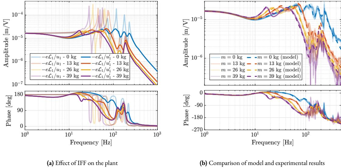
**Figure 4.95:** Comparison of the open-loop plants and the damped plant with Decentralized IFF, estimated from the multi-body model (a). Comparison of measured damped and modeled plants for all considered payloads (b). Only “direct” terms ( $\epsilon\mathcal{L}_i/u'_i$ ) are displayed for simplicity
