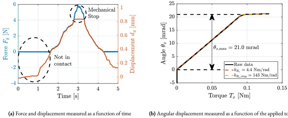
**Figure 4.36:** Results obtained on the first flexible joint. The measured force and displacement are shown in (a). The estimated angular displacement  $\theta_x$  as a function of the estimated applied torque  $T_x$  is shown in (b). The bending stiffness  $k_{R_x}$  of the flexible joint can be estimated by computing a best linear fit (red dashed line).
