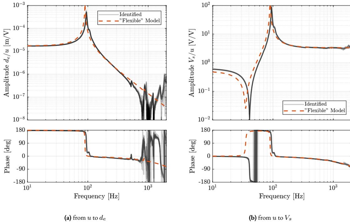
**Figure 4.25:** Comparison of the measured frequency response functions and the identified dynamics from the finite element model of the APA300ML. Both for the dynamics from  $u$  to  $d_e$  (a) and from  $u$  to  $V_s$  (b)
