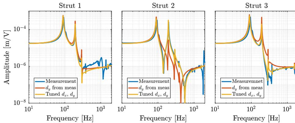
**Figure 4.54:** Comparison of the frequency response functions from DAC voltage  $u$  to measured displacement  $d_e$  by the encoders for the three struts. In blue, the measured dynamics is reprinted, in red the dynamics extracted from the model with the  $y$  misalignment estimated from measurements, and in yellow, the dynamics extracted from the model when both the  $x$  and  $y$  misalignments are tuned
