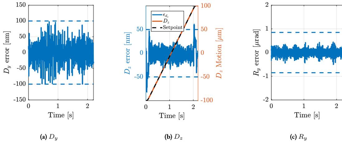
**Figure 4.110:**  $D_z$  scan at a velocity of  $100 \mu\text{m}/\text{s}$ .  $D_z$  setpoint, measured position and error are shown in (b). Errors in  $D_y$  and  $R_y$  are respectively shown in (a) and (c)
