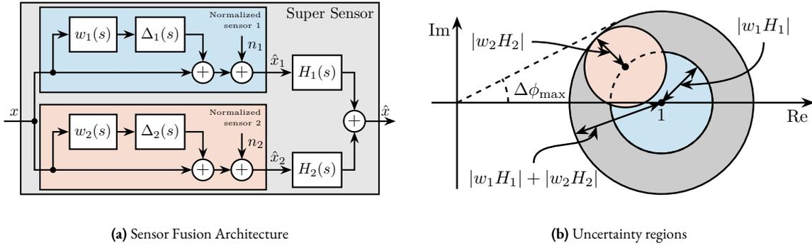
**Figure 3.48:** Sensor fusion architecture with sensor dynamics uncertainty (a). Uncertainty region (b) of the super sensor dynamics in the complex plane (grey circle). The contribution of both sensors 1 and 2 to the total uncertainty are represented respectively by a blue circle and a red circle. The frequency dependency  $\omega$  is here omitted.
