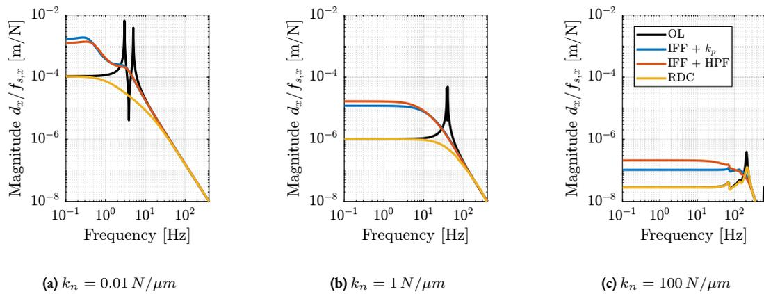
**Figure 2.62:** Effect of sample forces  $f_{s,x}$  on the position error  $d_x$  - Comparison of active damping techniques for the three nano-hexapod stiffnesses. Integral Force Feedback degrades this compliance at low-frequency.
