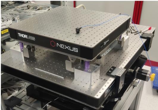
**Figure 4.61:** Mounted suspended table. Only 1 or the 15 accelerometers is mounted on top
