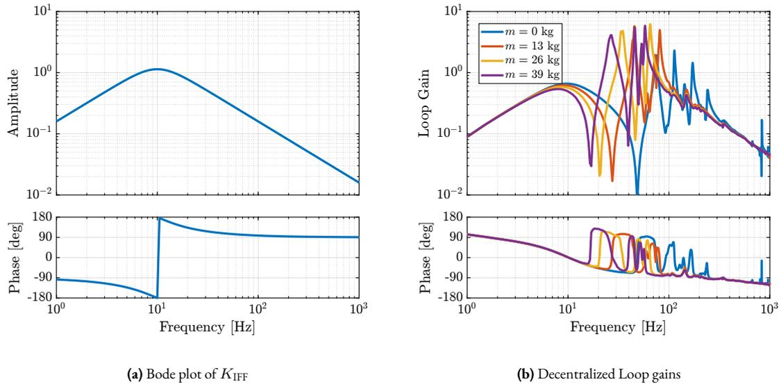
**Figure 4.93:** Bode plot of the decentralized IFF controller (a). The decentralized controller  $K_{\text{IFF}}$  multiplied by the identified dynamics from  $u_1$  to  $V_{s1}$  for all payloads are shown in (b)
