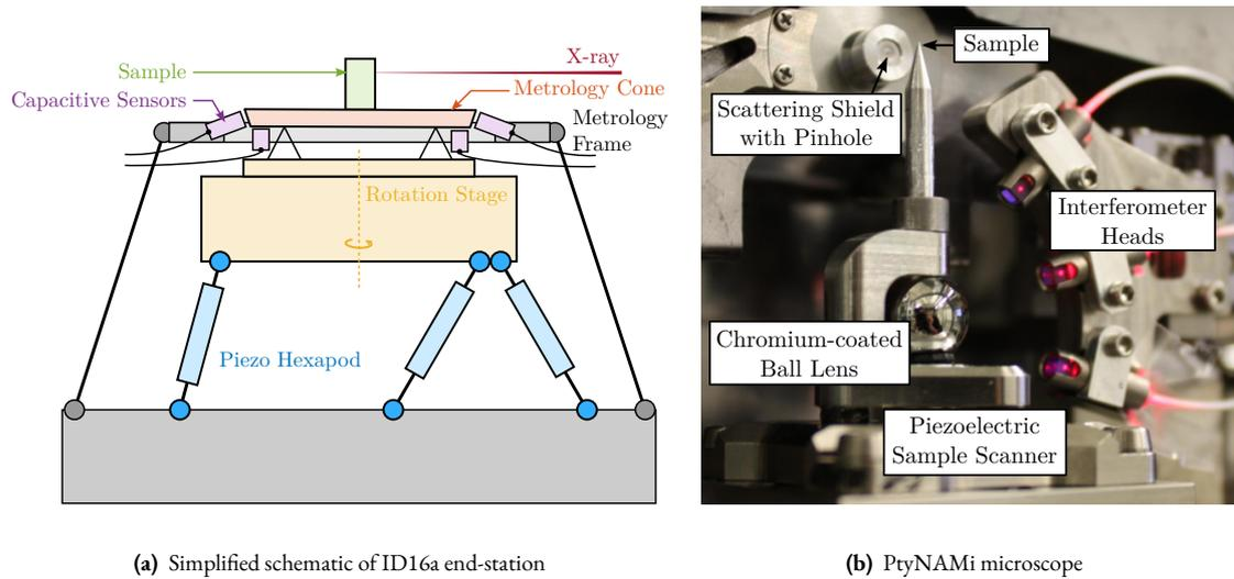
**Figure 2.101:** Example of two sample stages for tomography experiments. ID16a endstation [147] at the ESRF (a). PtyNAMi microscope [124, 125] at PETRA III (b)
