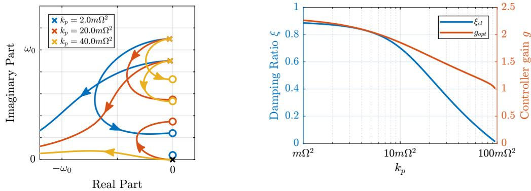
(a) Root Locus: Effect of parallel stiffness on the attainable damping,  $\Omega = 0.1\omega_0$  (b) Attainable damping ratio  $\xi_{cl}$  as a function of the parallel stiffness  $k_p$ . The corresponding control gain  $g_{opt}$  is also shown. Values for  $k_p < m\Omega^2$  are not shown because the system is unstable.
