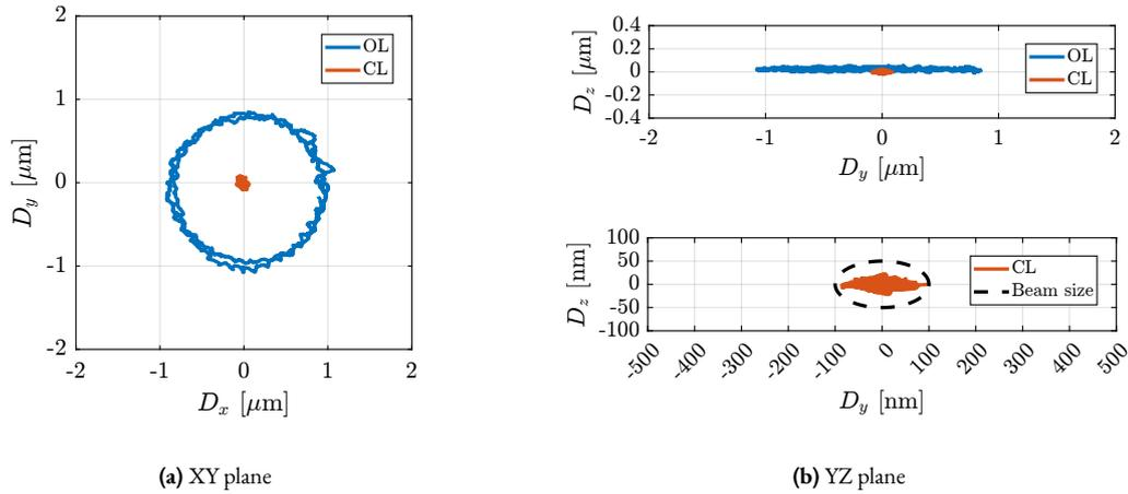
**Figure 2.134:** Position error of the sample in the XY (a) and YZ (b) planes during a simulation of a tomography experiment at 360 deg/s. 1kg payload is placed on top of the nano-hexapod.
