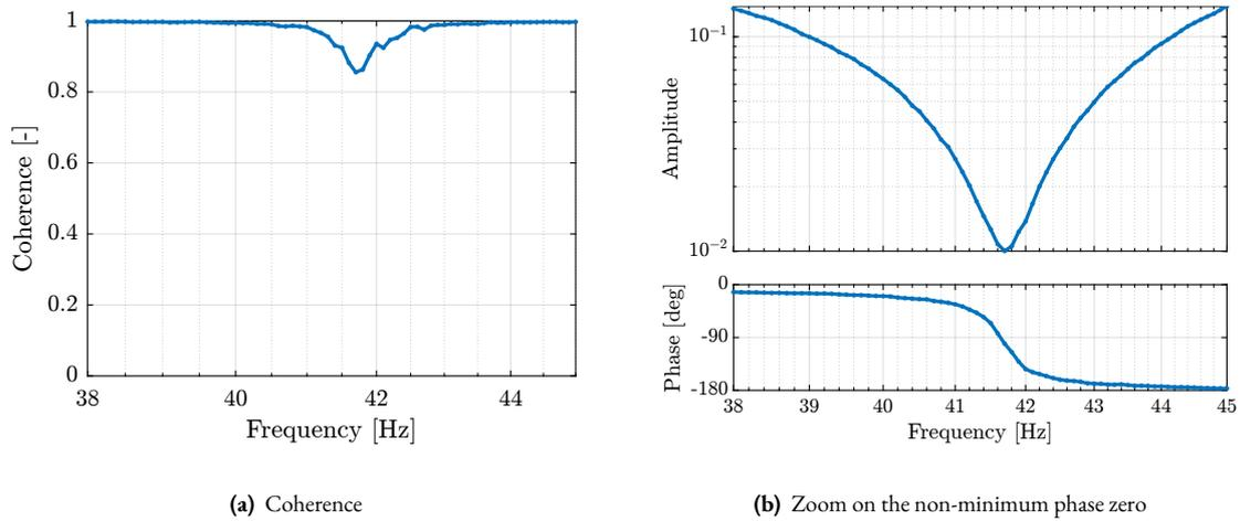
**Figure 4.15:** Measurement of the anti-resonance found in the transfer function from  $u$  to  $V_s$ . The coherence (a) is quite good around the anti-resonance frequency. The phase (b) shows a non-minimum phase behavior.
