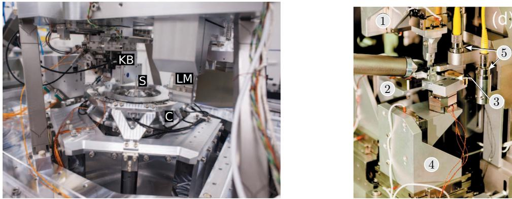
(a) ESRF ID16a - HPZ. KB is the focusing optics, S the sample, C the capacitive sensors and LM is the light microscope [147] (b) NSLS-II HXN - Microscope. 1 and 2 are focusing optics, 3 is the sample location, 4 the sample stage and 5 the interferometers [102]
