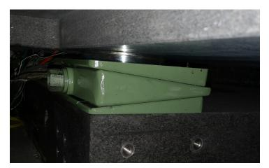
Figure 2.74: AirLoc used for the granite (2120-KSKC)
