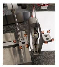
Figure 4.3: Measurement setup for flatness estimation
