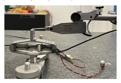
Figure 4.5: Bench to measure the APA stroke
