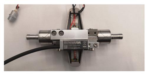
Figure 4.38: One strut including two flexible joints, an amplified piezoelectric actuator and an encoder
