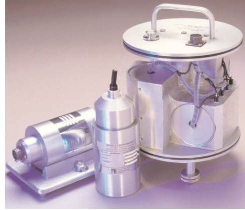
Figure 2.90: (3D) L-4C geophone.
