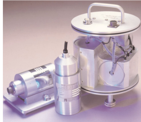
Figure 2.90: (3D) L-4C geophone
