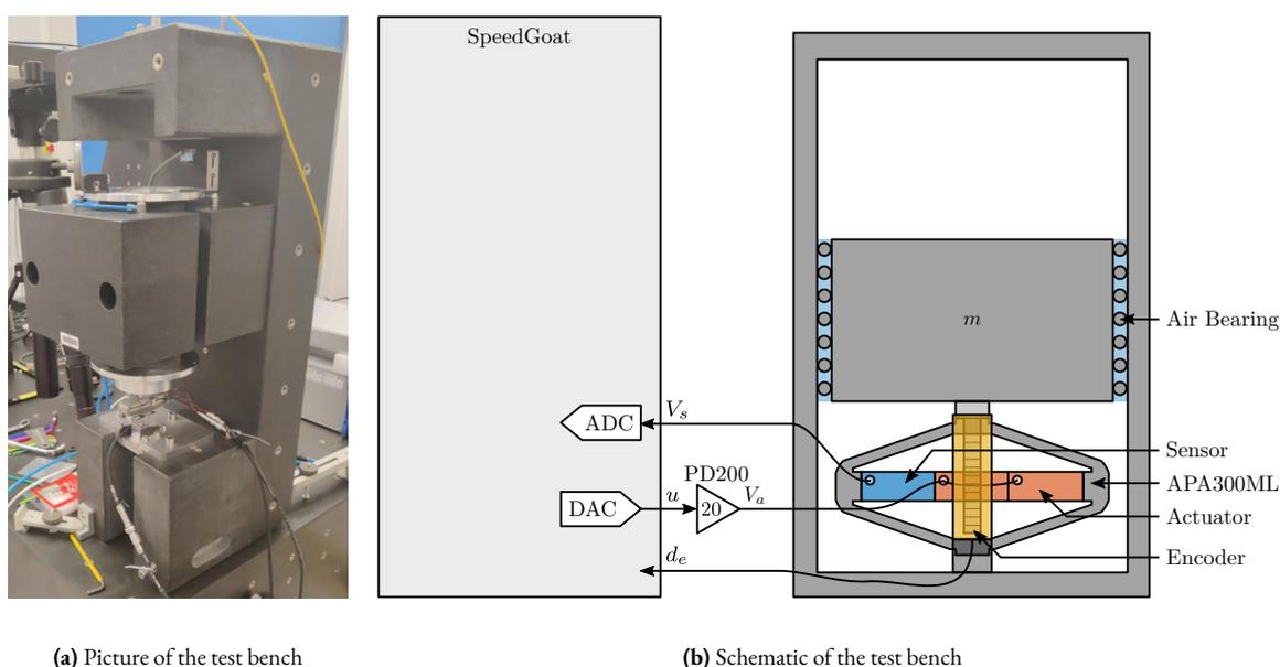
**Figure 4.10:** Test bench used to measure the dynamics of the APA300ML.  $u$  is the output DAC voltage,  $V_a$  the output amplifier voltage (i.e. voltage applied across the actuator stacks),  $d_e$  the measured displacement by the encoder and  $V_s$  the measured voltage across the sensor stack.
