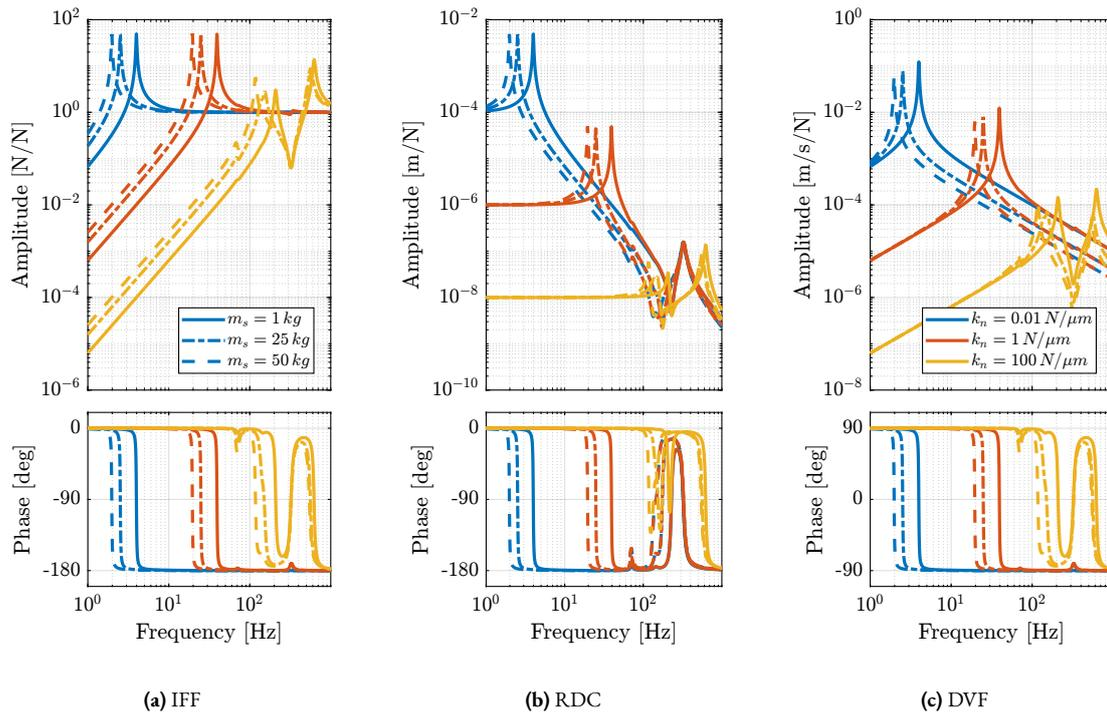
**Figure 2.16:** Plant dynamics for the three active damping techniques: IFF (a), RDC (b) and DVF (c). Three active platform stiffnesses ( $k_n = 0.01\text{ N}/\mu\text{m}$  in blue,  $k_n = 1\text{ N}/\mu\text{m}$  in red and  $k_n = 100\text{ N}/\mu\text{m}$  in yellow) and three sample's masses ( $m_s = 1\text{ kg}$ : solid curves,  $m_s = 25\text{ kg}$ : dot-dashed curves, and  $m_s = 50\text{ kg}$ : dashed curves) are considered in each case.
