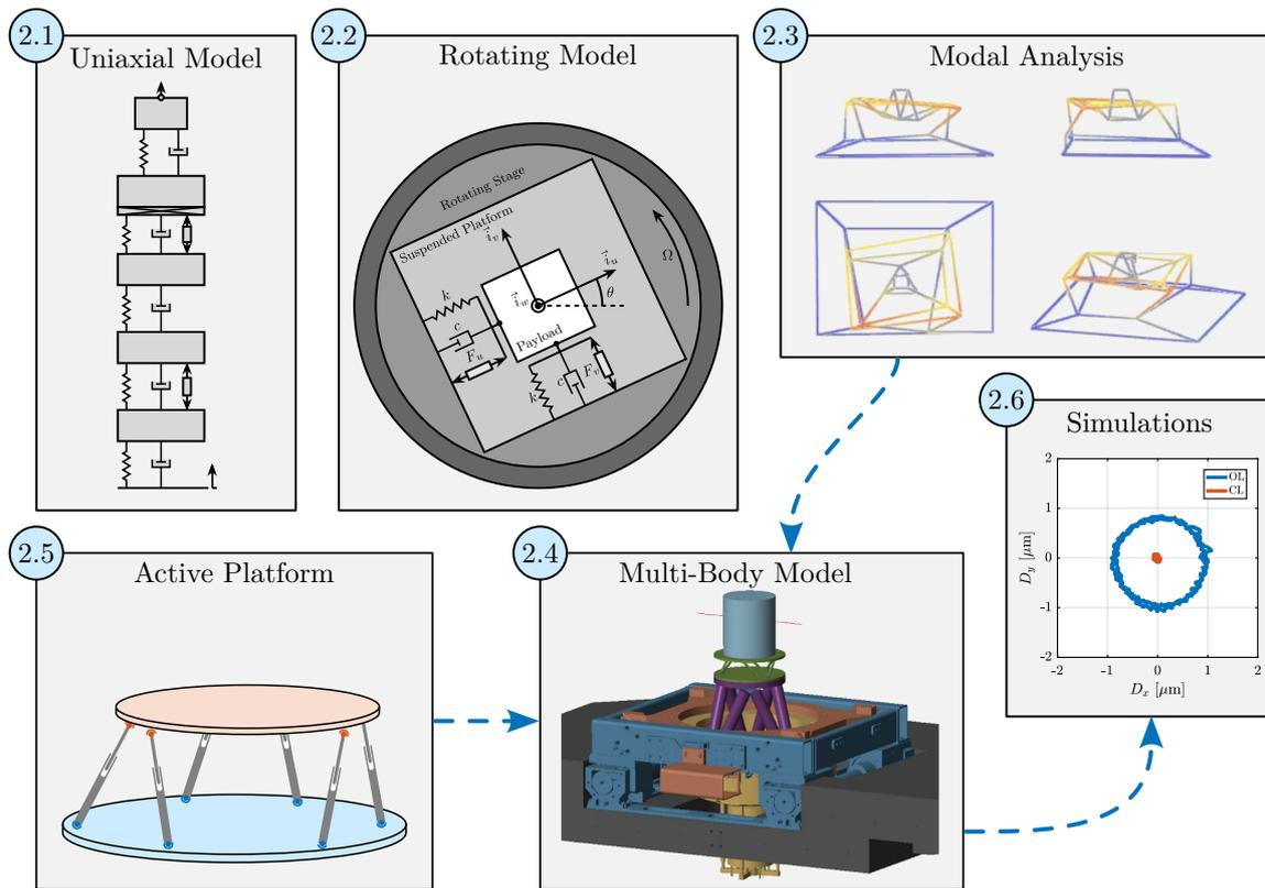
**Figure 2.1:** Overview of the conceptual design development. The approach evolves from simplified analytical models to a multi-body model tuned from experimental modal analysis. Closed-loop simulations of tomography experiments are used to validate the concept.
