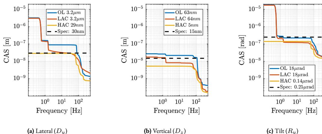
**Figure 4.104:** Cumulative Amplitude Spectrum for tomography experiments at 180 deg/s. Open-Loop case, IFF, and HAC-LAC are compared. Specifications are indicated by black dashed lines. The RMS values are indicated in the legend.
