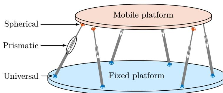
**Figure 2.104:** Schematic representation of the Stewart platform architecture.
