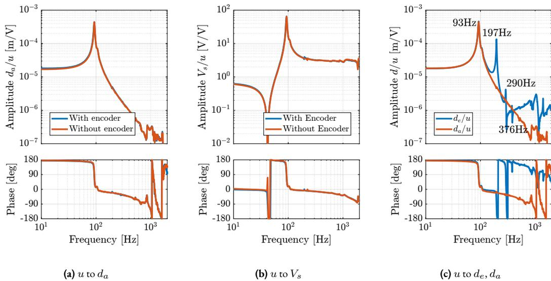
**Figure 4.46:** Effect of having the encoder fixed to the struts on the measured dynamics from  $u$  to  $d_a$  (a) and from  $u$  to  $V_s$  (b). Comparison of the observed dynamics by the encoder and interferometers (c).
