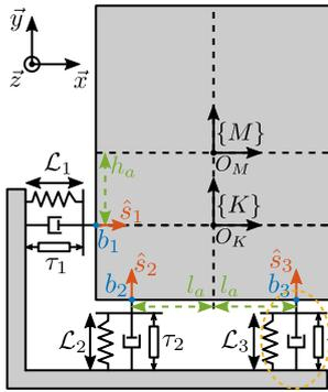
Figure 3.54: Model used to compare decoupling strategies.
