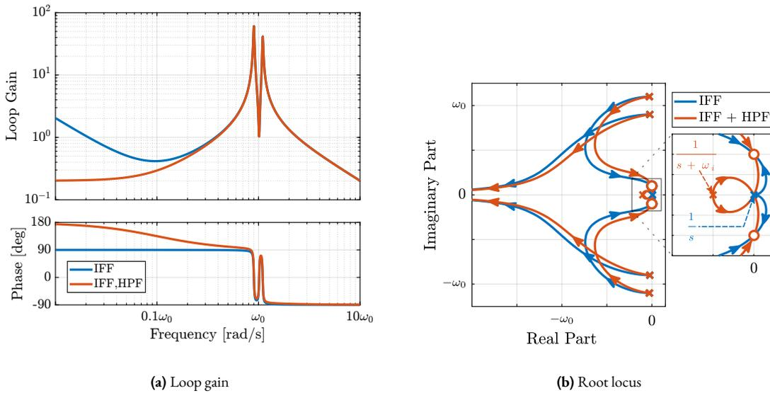
**Figure 2.42:** Comparison of the IFF with pure integrator and modified IFF with added high-pass filter ( $\Omega = 0.1\omega_0$ ). The loop gain is shown in (a) with  $\omega_i = 0.1\omega_0$  and  $g = 2$ . The root locus is shown in (b).
