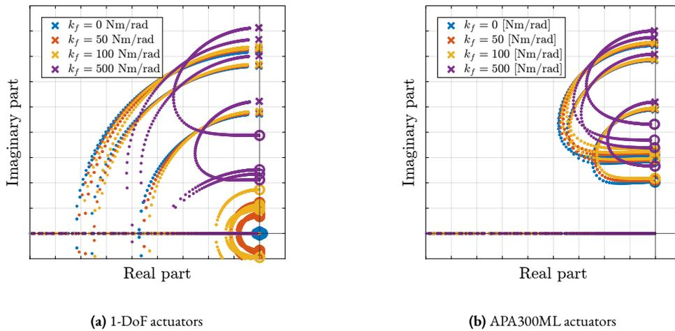
**Figure 3.37:** Effect of bending stiffness of the flexible joints on the attainable damping with decentralized IFF. For 1-DoF actuators (a), and with the 2-DoF model of the APA300ML (b).
