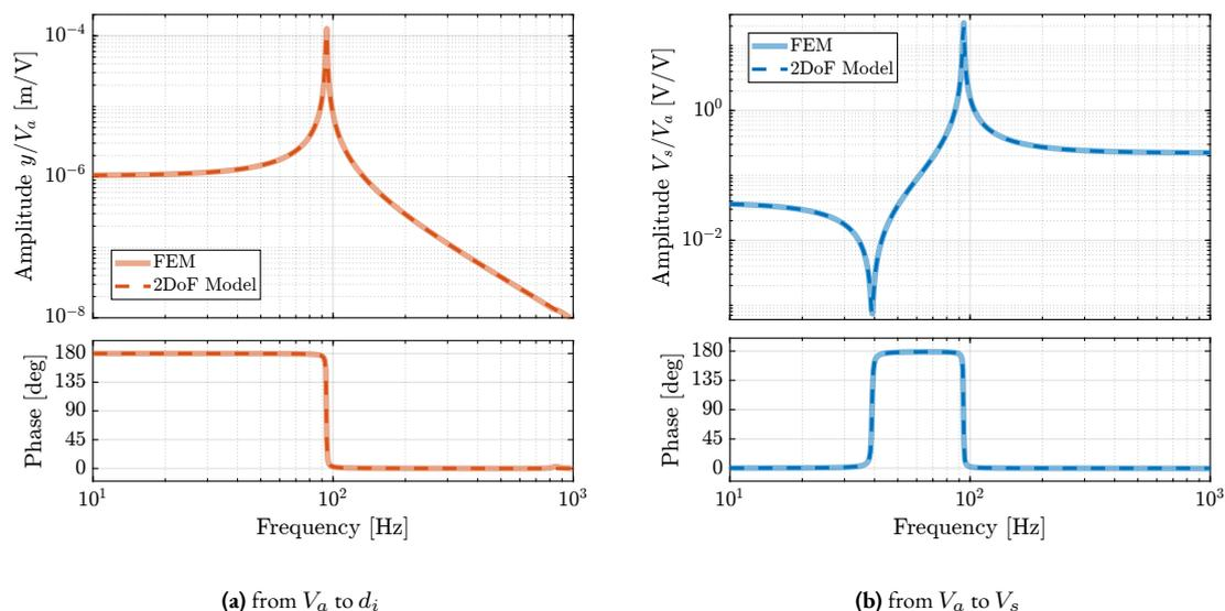
**Figure 3.32:** Comparison of the transfer functions extracted from the finite element model of the APA300ML and of the 2-DoF model. Both for the dynamics from  $V_a$  to  $d_i$  (a) and from  $V_a$  to  $V_s$  (b).
