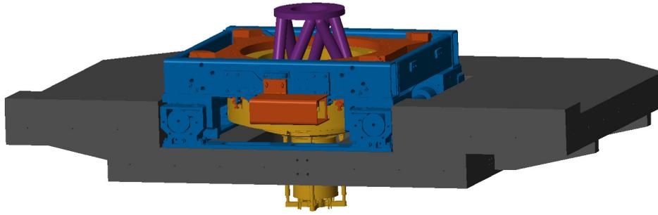
**Figure 2.85:** 3D view of the micro-station multi-body model.
