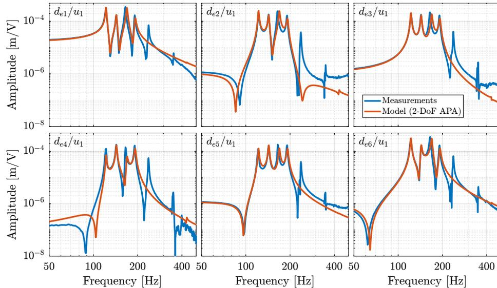
**Figure 4.71:** Comparison of the measured (in blue) and modelled (in red) FRFs from the first control signal  $u_1$  to the six encoders  $d_{e1}$  to  $d_{e6}$ . The APA are here modelled with a 2-DoF mass-spring-damper system. No payload is used.
