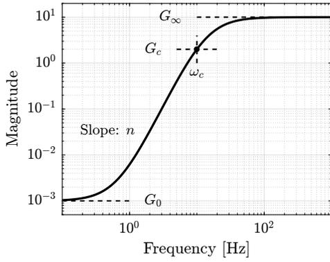
$$W(s) = \left( \frac{\frac{1}{\omega_c} \sqrt{\frac{1 - \left(\frac{G_0}{G_c}\right)^{\frac{2}{n}}}{1 - \left(\frac{G_c}{G_\infty}\right)^{\frac{2}{n}}}} s + \left(\frac{G_0}{G_c}\right)^{\frac{1}{n}}}{\frac{1}{G_\infty^{\frac{1}{n}}} \frac{1}{\omega_c} \sqrt{\frac{1 - \left(\frac{G_0}{G_c}\right)^{\frac{2}{n}}}{1 - \left(\frac{G_c}{G_\infty}\right)^{\frac{2}{n}}}} s + \frac{1}{G_c^{\frac{1}{n}}}} \right)^n \quad (3.33)$$
