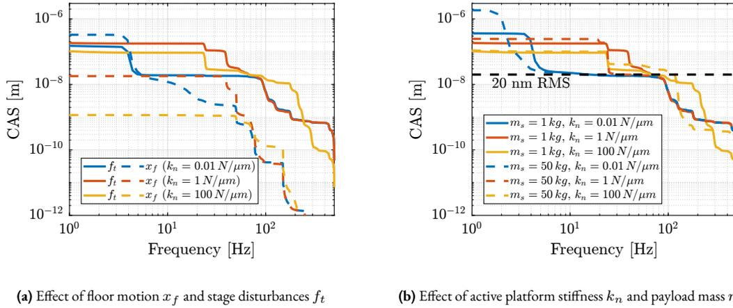
**Figure 2.11:** Cumulative Amplitude Spectrum of the relative motion  $d$ . The effect of  $x_f$  and  $f_t$  are shown in (a). The effect of sample mass for the three active platform stiffnesses is shown in (b). The control objective of having a residual error of 20 nm RMS is shown by the horizontal black dashed line.
