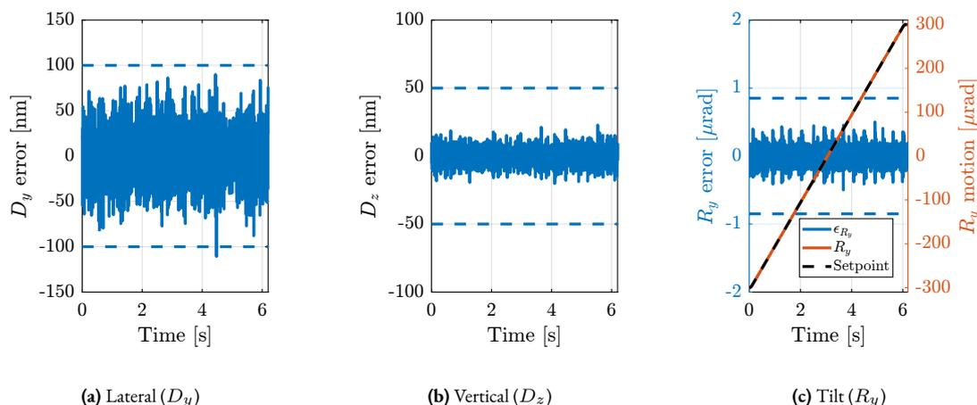
**Figure 4.105:** Reflectivity scan ( $R_y$ ) with a rotational velocity of 100  $\mu$ rad/s.
