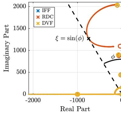
**Figure 2.18:** Root locus for the three damping techniques applied with the soft active platform. It is shown that the RDC active damping technique has some authority on one mode of the micro-station. This mode corresponds to the suspension mode of the positioning hexapod.
