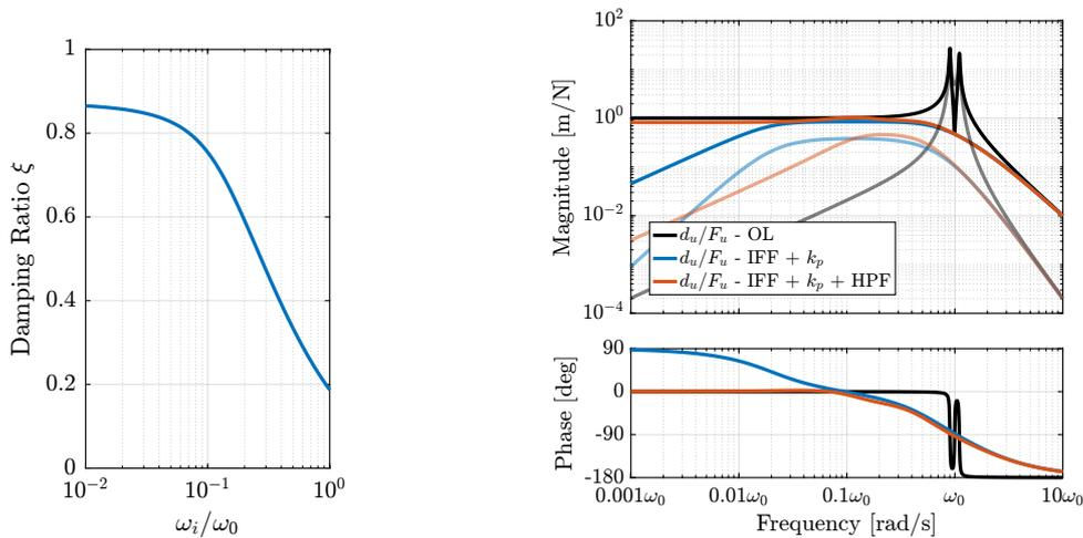
**Figure 2.48:** Effect of high-pass filter cut-off frequency on the obtained damping (a) and on the damped plant (b).
