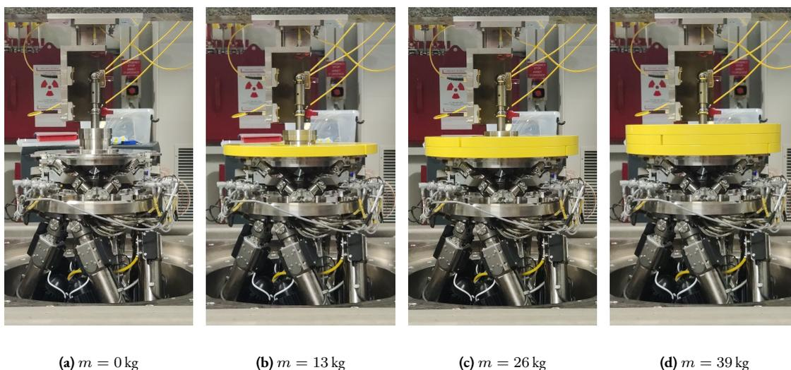
Figure 4.86: Four tested payload conditions: (a) no payload, (b) 13 kg payload, (c) 26 kg payload, (d) 39 kg payload.
