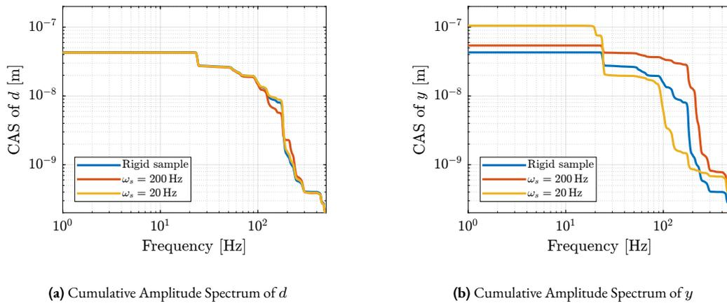
**Figure 2.36:** Cumulative Amplitude Spectrum of the distances  $d$  and  $y$ . The effect of the sample's flexibility does not affect much  $d$  but is detrimental to the stability of  $y$ . A sample mass  $m_s = 1$  kg and an active platform stiffness of  $100$  N/ $\mu$ m are used for the simulations.
