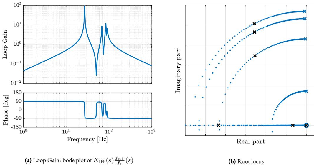
(a) Loop Gain: bode plot of  $K_{\text{IFF}}(s) \frac{f_{n1}}{f_1}(s)$
