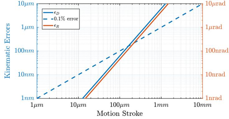
**Figure 2.107:** Errors associated with the use of the Jacobian matrix to solve the forward kinematic problem. A Stewart platform with a height of 100 mm was used to perform this analysis.  $\epsilon_D$  corresponds to the distance between the true position and the estimated position.  $\epsilon_R$  corresponds to the angular motion between the true orientation and the estimated orientation.
