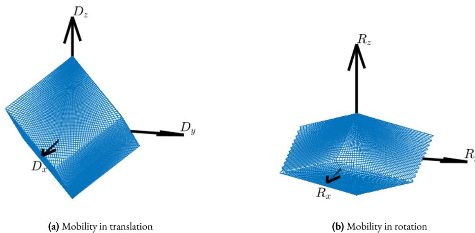
**Figure 3.9:** Mobility of a Stewart platform with Cubic architecture. Both for translations (a) and rotations (b).
