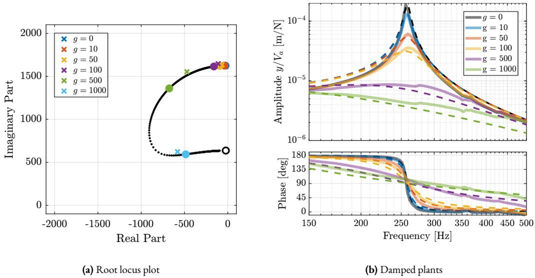
**Figure 3.28:** Results using Integral Force Feedback with the APA95ML. Closed-loop poles as a function of the controller gain  $g$  are predicted by the root locus plot (a). Circles are predictions from the model while crosses are poles estimated from the experimental data. Damped plants estimated from the model (dashed curves) and measured ones (solid curves) are compared in (b) for all tested controller gains.
