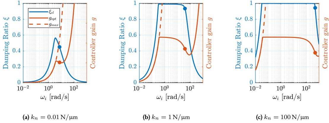
**Figure 2.54:** For each value of  $\omega_i$ , the maximum damping ratio  $\xi$  is computed (blue), and the corresponding controller gain is shown (in red). The chosen controller parameters used for further analysis are indicated by the large dots.
