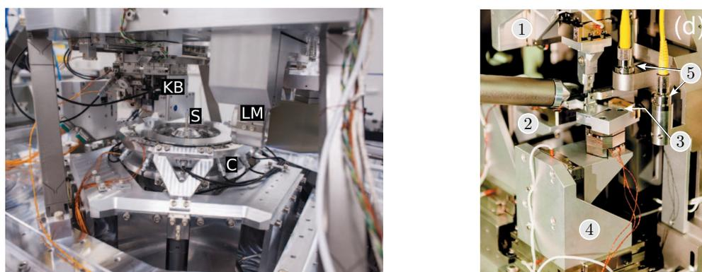
**(a)** ESRF ID16a - HPZ. KB is the focusing optics, S the sample, C the capacitive sensors and LM is the light microscope [152] **(b)** NSLS-II HXN. 1 and 2 are focusing optics, 3 is the sample location, 4 the sample stage and 5 the interferometers [107]
