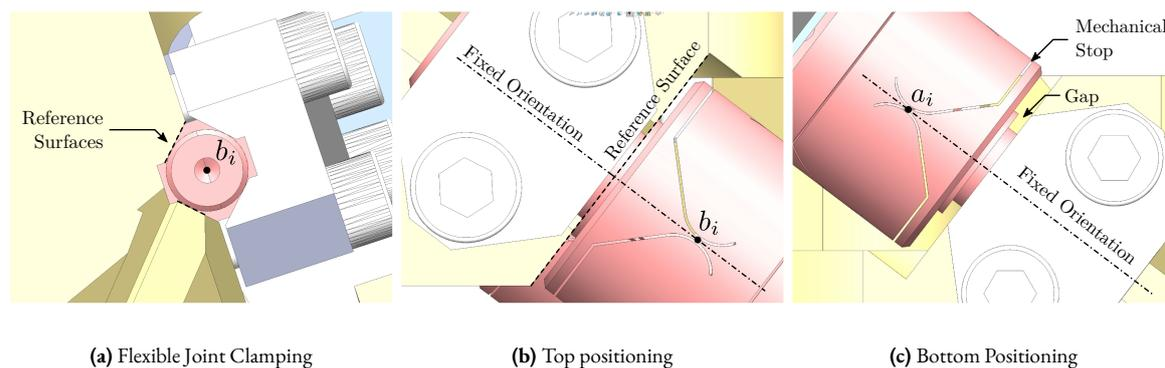
**Figure 3.96:** Clamping of the flexible points on the nano-hexapod plates. Both top and bottom flexible joints are clamped to the plates as shown in (a). While the top flexible joints are in contact with the top plate for precise positioning of its center of rotation (b), the bottom joints are just oriented (c).
