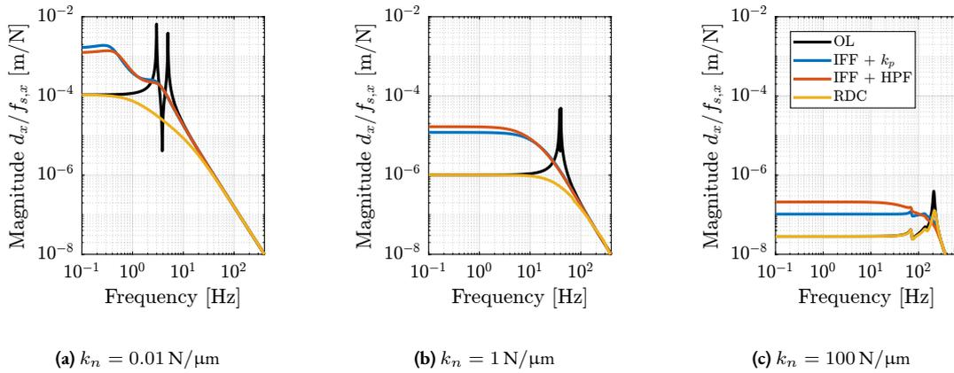
**Figure 2.62:** Effect of sample forces  $f_{s,x}$  on the position error  $d_x$  - Comparison of active damping techniques for the three active platform stiffnesses. Integral Force Feedback degrades this compliance at low-frequency.
