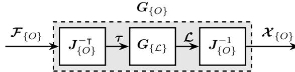
**Figure 3.56:** Block diagram of the decoupling the plant in a frame  $\{O\}$  using Jacobian matrix  $\mathbf{J}_{\{O\}}$
