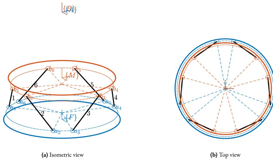
**Figure 3.21:** Obtained architecture for the active platform.
