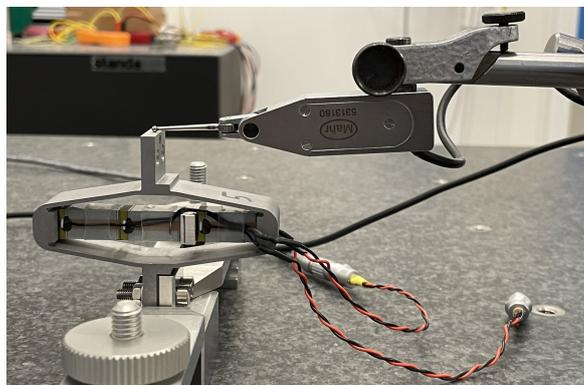
Figure 4.5: Test bench to measure the APA stroke.
