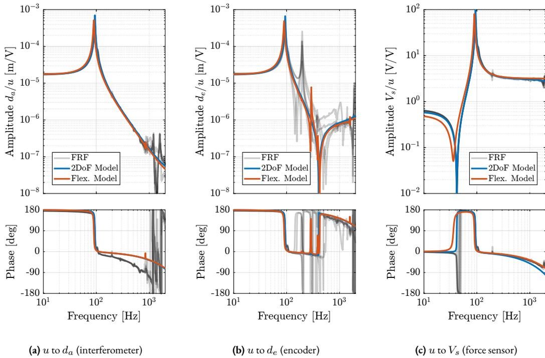
**Figure 4.49:** Comparison of the measured dynamics of the struts (black) with dynamics extracted from the multi-body model using the 2-DoF APA model (blue), and using the reduced order flexible model of the APA300ML model (red).
