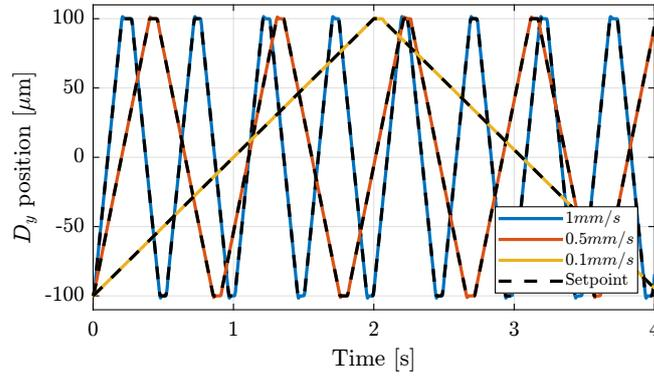
Figure 4.111: Lateral ( $D_y$ ) motion for several configured velocities.
