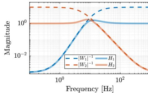
**Figure 3.51:** Weights and obtained filters.
