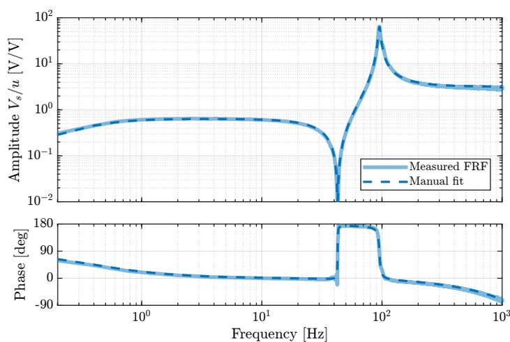
**Figure 4.15:** Identified IFF plant and manually tuned model of the plant (a time delay of  $200 \mu\text{s}$  is added to the model of the plant to better match the identified phase). Note that a minimum-phase zero is identified here even though the coherence is not good around the frequency of the zero.
