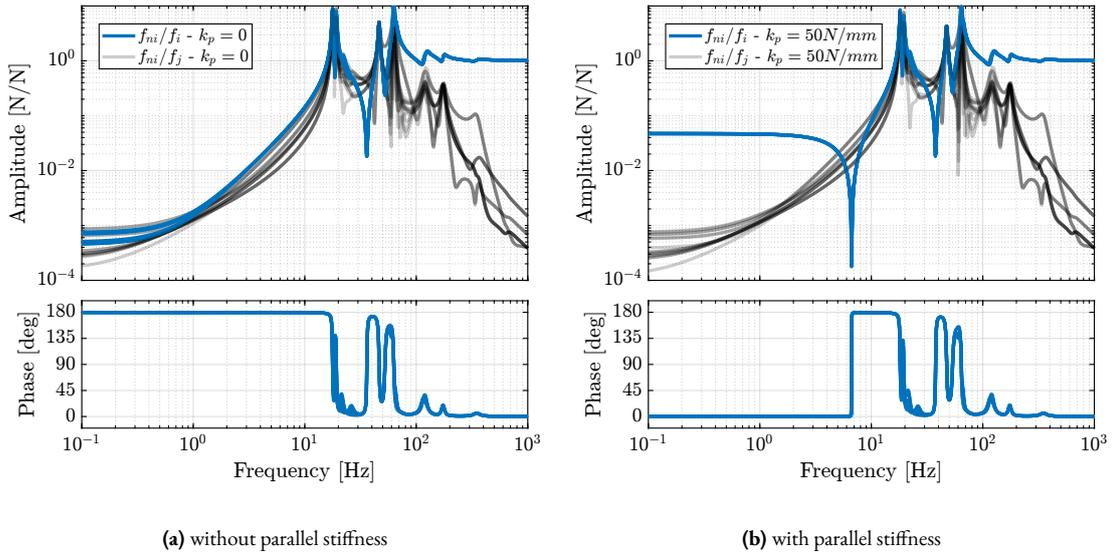
**Figure 2.125:** Effect of stiffness in parallel with the force sensor on the IFF plant with  $\Omega_z = 360$  deg/s and a payload mass of 25 kg. The dynamics without parallel stiffness has non-minimum phase zeros at low frequency (a). The added parallel stiffness transforms the non-minimum phase zeros into complex conjugate zeros (b).
