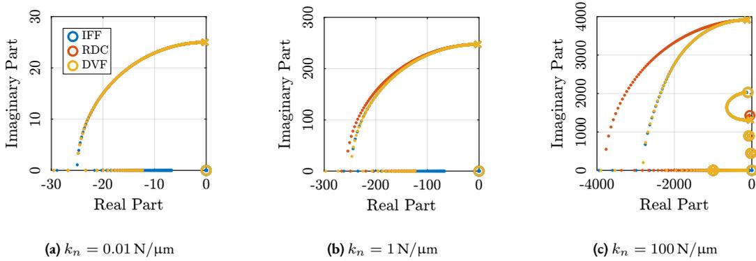
**Figure 2.17:** Root loci for the three active damping techniques (IFF in blue, RDC in red and DVF in yellow). This is shown for the three active platform stiffnesses. The root loci are zoomed on the suspension mode of the active platform.
