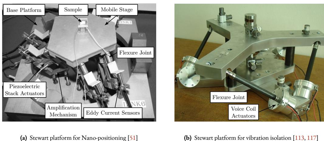
**Figure 2.103:** Two examples of Stewart platforms. (a) Stewart platform based on piezoelectric actuators and used for nano-positioning. (b) Stewart platform based on voice coil actuators and used for vibration isolation.
