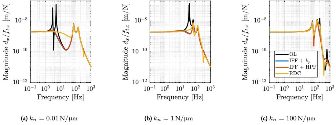
**Figure 2.61:** Effect of micro-station vibrations  $f_{t,x}$  on the position error  $d_x$  - Comparison of active damping techniques for the three active platform stiffnesses. Relative Damping Control increases the sensitivity to micro-station vibrations between the soft active platform suspension modes and the micro-station modes (a).
