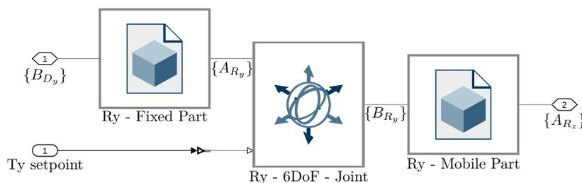
**Figure 2.84:** Example of a stage (here the tilt-stage) represented in the multi-body model software (Simulink - Simscape). It is composed of two solid bodies connected by a 6-DoF joint. One joint degree of freedom (here the tilt angle) can be “controlled”, the other degrees of freedom are represented by springs and dampers. Additional disturbing forces for all degrees of freedom can be included.
