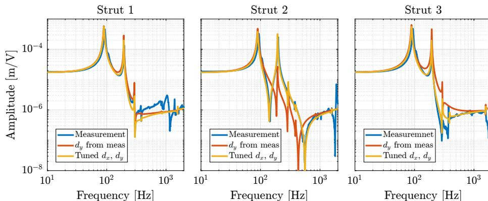
**Figure 4.52:** Comparison of the frequency response functions from DAC voltage  $u$  to measure displacement  $d_e$  by the encoders for three struts. The measured dynamics is shown in blue, the dynamics extracted from the model with the  $y$  misalignment estimated from measurements is shown in red, and the dynamics extracted from the model when both the  $x$  and  $y$  misalignments are tuned is shown in yellow.
