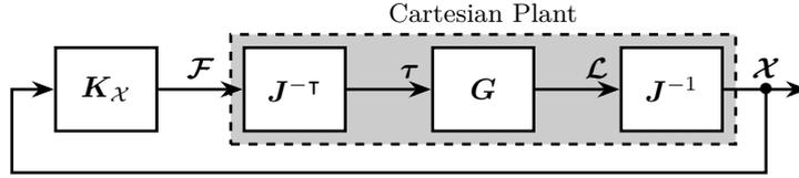
Figure 3.10: Typical control architecture in the cartesian frame.
