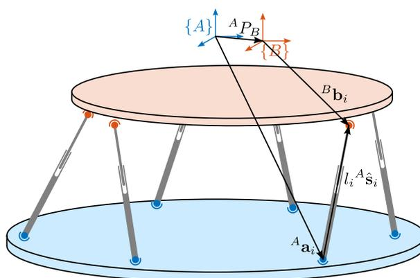
**Figure 2.106:** Geometrical representation of the loop closure.
