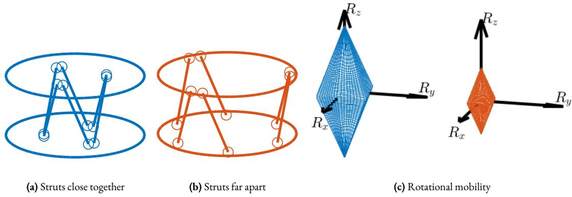
**Figure 3.6:** Effect of strut position on the obtained mobility in rotation. Two Stewart platform geometries are considered: struts close to each other (a) and struts further apart (b). Obtained mobility for both geometry are shown in (c).
