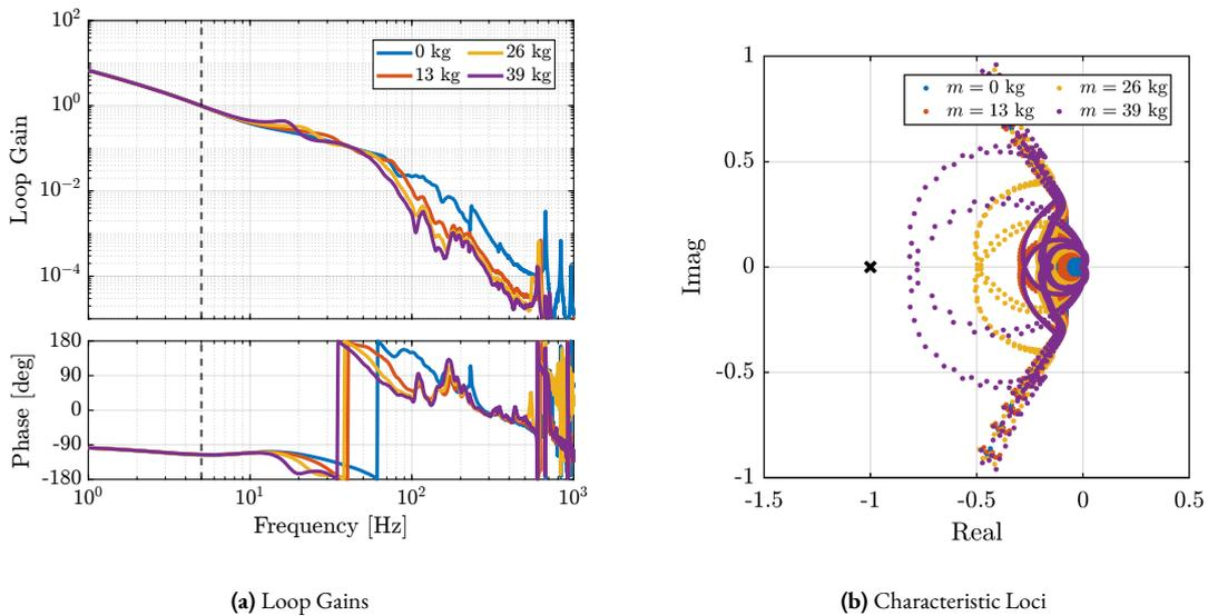
**Figure 4.98:** “Decentralized loop-gains” (a) and characteristic loci (b) for the robust high authority controller.
