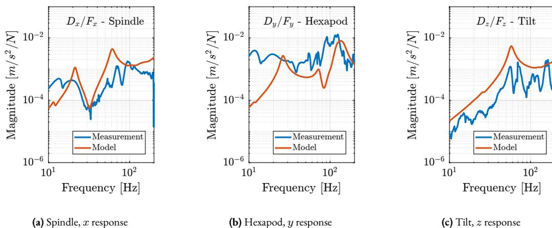
**Figure 2.86:** FRFs from a hammer impact to the stage acceleration, both expressed at its CoM. The measured FRFs are compared with the multi-body model. Different directions are computed for different stages.
