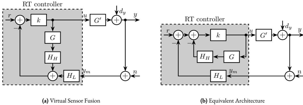
**Figure 3.64:** Control architecture for virtual sensor fusion (a) and equivalent architecture (b). Signals are the reference input  $r$ , the output perturbation  $d_y$ , the measurement noise  $n$  and the control input  $u$ .
