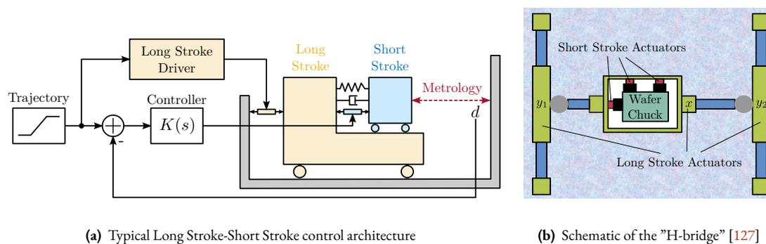
**Figure 1.15:** Schematic of a typical Long stroke-Short stroke control architecture (a). A 3-DoF long stroke-short stroke is shown in (b) where  $y_1$ ,  $y_2$  and  $x$  are 3-phase linear motors and short stroke actuators are voice coils.
