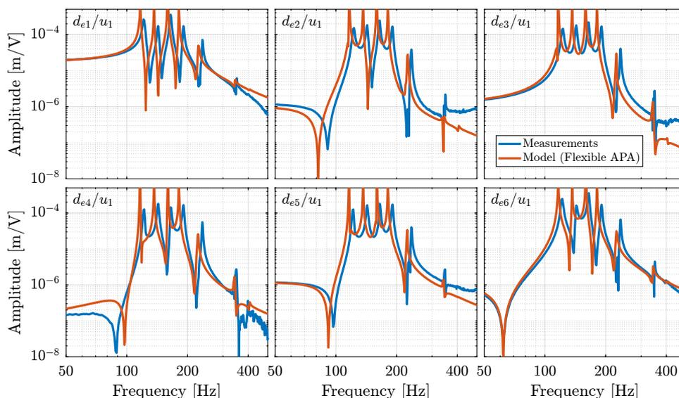
**Figure 4.72:** Comparison of the measured (in blue) and modelled (in red) FRFs from the first control signal  $u_1$  to the six encoders  $d_{e1}$  to  $d_{e6}$ . The APA are here modelled with a “super-element”. No payload was used.
