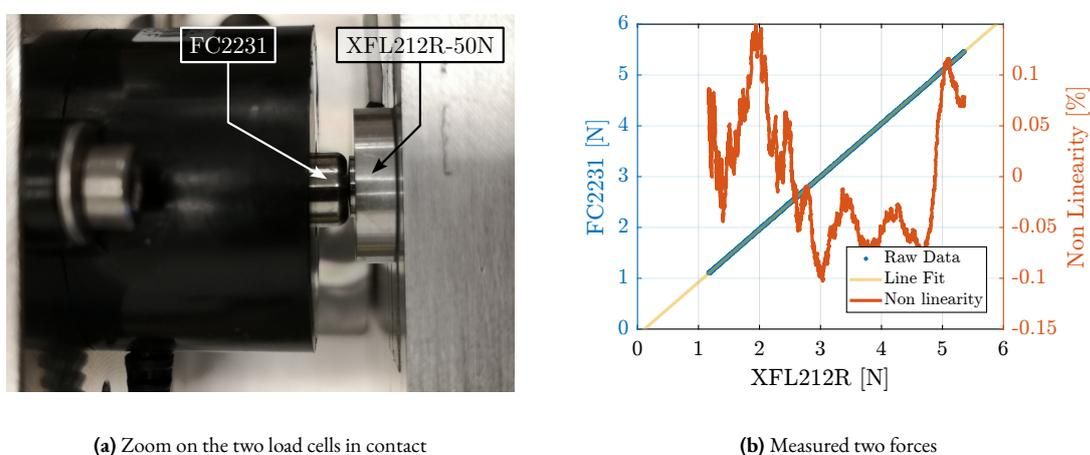
**Figure 4.32:** Estimation of the load cell accuracy by comparing the measured force of two load cells. A picture of the measurement bench is shown in (a). Comparison of the two measured forces and estimated non-linearity are shown in (b).
