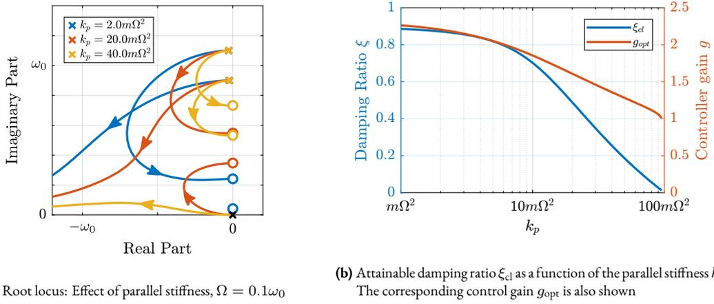
**Figure 2.47:** Effect of the parallel stiffness on the achievable damping with IFF.
