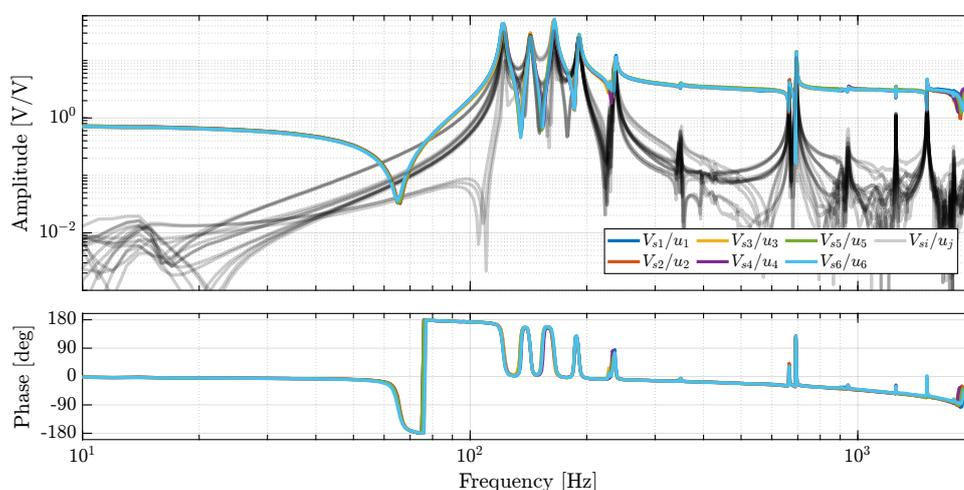
**Figure 4.66:** Measured FRF from  $u$  to  $V_s$ . The 6 direct terms are the colored lines, and the 30 coupling terms are the gray lines.
