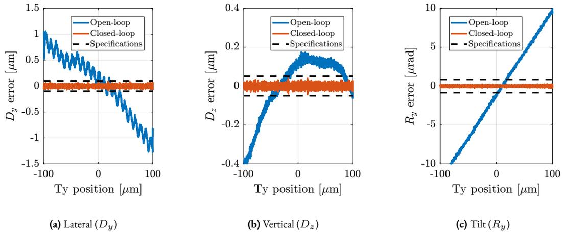
**Figure 4.109:** Open-loop (in blue) and closed-loop (i.e. using the NASS, in red) during a 10  $\mu\text{m}/\text{s}$  scan with the  $T_y$  stage.
