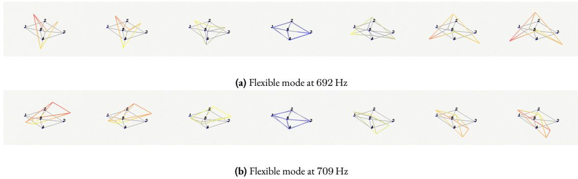
**Figure 4.64:** Two identified flexible modes of the top plate of the Nano-Hexapod.
