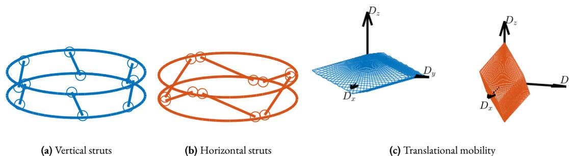
**Figure 3.5:** Effect of strut orientation on the obtained mobility in translation. Two Stewart platform geometries are considered: struts oriented vertically (a) and struts oriented horizontally (b). Obtained mobility for both geometry are shown in (c).
