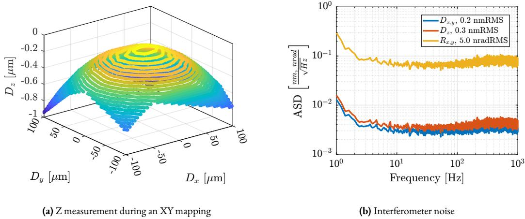
**Figure 4.81:** Estimated measurement errors of the metrology. Cross-coupling between lateral motion and vertical measurement is shown in (a). The effect of interferometer noise on the measured translations and rotations is shown in (b).
