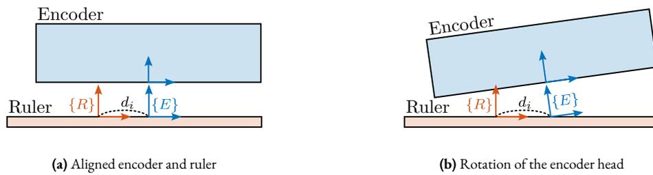
**Figure 3.101:** Representation of the encoder multi-body model. Measurement  $d_i$  corresponds to the  $x$  position of the encoder frame  $\{E\}$  expressed in the ruler frame  $\{R\}$  (a). A rotation of the encoder therefore induces a measured displacement (b).
