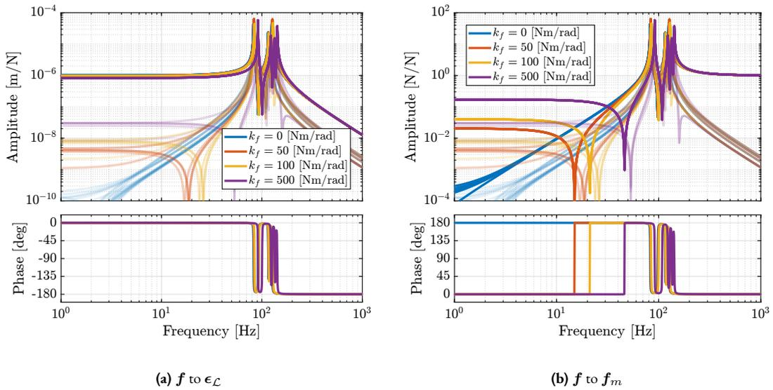
**Figure 3.36:** Effect of bending stiffness of the flexible joints on the plant dynamics. Both from actuator force  $f$  to strut motion measured by external metrology  $\epsilon_L$  (a) and to the force sensors  $f_m$  (b).
