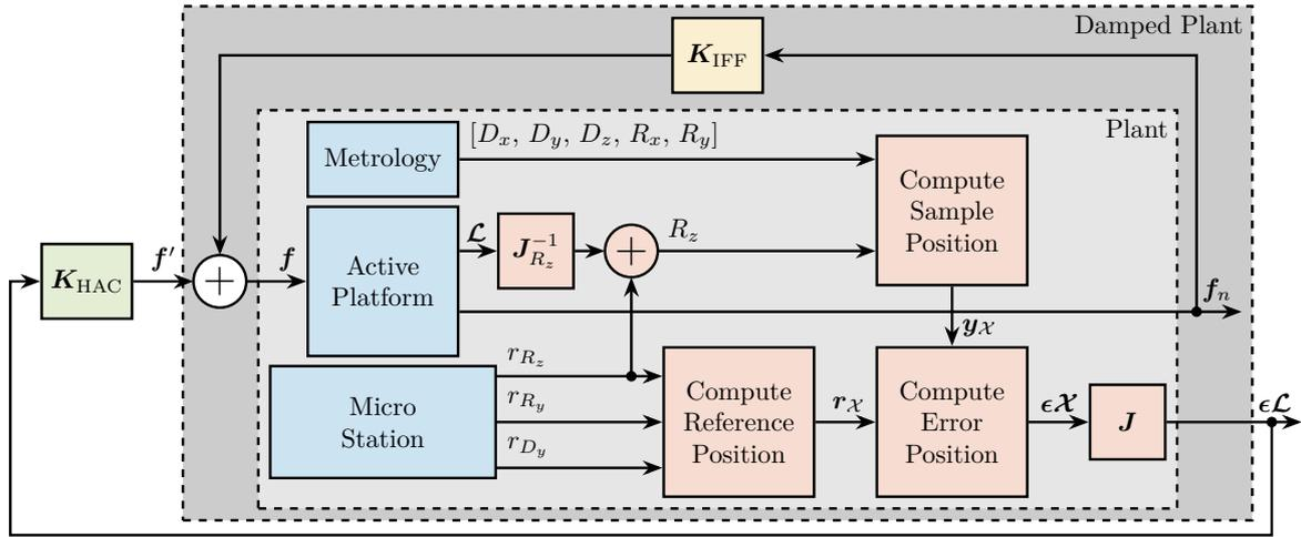
**Figure 2.124:** Control architecture for the NASS. Physical systems are shown in blue, control kinematics elements in red, decentralized Integral Force Feedback controller in yellow, and centralized high authority controller in green.
