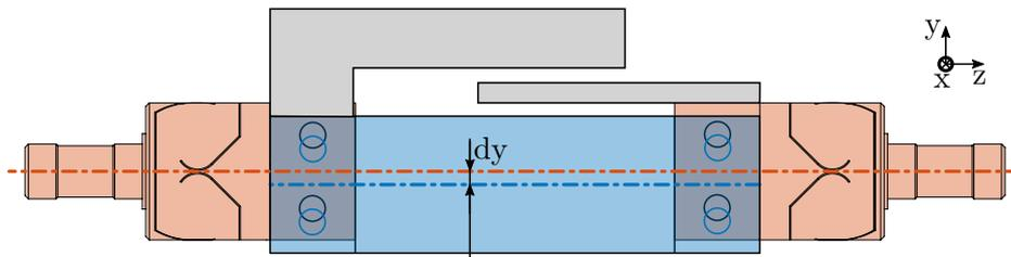
**Figure 4.50:** Misalignment between the joints and the APA.
