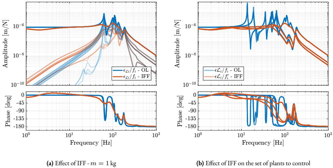
**Figure 2.130:** Effect of decentralized Integral Force Feedback on the positioning plant for a 1 kg sample mass (a). Direct terms are shown by solid lines while coupling terms are shown by shaded lines. The direct terms of the positioning plants for all considered payloads are shown in (b).
