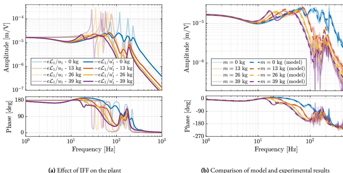
**Figure 4.93:** Comparison of the open-loop plant and the damped plant with decentralized IFF, estimated from the multi-body model (a). Comparison of measured damped and modelled plants for all considered payloads (b). Only “direct” terms ( $\epsilon\mathcal{L}_i/u_i$ ) are displayed for simplicity.
