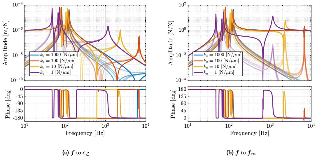
**Figure 3.38:** Effect of axial stiffness of the flexible joints on the plant dynamics. Both from actuator force  $\mathbf{f}$  to strut motion measured by external metrology  $\epsilon_{\mathcal{L}}$  (a) and to the force sensors  $\mathbf{f}_m$  (b).
