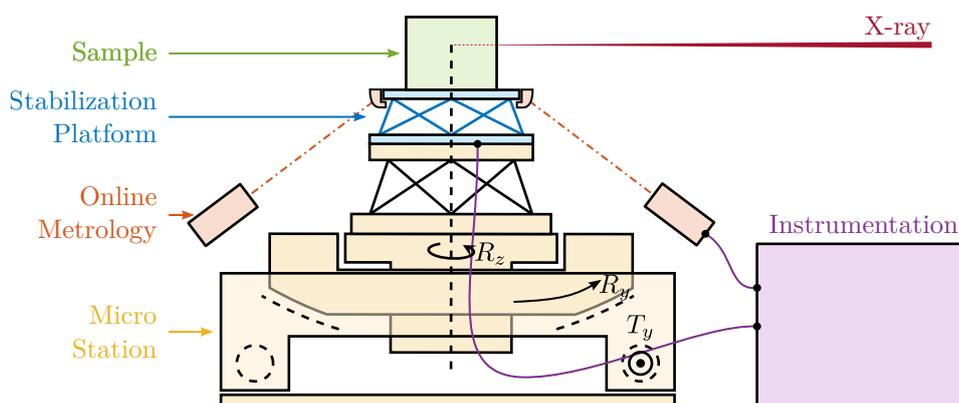
**Figure 1.16:** The Nano Active Stabilization System concept.
