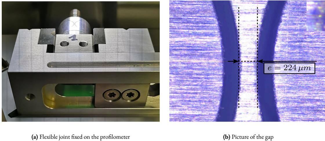
**Figure 4.26:** Setup to measure the dimensions of the flexible “neck” corresponding to the X-bending stiffness. The flexible joint is fixed to the profilometer (a) and an image is obtained with which the “neck” size can be estimated (b).
