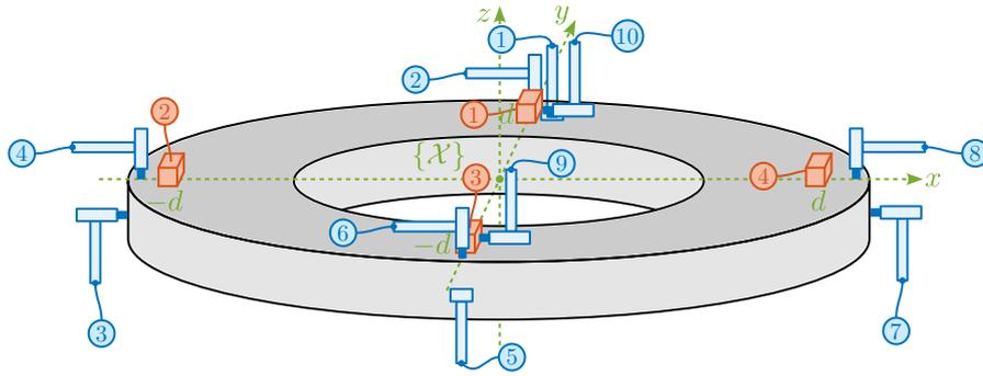
**Figure 2.87:** Schematic of the measurement setup used to estimate the compliance of the micro-station. Four 3-axis accelerometers (shown in red) are fix on top of the positioning hexapod platform. 10 hammer impacts are performed at different locations (shown in blue).
