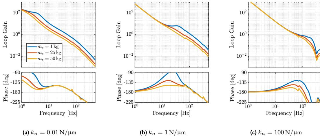
**Figure 2.25:** Loop gains for the High Authority Controllers.
