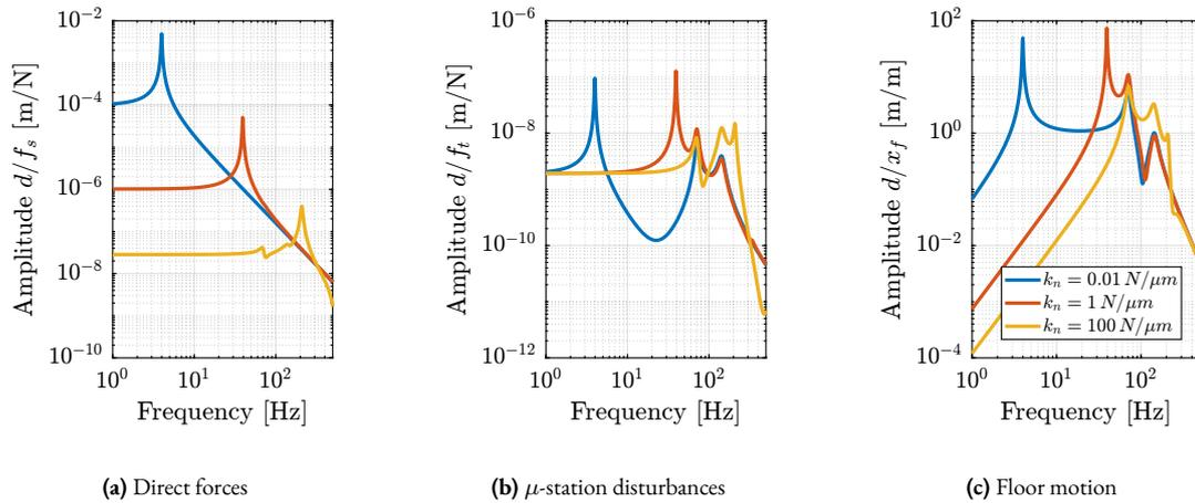
**Figure 2.10:** Sensitivity of  $d$  to disturbances for three different active platform stiffnesses.  $f_s$  the direct forces applied on the sample (a),  $f_t$  disturbances from the micro-station stages (b) and  $x_f$  the floor motion (c).
