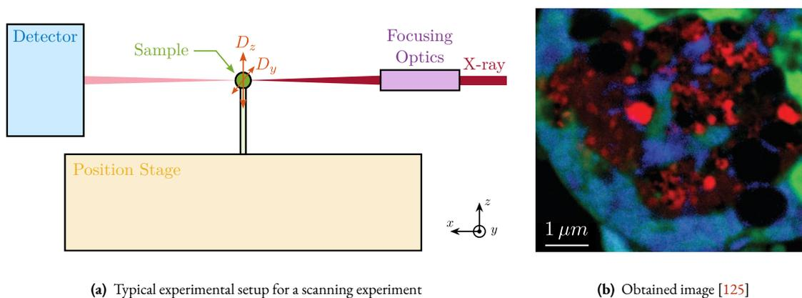
(a) Typical experimental setup for a scanning experiment
