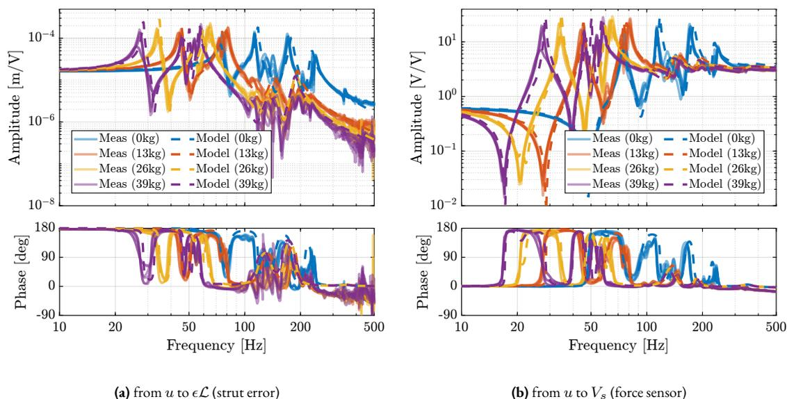
Figure 4.87: Comparison of the diagonal elements (i.e. “direct” terms) of the measured FRF matrix and the dynamics identified from the multi-body model. Both for the dynamics from  $u$  to  $\epsilon\mathcal{L}$  (a) and from  $u$  to  $V_s$  (b).
