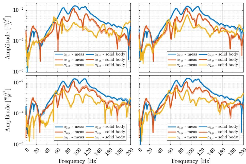
**Figure 2.71:** Comparison of the original accelerometer responses with responses reconstructed from the solid body response. Accelerometers 1 to 4, corresponding to the positioning hexapod, are shown. Input is a hammer force applied on the positioning hexapod in the  $x$  direction.
