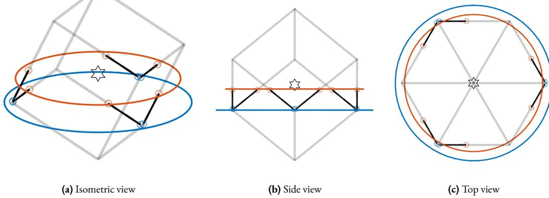
**Figure 3.20:** Cubic architecture with cube's center above the top platform. A cube height of 240 mm is used.
