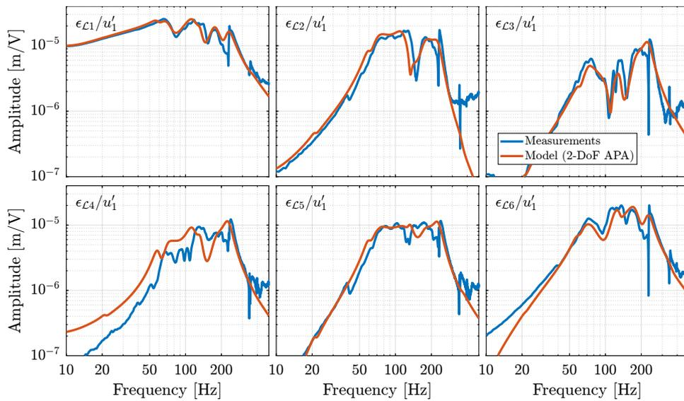
**Figure 4.95:** Comparison of the measured (in blue) and modelled (in red) FRFs from the first control signal ( $u'_1$ ) of the damped plant to the estimated errors ( $\epsilon_{\mathcal{L}_i}$ ) in the frame of the six struts by the external metrology.
