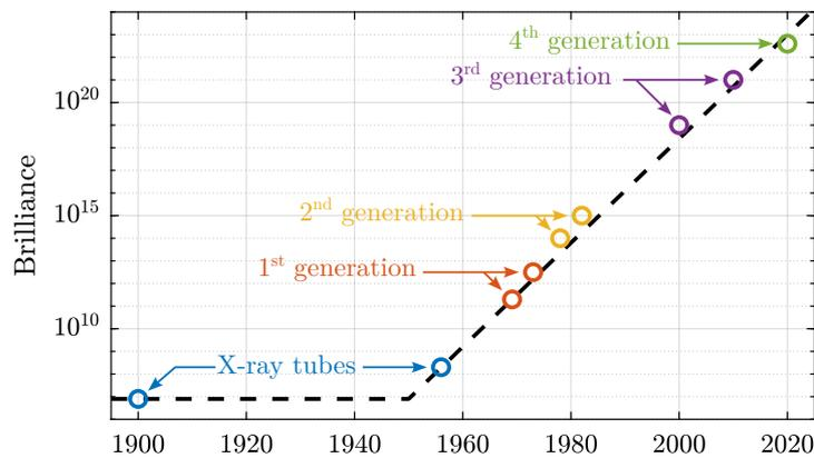
**Figure 1.3:** Evolution of the peak brilliance (expressed in photons/s/mm<sup>2</sup>/mrad<sup>2</sup>/0.1%BW) of synchrotron radiation facilities. Note the vertical logarithmic scale.
