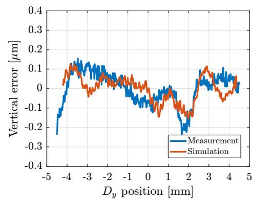
**Figure 2.99:** Vertical errors during a constant-velocity scan of the translation stage.
