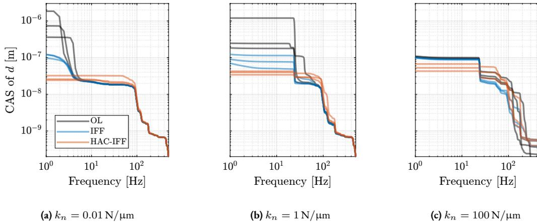
**Figure 2.27:** Cumulative Amplitude Spectra for all three active platform stiffnesses in OL, with IFF and with HAC-LAC. The three lines of each color are corresponding to the considered three sample masses.
