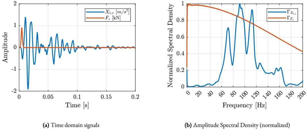
**Figure 2.68:** Raw measurement of the accelerometer 1 in the  $x$  direction (blue) and of the force sensor at the Hammer tip (red) for an impact in the  $z$  direction (a). Computed Amplitude Spectral Densities of the two signals (normalized) (b).
