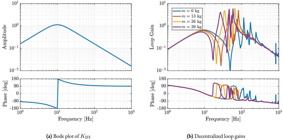
**Figure 4.91:** Bode plot of the decentralized IFF controller (a). The decentralized controller  $K_{\text{IFF}}$  multiplied by the identified dynamics from  $u_1$  to  $V_{s1}$  for all payloads are shown in (b).
