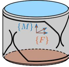
**Figure 3.41:** Defined frames for the reduced order flexible body. The two flat interfaces are considered rigid, and are linked to the two frames  $\{F\}$  and  $\{M\}$  both located at the center of rotation.
