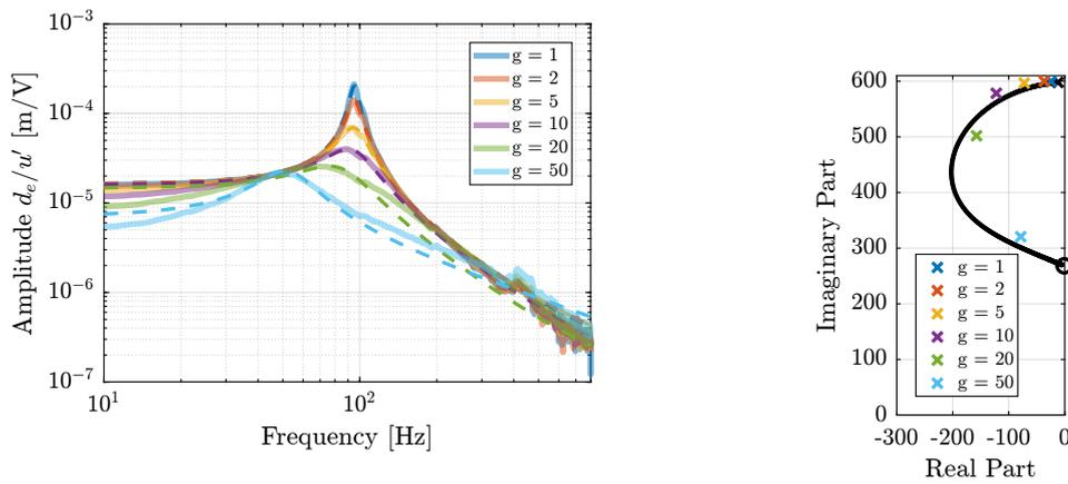
(a) Measured frequency response functions of damped plants for several IFF gains (solid lines). Identified 2nd order plants that match the experimental data (dashed lines) (b) Root locus plot using the plant model (black) and poles of the identified damped plants (color crosses)
