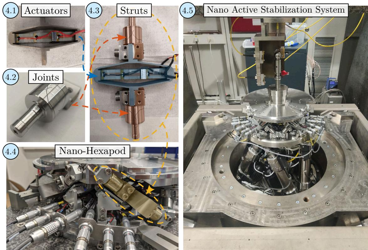
**Figure 4.1:** Overview of the experimental validation phase. The actuators and flexible joints and individual tested and then integrated into the struts. The Nano-hexapod is then mounted and the complete system is validated on the ID31 beamline.
