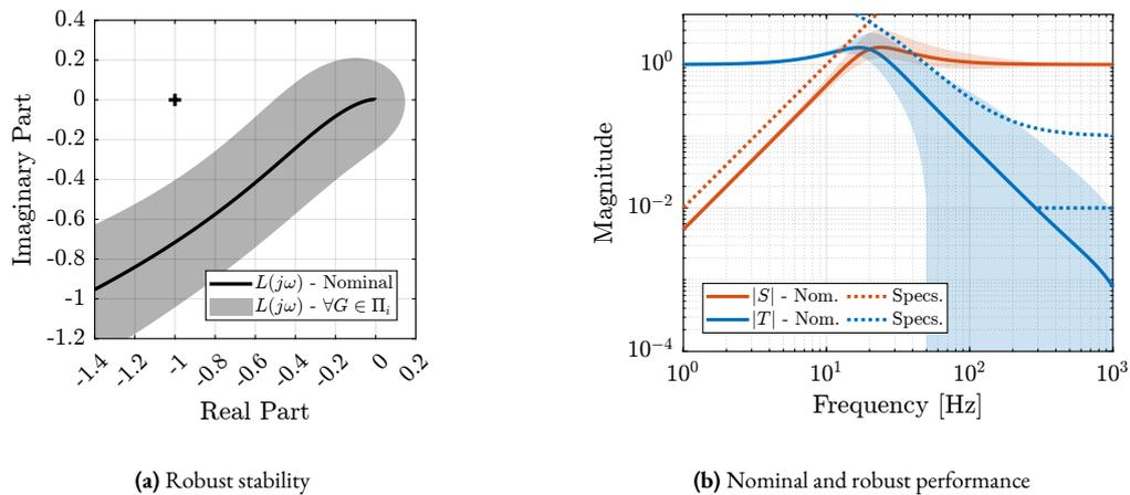
**Figure 3.71:** Validation of robust stability with the Nyquist plot (a) and validation of the nominal and robust performance with the magnitude of the closed-loop transfer functions (b).
