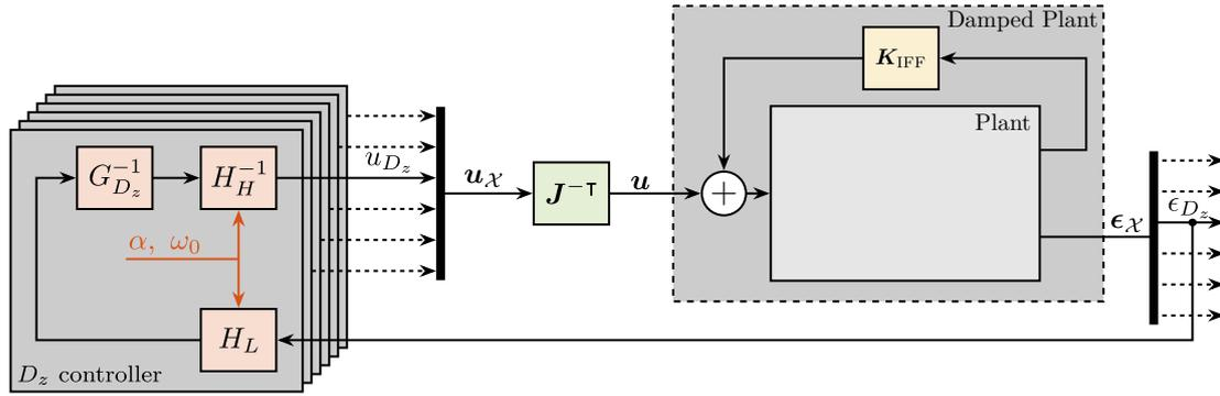
**Figure 4.113:** Control architecture using complementary filters proposed in Section 3.3.3, here adapted for the NASS. Jacobian matrices are used to have the control in the Cartesian frame. Only the  $D_z$  controller is shown.  $H_L$  and  $H_H$  are complementary filters.
