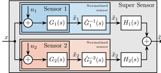
Figure 3.46: Sensor fusion architecture with two normalized sensors.
