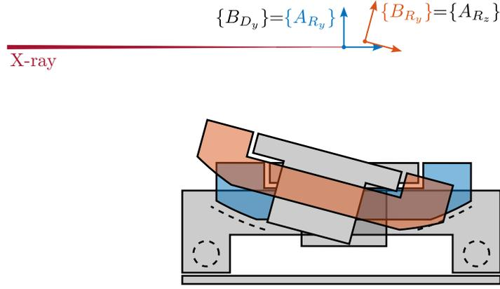
**Figure 2.83:** Example of the motion induced by the tilt-stage  $R_y$ . Initial position is shown in blue while an arbitrary position is shown in red. Parasitic motions are here magnified for clarity.
