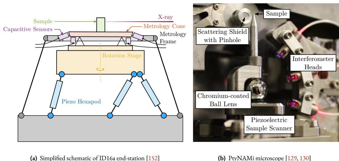
(a) Simplified schematic of ID16a end-station [152]
