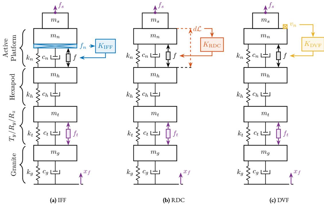
**Figure 2.12:** Three active damping strategies. Integral Force Feedback (a) using a force sensor, Relative Damping Control (b) using a relative displacement sensor, and Direct Velocity Feedback (c) using a geophone.
