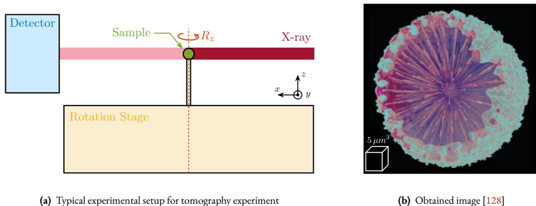
(a) Typical experimental setup for tomography experiment
