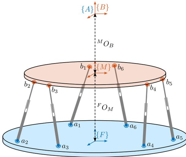
Figure 2.108: Geometrical parameters of the Stewart platform.
