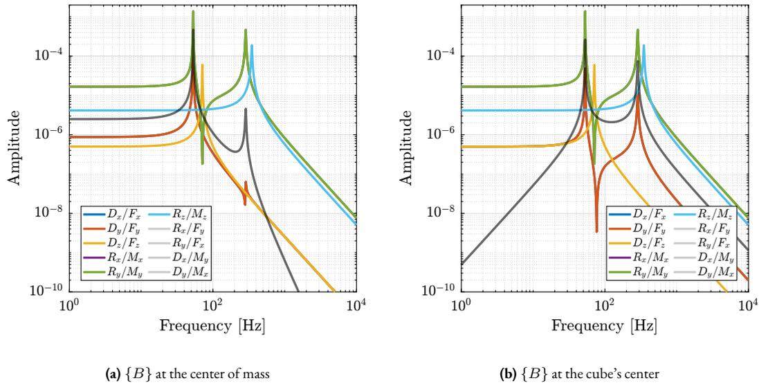
**Figure 3.12:** Transfer functions for a cubic Stewart platform expressed in the Cartesian frame. Two locations of the  $\{B\}$  frame are considered: at the center of mass of the moving body (a) and at the cube's center (b).
