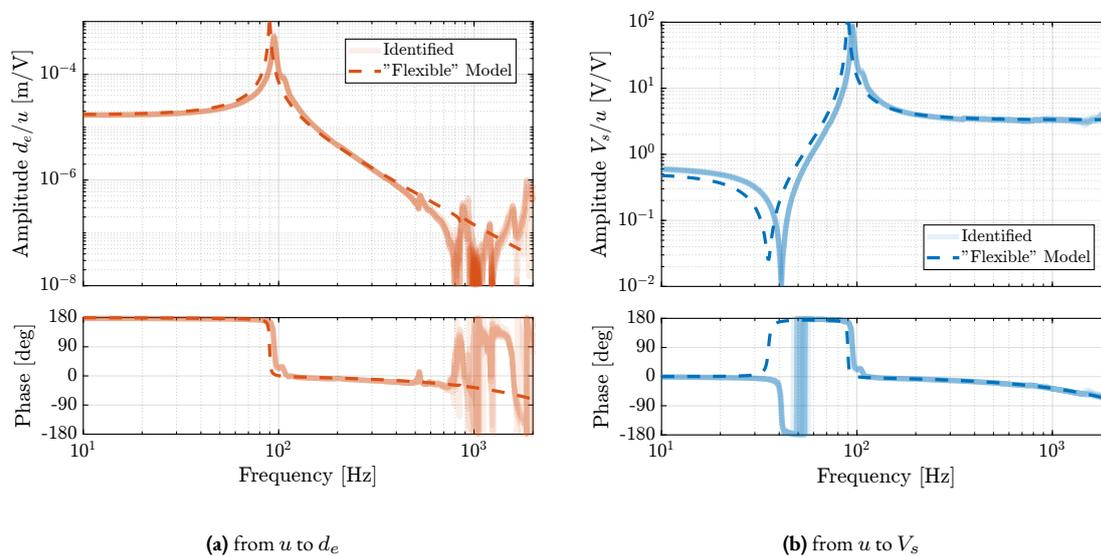
**Figure 4.23:** Comparison of the measured frequency response functions and the identified dynamics from the finite element model of the APA300ML. Both for the dynamics from  $u$  to  $d_e$  (a) and from  $u$  to  $V_s$  (b).
