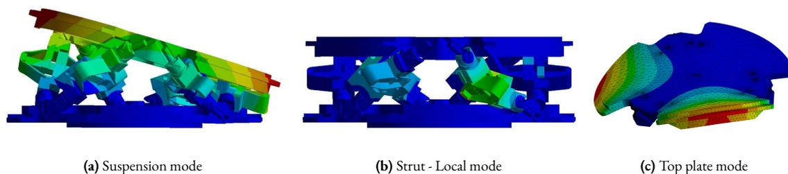
**Figure 3.97:** Finite Element Model of the nano-hexapod. The first six modes are “suspension” modes in which the top plate behaves as a rigid body (a). Then modes of the struts have natural frequencies from 205 Hz to 420 Hz (b). Finally, the first flexible mode of the top plate is at 650 Hz (c).
