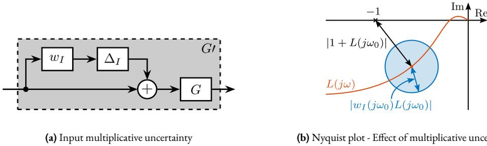
**Figure 3.66:** Input multiplicative uncertainty used to model the differences between the model and the physical plant (a). Effect of this uncertainty is illustrated on the Nyquist plot (b).
