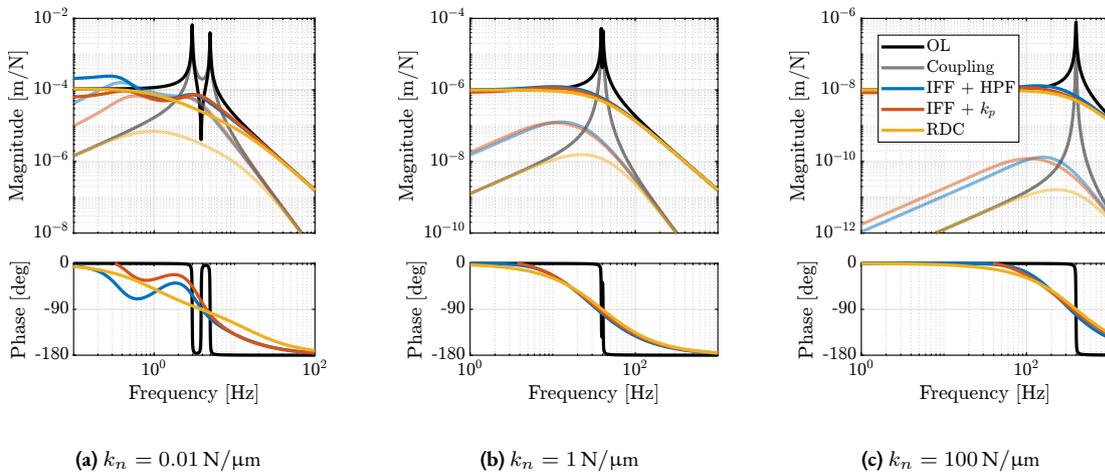
**Figure 2.57:** Comparison of the damped plants for the three proposed active damping techniques (IFF with HPF in blue, IFF with  $k_p$  in red and RDC in yellow). The direct terms are shown by solid lines, and the coupling terms are shown by the shaded lines. Three active platform stiffnesses are considered. Rotating velocity is  $\Omega = 60$  rpm and the suspended mass is  $m_n + m_s = 16$  kg.
