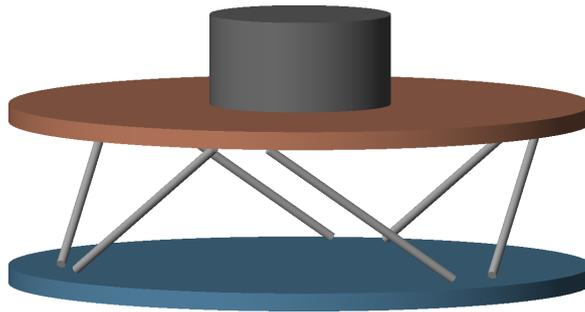
Figure 3.11: Cubic Stewart platform with cylindrical payload located on the top platform.
