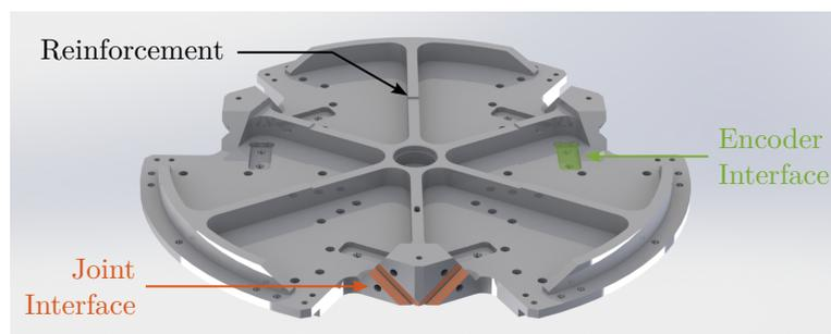
**Figure 3.95:** The mechanical design for the top platform incorporates precisely positioned V-grooves for the joint interfaces (displayed in red). The purpose of the encoder interface (shown in green) is later detailed.
