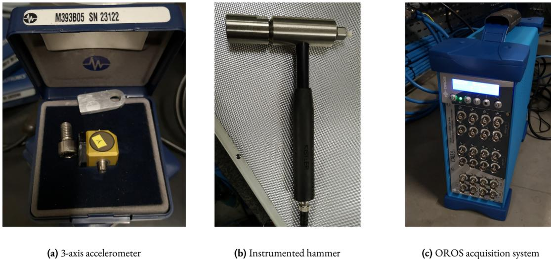
**Figure 2.64:** Instrumentation used for the modal analysis.
