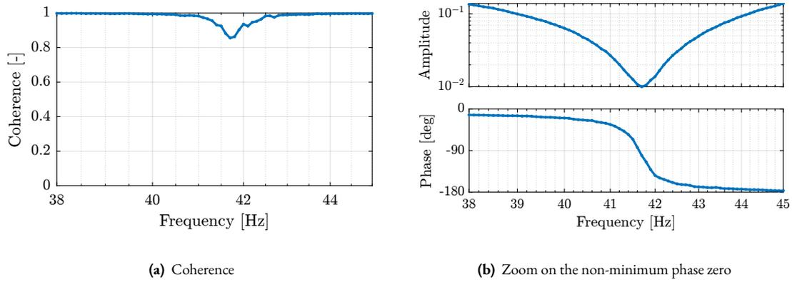
**Figure 4.13:** Measurement of the anti-resonance found in the transfer function from  $u$  to  $V_s$ . The coherence (a) is quite good around the anti-resonance frequency. The phase (b) shows a non-minimum phase behavior.
