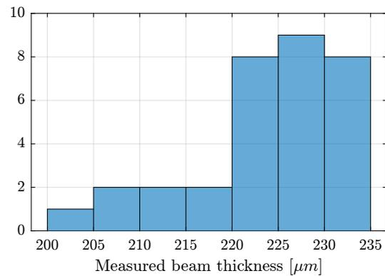
**Figure 4.27:** Histogram for the measured beams' thicknesses.
