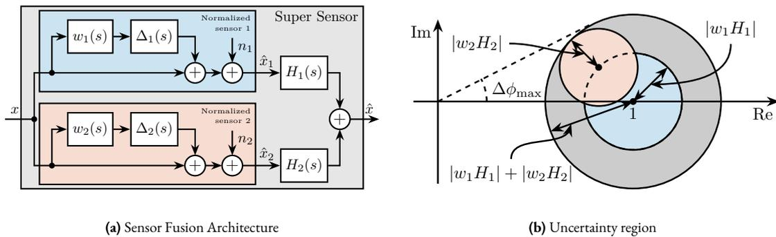
**Figure 3.48:** Sensor fusion architecture with sensor dynamics uncertainty (a). Uncertainty region (b) of the super sensor dynamics in the complex plane (grey circle). The contribution of both sensors 1 and 2 to the total uncertainty are represented respectively by a blue circle and a red circle. The uncertainty region is function of frequency, which is omitted.
