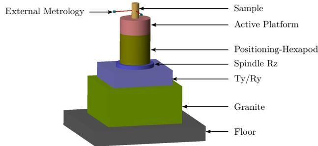
**Figure 2.58:** 3D view of the Nano-Active-Stabilization-System model.
