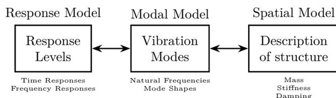
**Figure 2.63:** Three models of the same structure. The goal is to tune a spatial model (i.e. mass, stiffness and damping properties) from a response model. The modal model can be used as an intermediate step.
