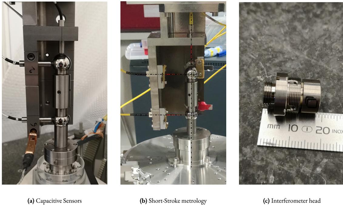
**Figure 4.76:** Short stroke metrology system used to measure the sample position with respect to the granite in 5-DoF. The system is based on a “Spindle error analyzer” (a), but the capacitive sensors are replaced with fibered interferometers (b). One interferometer head is shown in (c).
