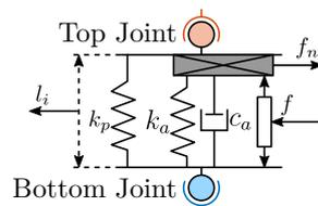
Figure 2.109: Model of the active platform actuators.
