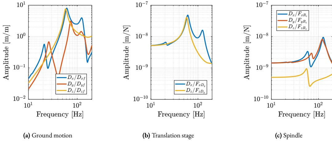
**Figure 2.95:** Extracted transfer functions from disturbances to relative motion between the micro-station’s top platform and the granite. The considered disturbances are the ground motion (a), the translation stage vibrations (b), and the spindle vibrations (c).
