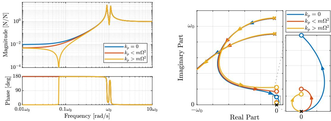
(a) Bode plots of  $f_u/F_u$  without parallel spring (blue), with parallel spring  $k_p < m\Omega^2$  (red) and  $k_p > m\Omega^2$ ,  $\Omega = 0.1\omega_0$  (yellow) (b) Root locus for IFF without parallel spring, with soft parallel spring and with stiff parallel spring
