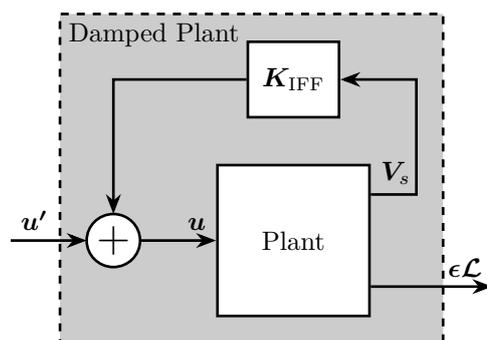
**Figure 4.89:** Block diagram of the implemented decentralized IFF controller. The controller  $K_{\text{IFF}}$  is a diagonal controller.
