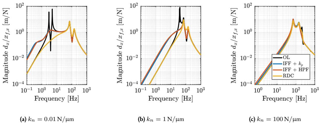
**Figure 2.60:** Effect of floor motion  $x_{f,x}$  on the position error  $d_x$  - Comparison of active damping techniques for the three active platform stiffnesses. IFF is shown to increase the sensitivity to floor motion at low-frequency.
