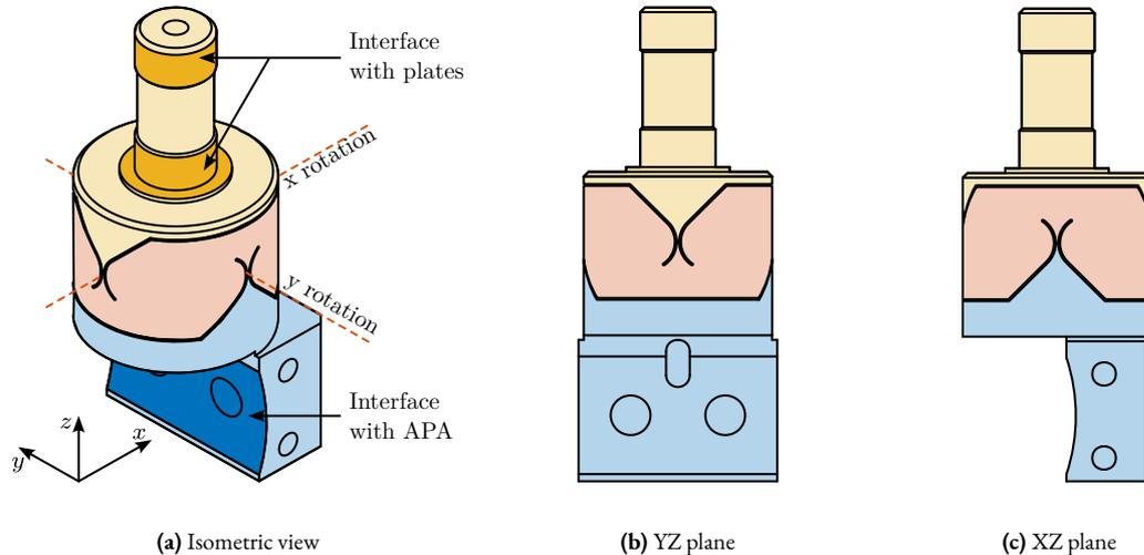
**Figure 4.24:** Geometry of the optimized flexible joints.
