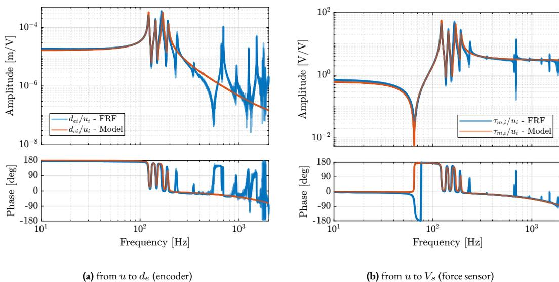
**Figure 4.70:** Comparison of the diagonal elements (i.e. “direct” terms) of the measured FRF matrix and the dynamics identified from the multi-body model. Both for the dynamics from  $u$  to  $d_e$  (a) and from  $u$  to  $V_s$  (b).
