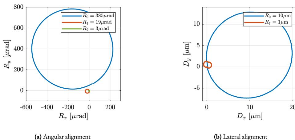
**Figure 4.80:** Measured angular (a) and lateral (b) errors during full spindle rotation. Between two rotations, the positioning hexapod is adjusted to better align the two spheres with the rotation axis.
