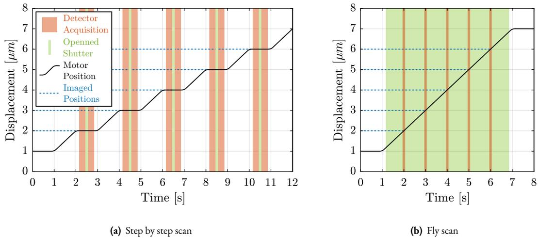
**Figure 1.10:** Two acquisition modes. In step-by-step mode (a), the motor moves to the desired imaged position, the detector acquisition is started, the shutter is opened briefly to have the wanted exposure, the detector acquisition is stopped, and the motor can move to a new position. In *fly-scan* mode (b), the shutter is opened while the sample is in motion, and the detector acquires data only at the desired positions while in motion (“on the fly”).
