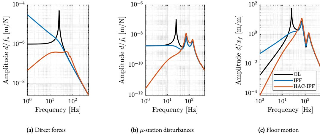
**Figure 2.26:** Change of sensitivity to disturbances with LAC and with HAC-LAC. An active platform with  $k_n = 1 \text{ N}/\mu\text{m}$  and a sample mass of 25 kg are used. Disturbances are:  $f_s$  the direct forces applied on the sample (a),  $f_t$  the disturbances from the micro-station stages (b) and  $x_f$  the floor motion (c).
