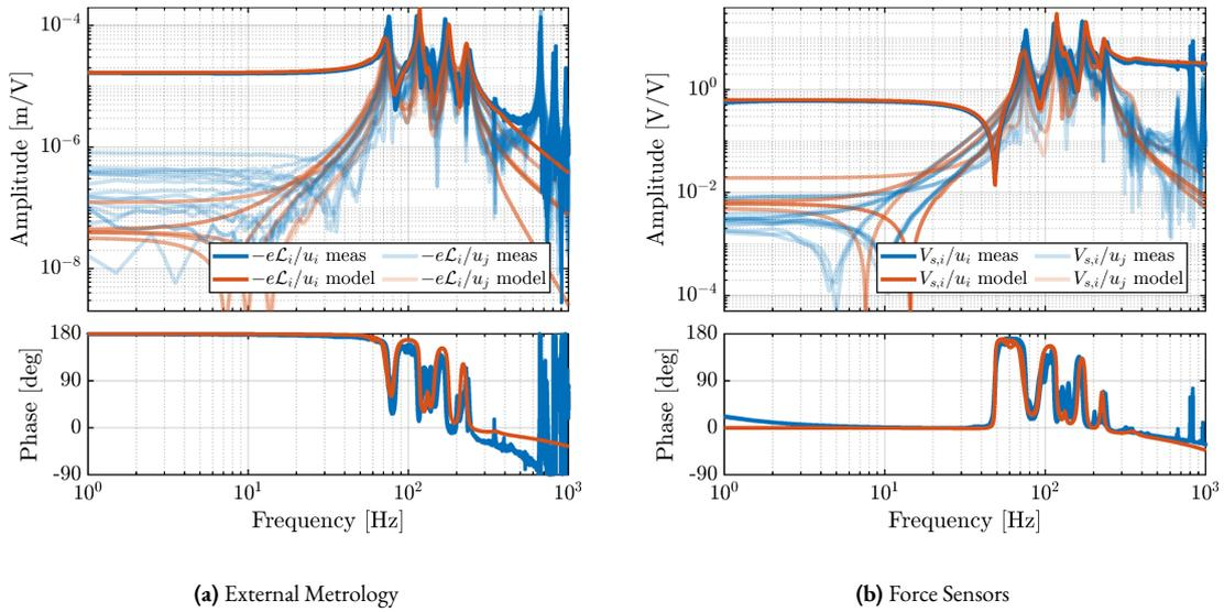
**Figure 4.83:** Comparison between the measured dynamics and the multi-body model dynamics. Both for the external metrology (a) and for force sensors (b). Direct terms are displayed with solid lines while off-diagonal (i.e. coupling) terms are displayed with shaded lines.
