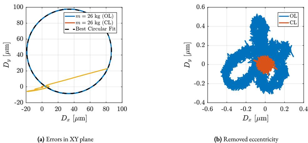
**Figure 4.101:** Tomography experiment with a rotation velocity of 6 deg/s, and payload mass of 26 kg. Errors in the XY plane are shown in (a). The estimated eccentricity is represented by the black dashed circle. The errors with subtracted eccentricity are shown in (b).
