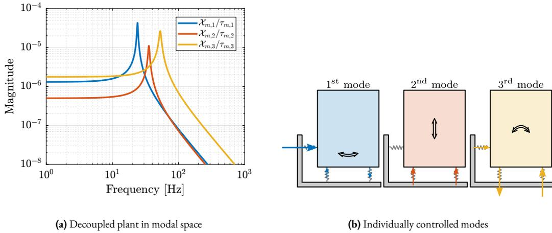
**Figure 3.60:** Plant using modal decoupling consists of second order plants (a). Decoupled elements can be used to individually address the modes illustrated in (b).
