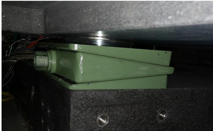
**Figure 2.74:** AirLoc used for the granite (2120-KSKC).
