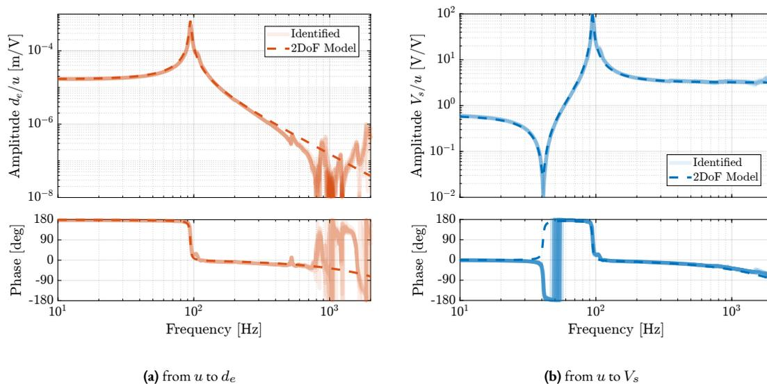
**Figure 4.21:** Comparison of the measured frequency response functions and the identified dynamics from the 2-DoF model of the APA300ML. Both for the dynamics from  $u$  to  $d_e$  (a) and from  $u$  to  $V_s$  (b).
