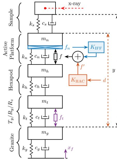
**Figure 2.35:** Uniaxial model considering some flexibility between the active platform top platform and the sample. In this case, the measured and controlled distance  $d$  is different from the distance  $y$  which is the real performance index.
