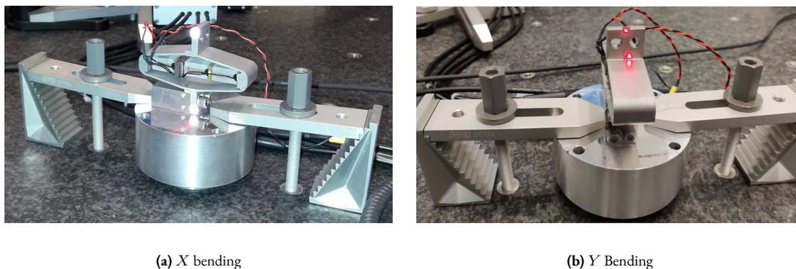
**Figure 4.8:** Experimental setup to measure the flexible modes of the APA300ML. For the bending in the  $X$  direction (a), the hammer impact point is at the back of the top measurement point. For the bending in the  $Y$  direction (b), the hammer impact point is located at the back of the top measurement point.
