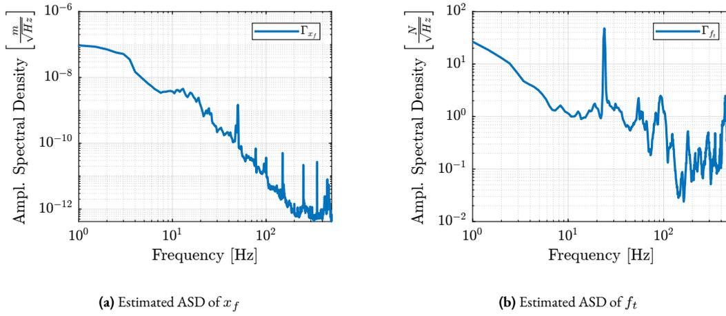
**Figure 2.8:** Estimated amplitude spectral density of the floor motion  $x_f$  (a) and of the stage disturbances  $f_t$  (b). Data are shown between 1 and 500 Hz, a frequency range for which the measurement quality is good.
