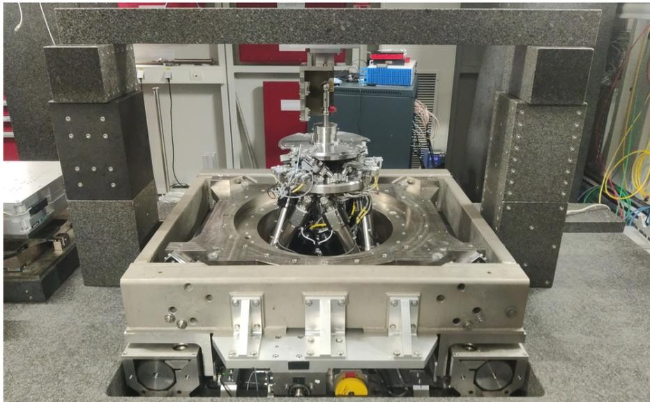
**Figure 4.79:** Granite gantry used to fix the short-stroke metrology system.
