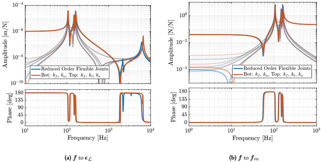
**Figure 3.42:** Comparison of the dynamics obtained between an active platform including joints modelled with FEM and an active platform having 2-DoF bottom joints and 3-DoF top joints. Both from actuator force  $f$  to strut motion measured by external metrology  $\epsilon_{\mathcal{L}}$  (a) and to the force sensors  $f_m$  (b).
