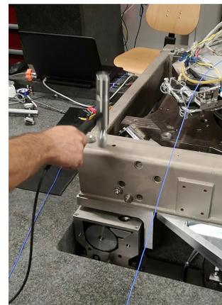
(c)  $Z$  impact**Figure 2.67:** The three hammer impacts used for the modal analysis.
