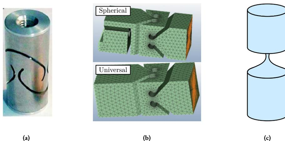
**Figure 3.35:** Example of different flexible joints geometry used for Stewart platforms. (a) Typical “universal” flexible joint used in [117]. (b) Torsional stiffness can be explicitly specified as done in [160]. (c) “Thin” flexible joints having “notch curves” [41].
