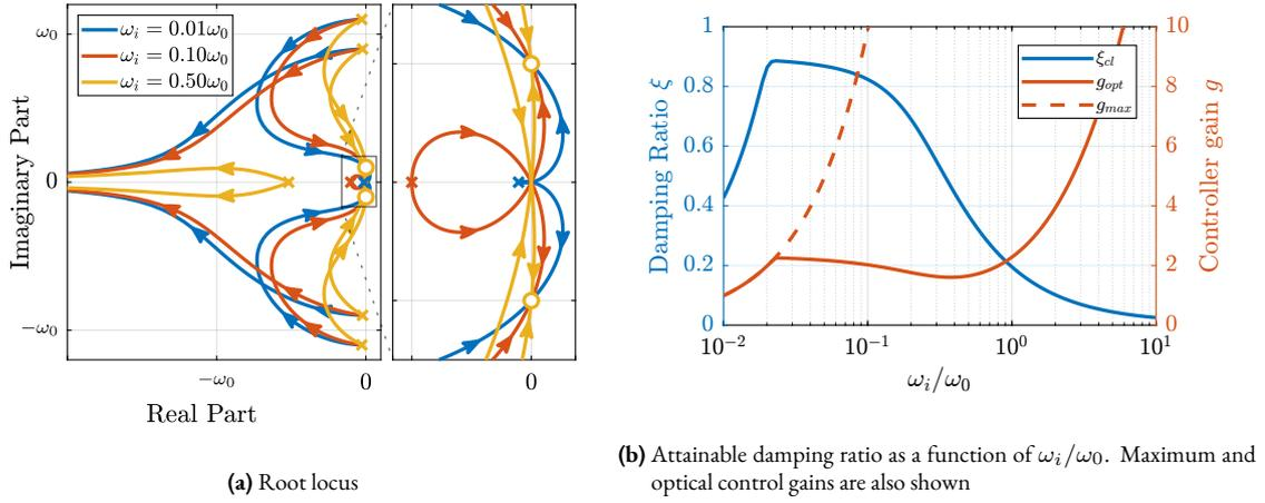
**Figure 2.43:** Root loci for several high-pass filter cut-off frequency (a). Achievable damping ratio decreases as  $\omega_i$  increases (b).
