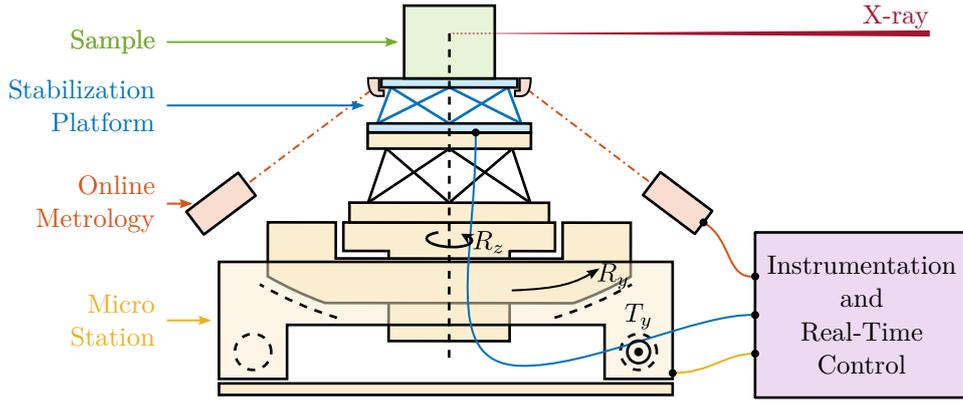
**Figure 2.123:** Schematic of the Nano Active Stabilization System.
