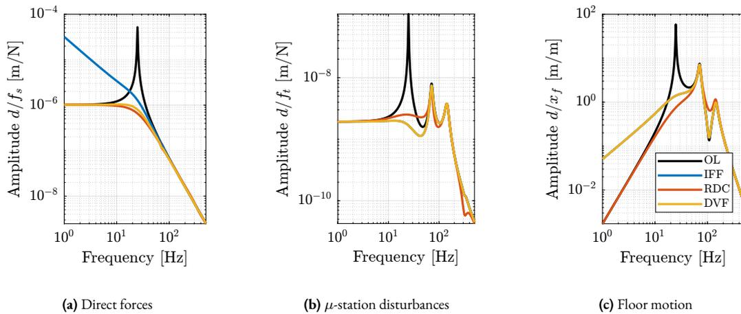
**Figure 2.20:** Change of sensitivity to disturbances for all three active damping strategies. Considered disturbances are  $f_s$  the direct forces applied on the sample (a),  $f_t$  disturbances from the micro-station stages (b) and  $x_f$  the floor motion (c). Sensitivity for IFF (displayed in blue) is superimposed with the sensitivity for DVF (yellow).
