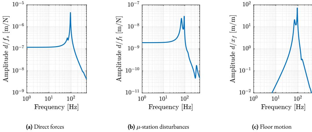
**Figure 2.5:** Sensitivity of the relative motion  $d$  to the following disturbances:  $f_s$  the direct forces applied on the sample (a),  $f_t$  disturbances from the micro-station stages (b) and  $x_f$  the floor motion (c).
