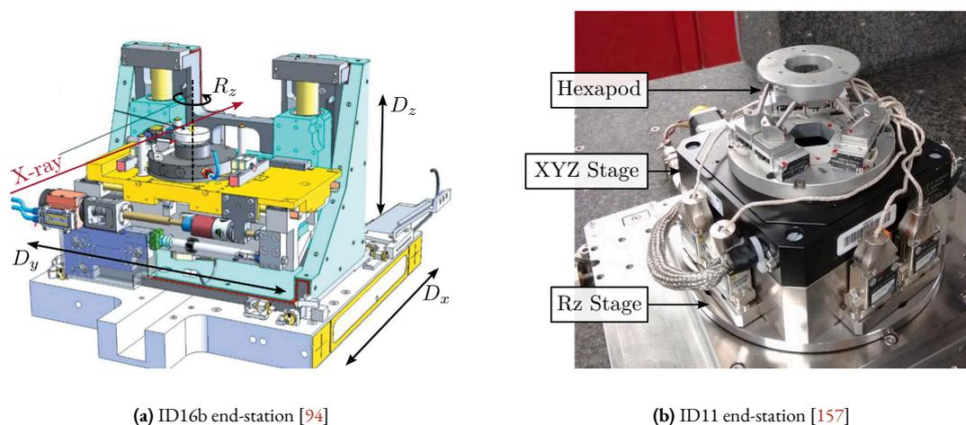
**Figure 1.12:** Example of two nano end-stations lacking online metrology for measuring the sample's position.
