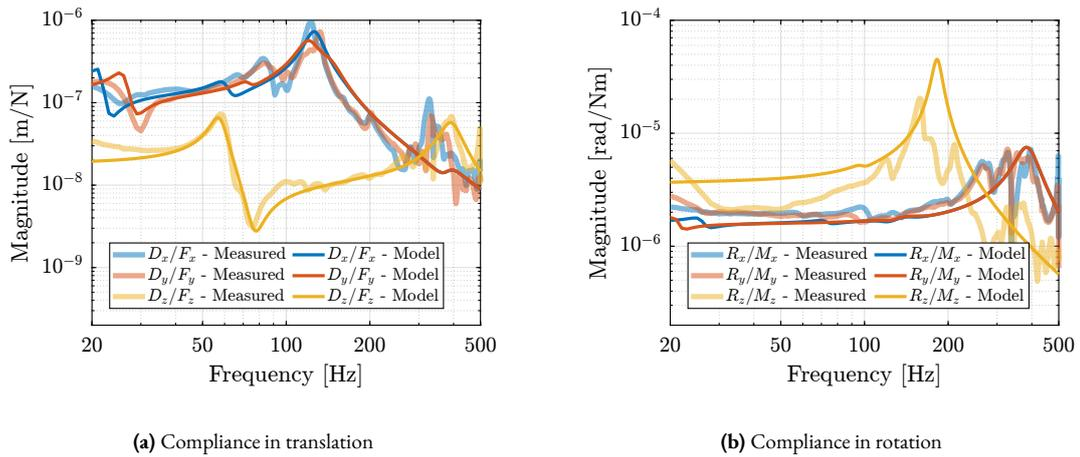
**Figure 2.88:** Compliance of the micro-station expressed in frame  $\{\mathcal{X}\}$ . The measured FRFs are displayed by translucent lines, while the FRFs extracted from the multi-body models are shown by opaque lines. Both translation terms (a) and rotational terms (b) are displayed.
