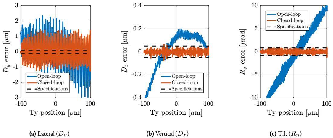
**Figure 4.110:** Open-Loop (in blue) and Closed-loop (i.e. using the NASS, in red) during a 100  $\mu\text{m}/\text{s}$  scan with the  $T_y$  stage.
