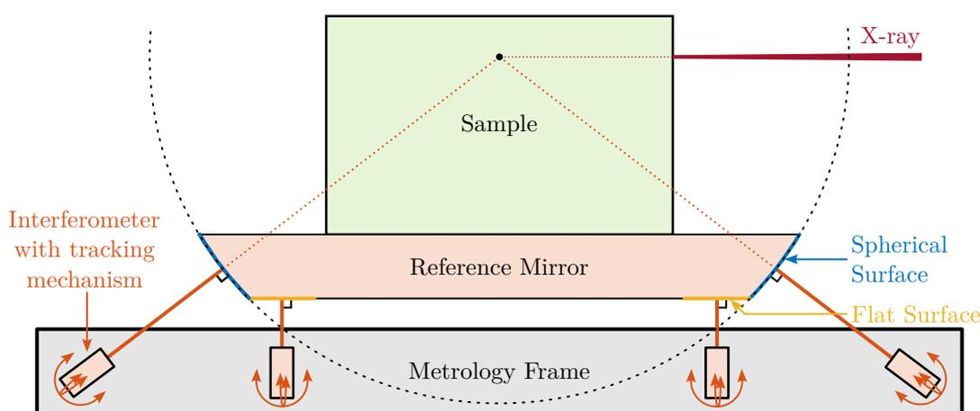
**Figure 1.17:** 2D representation of the NASS metrology system.
