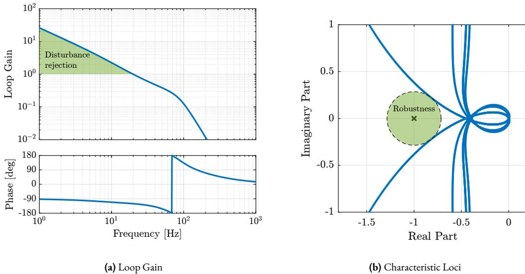
**Figure 2.121:** Decentralized HAC-IFF. Loop gain (a) is used for the design of the controller and to estimate the disturbance rejection level. Characteristic Loci (b) is used to verify the stability and robustness of the feedback loop.
