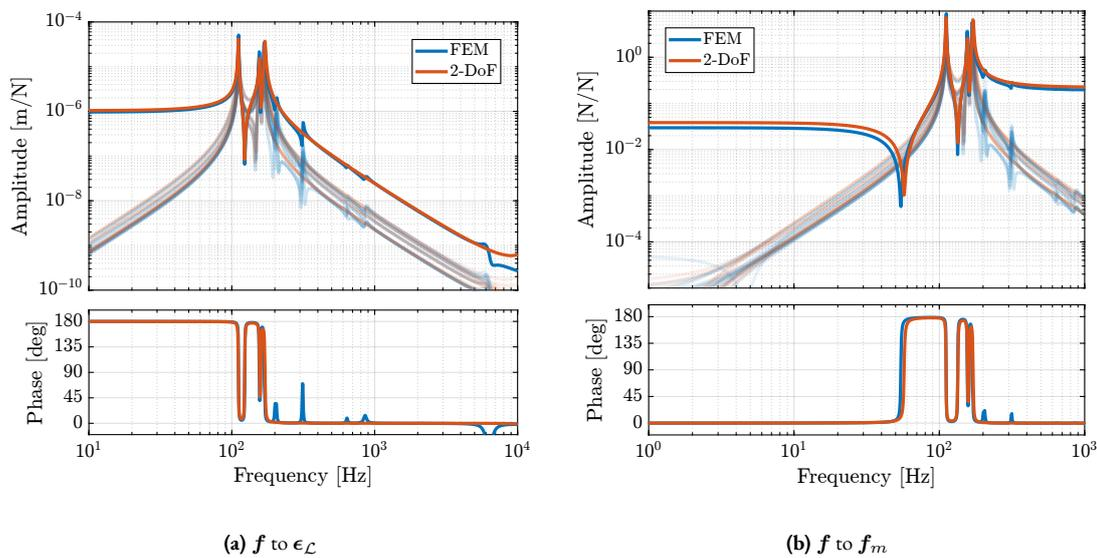
**Figure 3.34:** Comparison of the dynamics obtained between an active platform having the actuators modelled with FEM and an active platform having actuators modelled as 2-DoF system. Both from actuator force  $\mathbf{f}$  to strut motion measured by external metrology  $\epsilon_{\mathcal{L}}$  (b) and to the force sensors  $\mathbf{f}_m$  (a).
