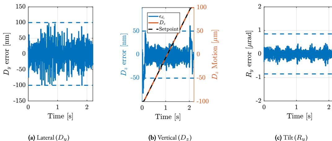
**Figure 4.108:**  $D_z$  scan at a velocity of  $100 \mu\text{m/s}$ .  $D_z$  setpoint, measured position and error are shown in (b). Errors in  $D_y$  and  $R_y$  are respectively shown in (a) and (c).
