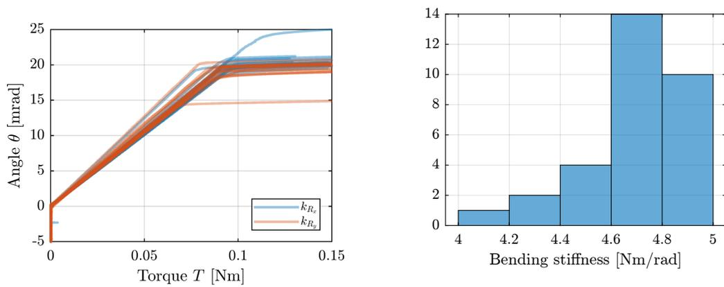
(a) Measured torque and angular motion for the flexible joints
