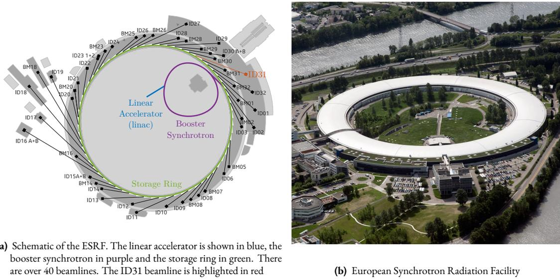
(a) Schematic of the ESRF. The linear accelerator is shown in blue, the booster synchrotron in purple and the storage ring in green. There are over 40 beamlines. The ID31 beamline is highlighted in red
