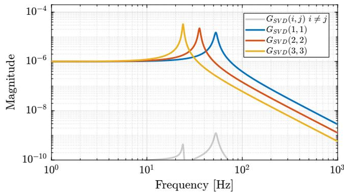
**Figure 3.62:** Plant dynamics  $\mathbf{G}_{\text{SVD}}(s)$  obtained after decoupling using Singular Value Decomposition.
