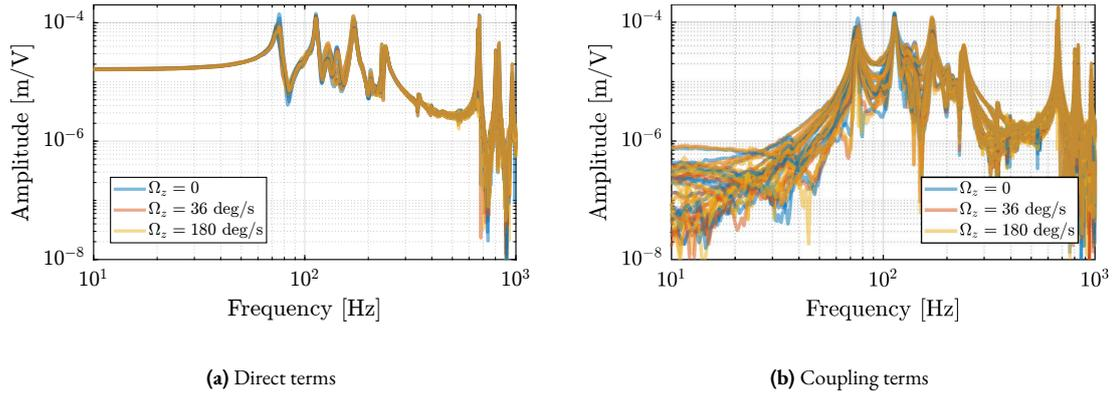
**Figure 4.88:** Effect of the spindle rotation on the plant dynamics from  $u$  to  $\epsilon\mathcal{L}$ . Three rotational velocities are tested (0 deg/s, 36 deg/s and 180 deg/s). Both direct terms (a) and coupling terms (b) are displayed.
