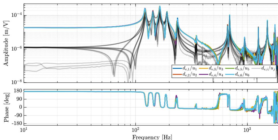
**Figure 4.65:** Measured FRFs from  $u$  to  $d_e$ . The 6 direct terms are the colored lines, and the 30 coupling terms are the gray lines.
