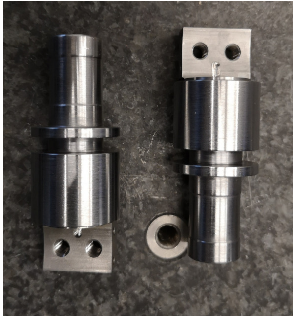
Figure 1.5: Step 1 - Flexible joints fixed on the cylindrical interface elements
