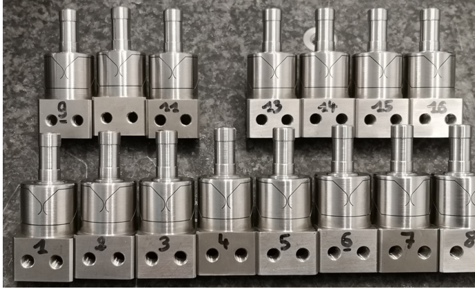
(a) 15 of the 16 received flexible joints
