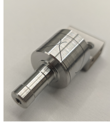
(b) Zoom on one flexible joint
