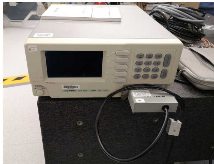
Figure 1.2: LCR Meter used for the measurements
