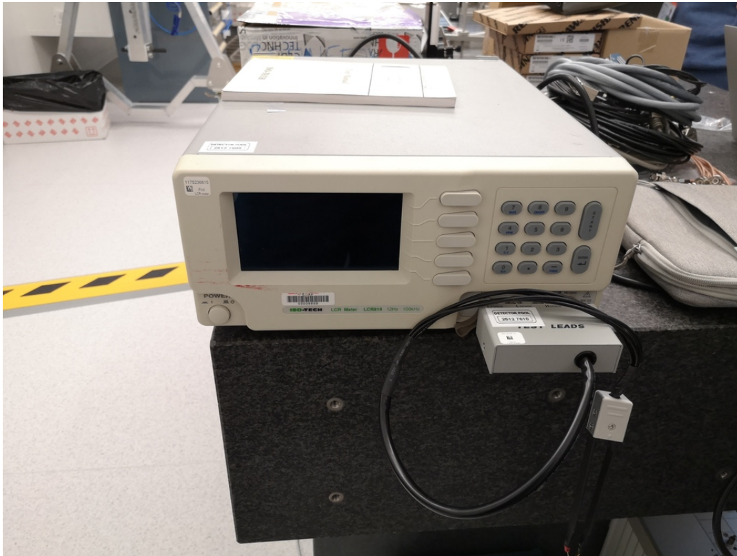
Figure 2.3: LCR Meter used for the measurements
