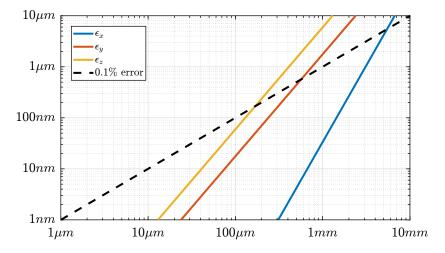
Figure 2.4: Errors associated with the use of the Jacobian matrix to solve the forward kinematic problem
