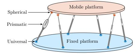
Figure 2.1: Schematical representation of the Stewart platform architecture.
