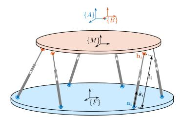
Figure 2.2: Frame and key notations for the Stewart platform
