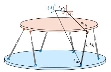
Figure 2.3: Notations to compute the kinematic loop closure
