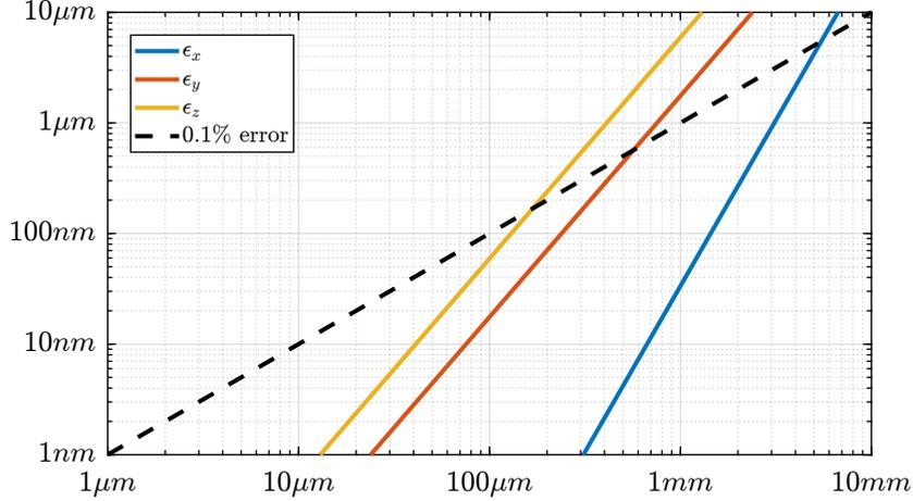
**Figure 2.4:** Errors associated with the use of the Jacobian matrix to solve the forward kinematic problem
