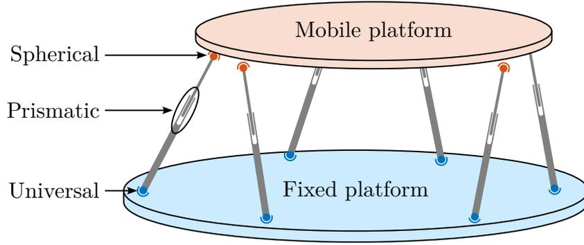
**Figure 2.1:** Schematical representation of the Stewart platform architecture.
