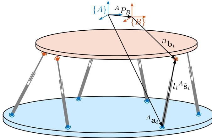
Figure 2.3: Notations to compute the kinematic loop closure
