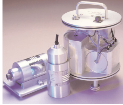
Figure 3.2: (3D) L-4C geophone
