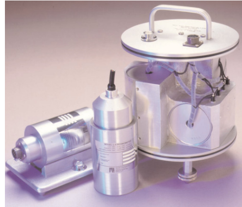
Figure 3.2: (3D) L-4C geophone
