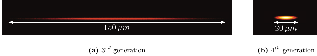
Figure 1.8: View of the ESRF X-ray beam before the EBS upgrade (a) and after the EBS upgrade (b). The brilliance is increased, whereas the horizontal size and emittance are reduced.
