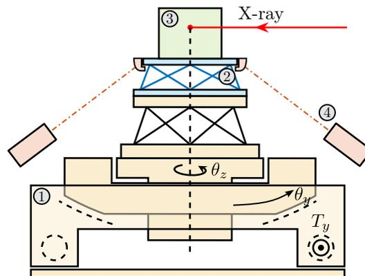
**Figure 2.1:** Nass Concept. 1: micro-station, 2: nano-hexapod, 3: sample, 4: 5DoF metrology
