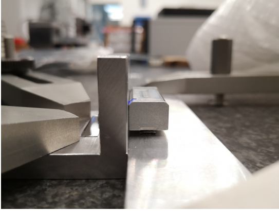
Figure 3.12: Test bench used to measured the encoder noise
