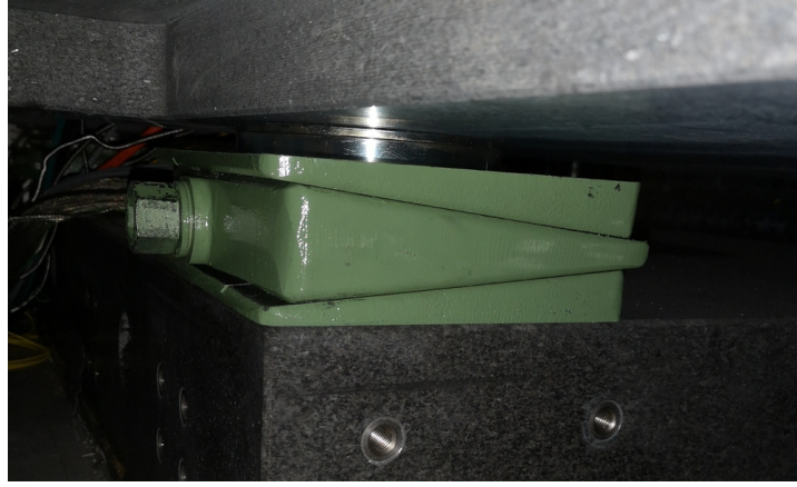
Figure 3.3: AirLoc used for the granite (2120-KSKC)
