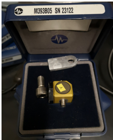
(a) 3-axis accelerometer
