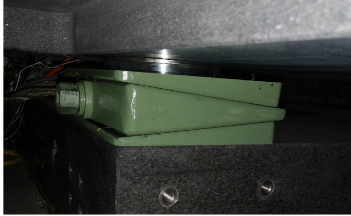
Figure 3.5: AirLoc used for the granite (2120-KSKC)
