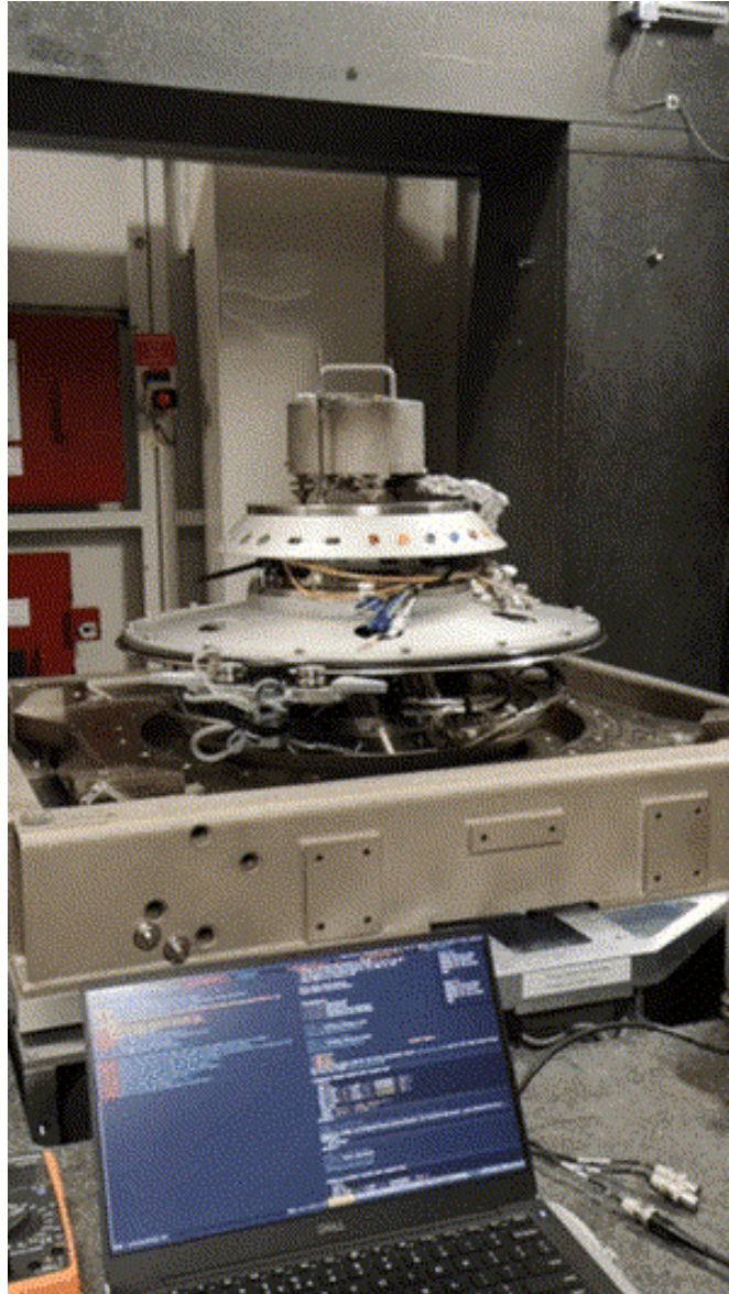
Figure 15 – Measurement of the sample's vertical motion when rotating at 6rpm
