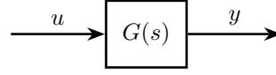
Figure 5 – LTI dynamical system G(s) with input signal u and output signal y
