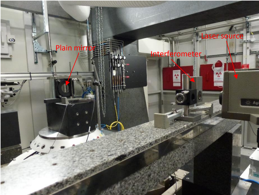
Measurement setup of the angular deviation measurement R Yy (See picture below).
