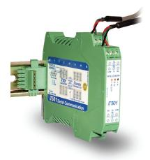
The *iT* Series provides a low cost online condition monitoring system. Once a potential problem is identified, a portable vibration analyzer can be attached to the front of the transmitter for a complete detailed analysis.
