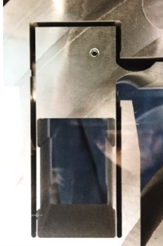
Figure 25: Use leaf springs instead of linear roller bearings
