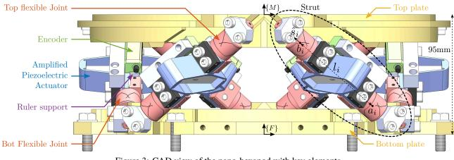
Figure 3: CAD view of the nano-hexapod with key elements
