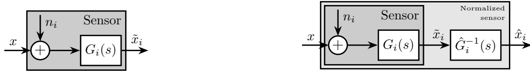
(a) Basic sensor model consisting of a noise input n_i and a linear time invariant transfer function G_i(s) (b) Normalized sensors using the inverse of an estimate \hat{G}_i(s) of the sensor dynamics
