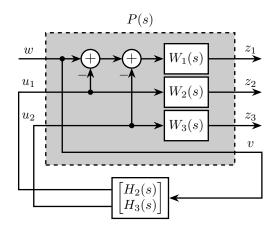
Figure 7: Architecture for  $\mathcal{H}_{\infty}$  synthesis of three complementary filters
