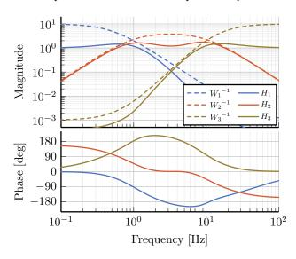
Figure 8: Frequency response of the weighting functions and three complementary filters obtained using  $\mathcal{H}_{\infty}$  synthesis
