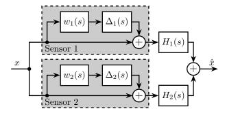
Figure 2: Sensor fusion architecture with sensor dynamics uncertainty
