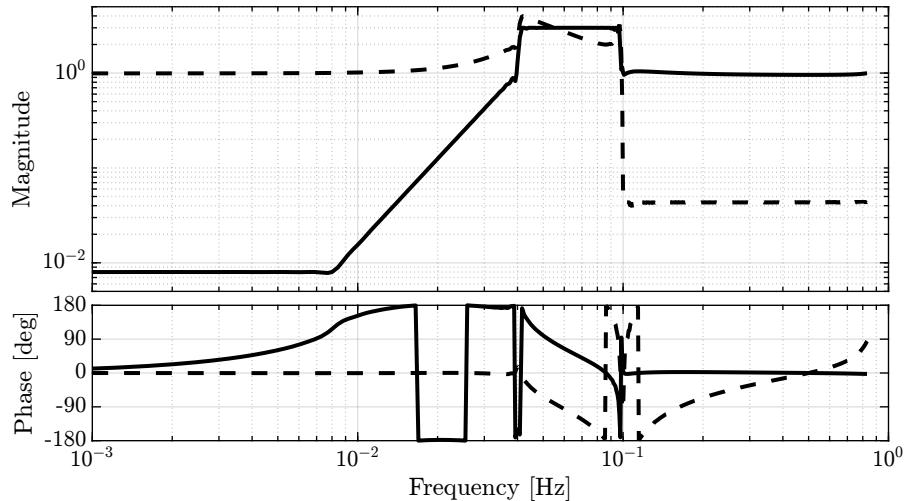
**Figure 3.2:** FIR Complementary filters obtain after convex optimization
