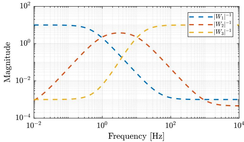
**Figure 2.2:** Three weighting functions used for the  $\mathcal{H}_\infty$  synthesis of the complementary filters
