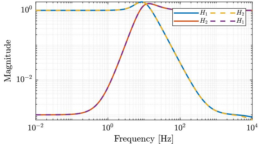
**Figure 4.4:** Comparison of  $H_1(s)$  with  $1 - H_2(s)$ , and  $H_2(s)$  with  $1 - H_1(s)$
