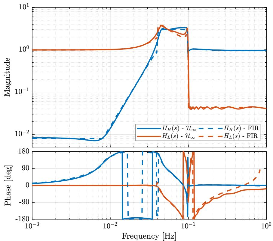
**Figure 3.5:** Comparison between the FIR filters developed for LIGO and the  $\mathcal{H}_\infty$  complementary filters
