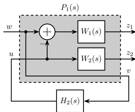
**Figure 4.1:** Complementary Filter Synthesis - Conf 1
