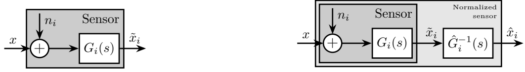
(a) Basic sensor model consisting of a noise input n_i and a dynamics G_i(s) (b) Calibrated sensors using the inverse of an estimate \hat{G}_i(s) of the sensor dynamics
