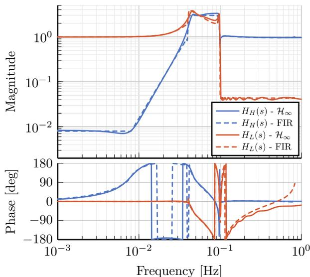
Figure 10: Comparison of the FIR filters (solid) designed in [6] with the filters obtained with  $\mathcal{H}_\infty$  synthesis (dashed)
