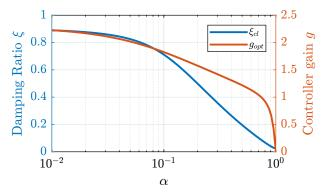
Figure 16: Optimal damping ratio  $\xi_{\rm opt}$  and the corresponding optimal gain  $g_{\rm opt}$  as a function of  $\alpha$
