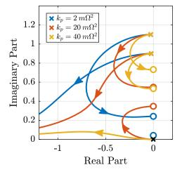
Figure 15: Comparison of the Root Locus plots for three parallel stiffnesses  $k_p$
