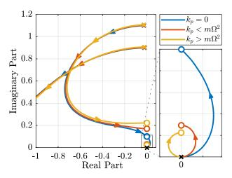
Figure 14: Root Locus for IFF without parallel spring, with parallel spring stiffness  $k_p < m\Omega^2$  and  $k_p > m\Omega^2$ ,  $\Omega = 0.1\omega_0$
