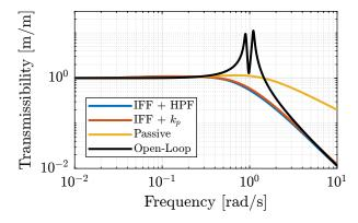
Figure 18: Comparison of the two proposed active damping techniques - transmissibility
