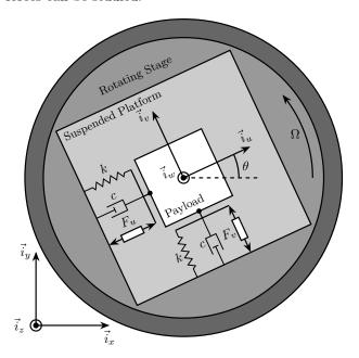
Figure 1: Schematic of the studied system
