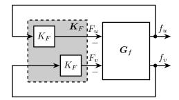
Figure 5: Control diagram for decentralized IFF
