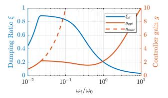
Figure 11: Attainable damping ratio  $\xi_{\rm cl}$  as a function of  $\omega_i/\omega_0$ . Corresponding control gain  $g_{\rm opt}$  and  $g_{\rm max}$  are also shown
