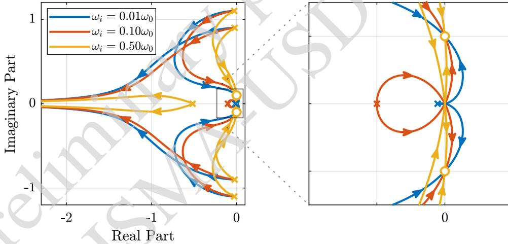
Figure 10: Root Locus for several HFP cut-off frequencies  $\omega_i$ ,  $\Omega = 0.1\omega_0$
