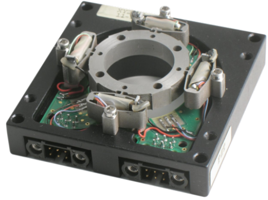
Figure 13. XY Piezoelectric Stage (XY25XS from Cedrat Technology)
