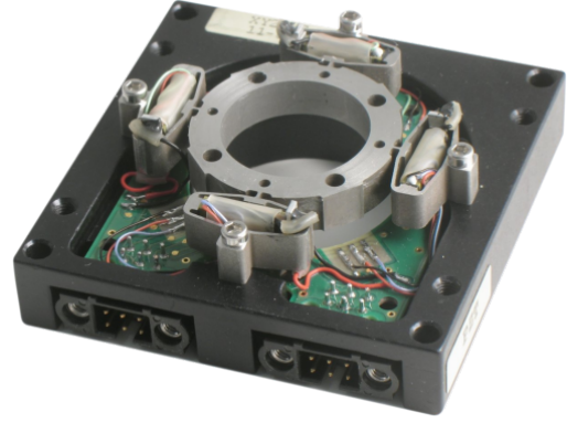
Figure 12: Studied system with additional springs in parallel with the actuators and force sensors Figure 13: XY Piezoelectric Stage (XY25XS from Cedrat Technology)
