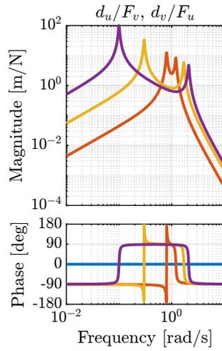
**Figure 1.6:** Comparison of the transfer functions from  $[F_u, F_v]$  to  $[d_u, d_v]$  for several rotating speed - Coupling Terms
