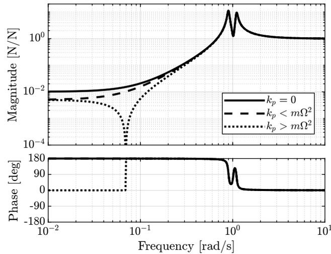
Figure 4.3: Transfer function from  $[F_u, F_v]$  to  $[f_u, f_v]$  for  $k_p = 0$ ,  $k_p < m\Omega^2$  and  $k_p > m\Omega^2$
