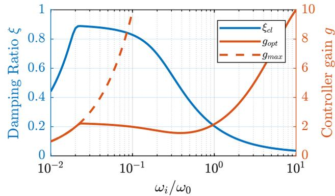
**Figure 3.6:** Simultaneous attainable damping of the closed loop poles as a function of  $\omega_i$
