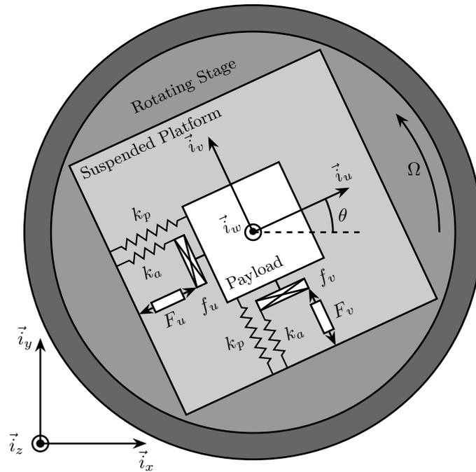
**Figure 4.1:** Studied system with additional springs in parallel with the actuators and force sensors
