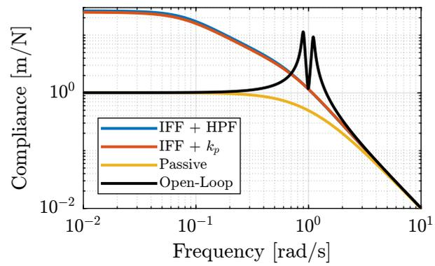
**Figure 5.3:** Comparison of the obtained Compliance
