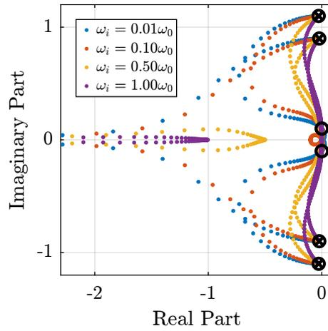
**Figure 3.4:** Root Locus for the modified IFF controller (zoomed plot on the left)
