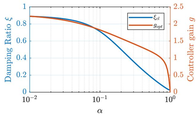
**Figure 4.7:** Attainable damping ratio and corresponding controller gain for different parameter  $\alpha$
