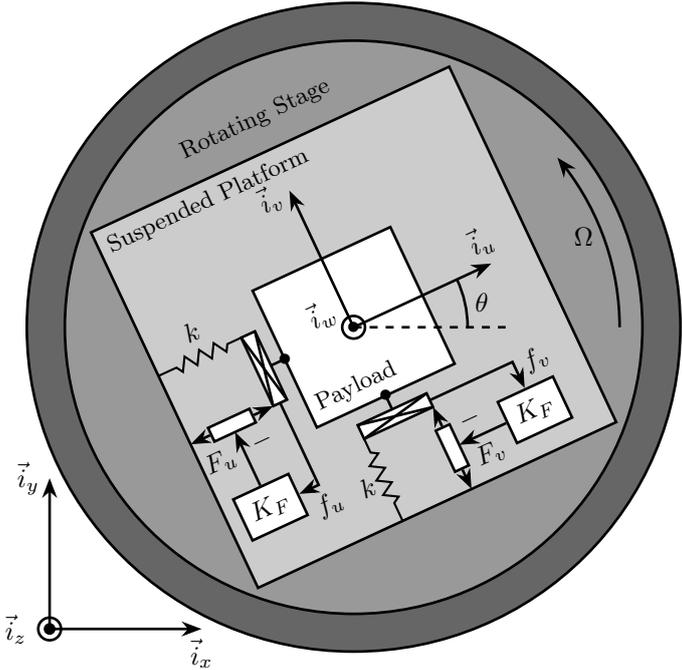
Figure 2.1: System with added Force Sensor in series with the actuators
