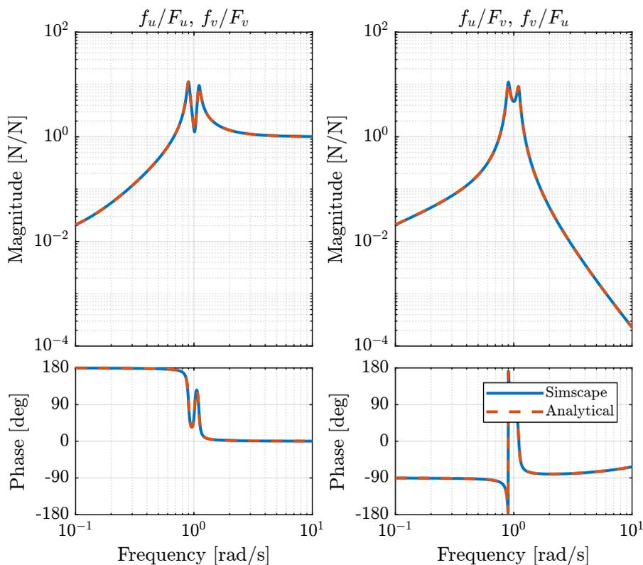
**Figure 2.2:** Comparison of the transfer functions from  $[F_u, F_v]$  to  $[f_u, f_v]$  between the Simscape model and the analytical one
