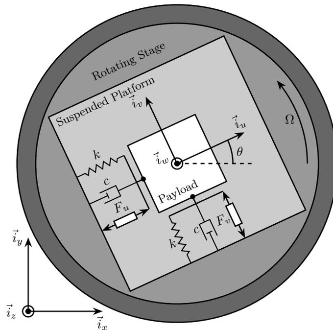
**Figure 1.1:** Schematic of the studied system
