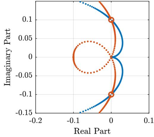
**Figure 3.3:** Root Locus for the modified IFF controller - Zoom
