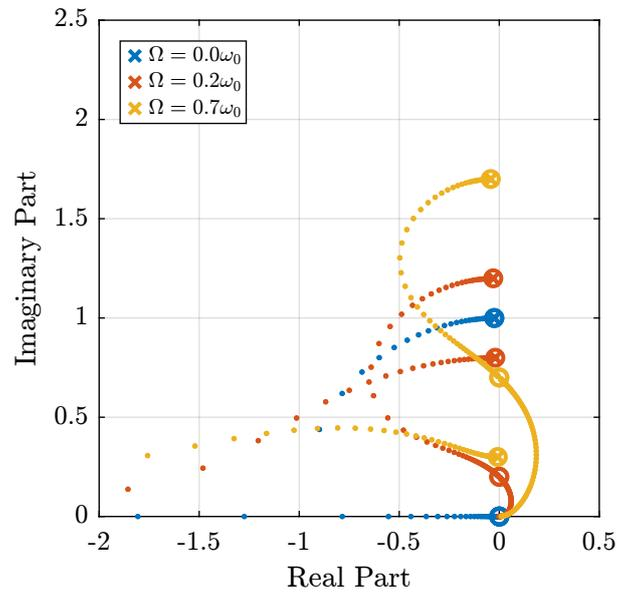
**Figure 2.4:** Root Locus for the Decentralized Integral Force Feedback controller. Several rotating speed are shown.
