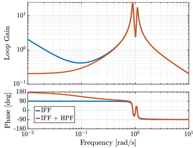
Figure 3.1: Loop Gain for the modified IFF controller
