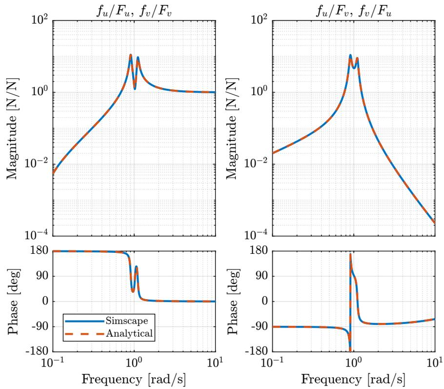
**Figure 4.2:** Comparison of the transfer functions from  $[F_u, F_v]$  to  $[f_u, f_v]$  between the Simscape model and the analytical one
