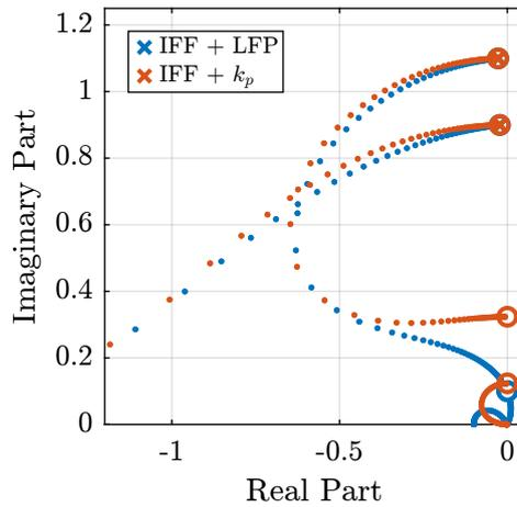
**Figure 5.1:** Root Locus plot - Comparison of IFF with additional high pass filter, IFF with additional parallel stiffness
