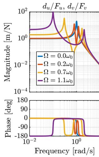
**Figure 1.5:** Comparison of the transfer functions from  $[F_u, F_v]$  to  $[d_u, d_v]$  for several rotating speed - Direct Terms
