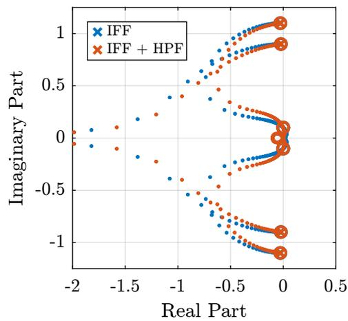
Figure 3.2: Root Locus for the modified IFF controller
