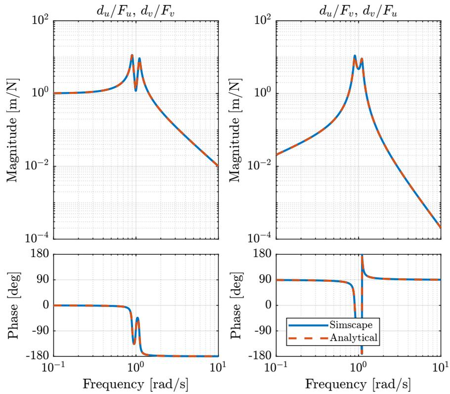
**Figure 1.4:** Bode plot of the transfer function from  $[F_u, F_v]$  to  $[d_u, d_v]$  as identified from the Simscape model and from an analytical model
