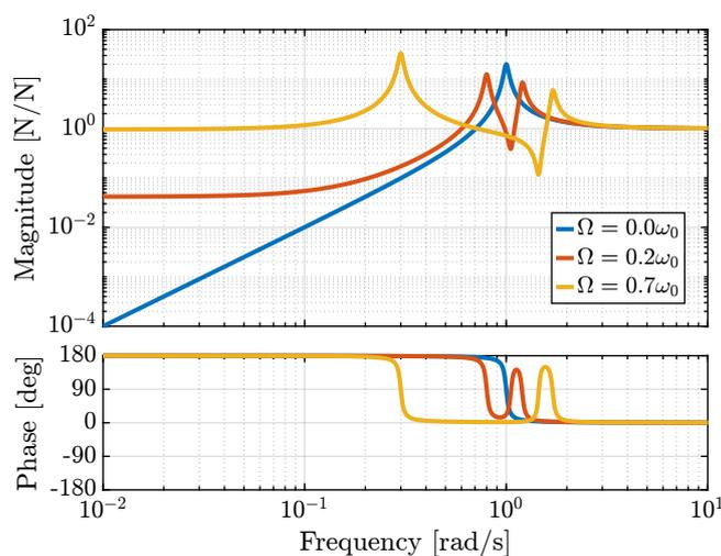
**Figure 2.3:** Comparison of the transfer functions from  $[F_u, F_v]$  to  $[f_u, f_v]$  for several rotating speed
