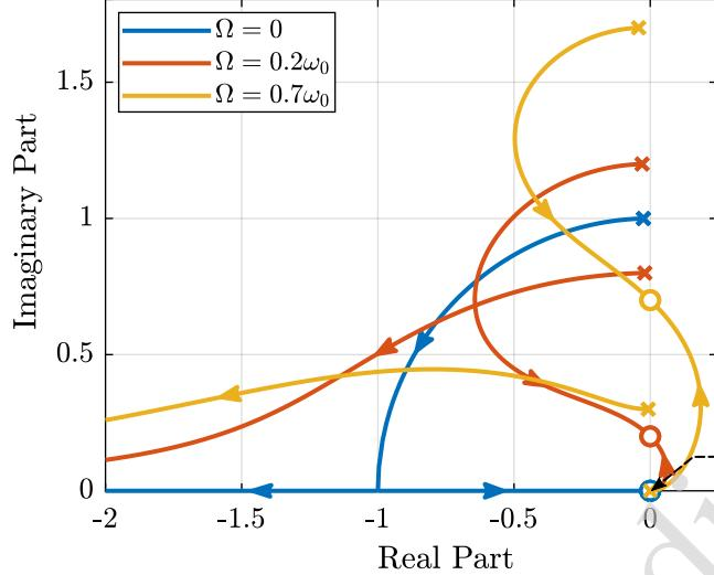
Figure 7: Root Locus: evolution of the closed-loop poles with increasing controller gains  $g$
