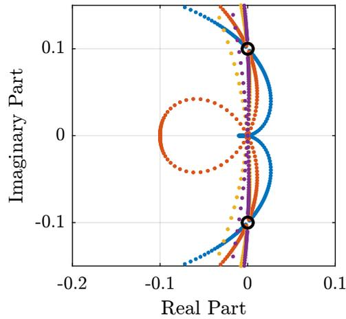
**Figure 3.5:** Root Locus for the modified IFF controller (zoomed plot on the left)
