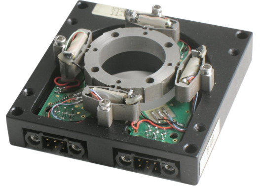
Figure 13: XY Piezoelectric Stage (XY25XS from Cedrat Technology)
