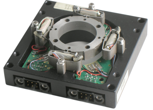
Figure 13: XY Piezoelectric Stage (XY25XS from Cedrat-Technology)
