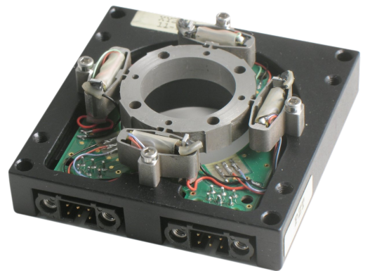
Figure 13: XY Piezoelectric Stage (XY25XS from Cedrat Technology)
